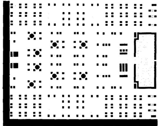
minimize offsets and thermal drift. The capacitor on the tile eliminates external compensation capacitors for op amps. This results in a savings of components, board space, and package pin count, and increases reliability. Ion implanted resistors have been included; these high resistor values in a small silicon area simplify low power designs. Dual layer metal greatly simplifies interconnection and power supply bussing.
