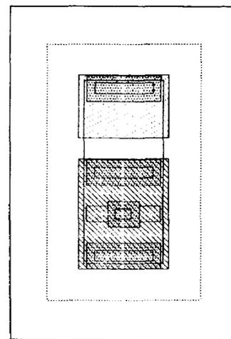
Low Noise, High Speed NPN Transistor
