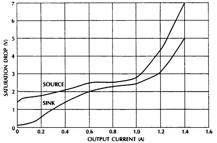
Figure 7. Output Saturation Voltage vs. Output Current
