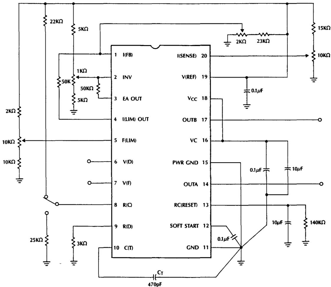
This test fixture is useful for exercising many of the ML4816's functions and measuring their specifications. As with any wideband circuit, careful grounding and bypass procedures should be followed. The use of a ground plane is highly recommended.
