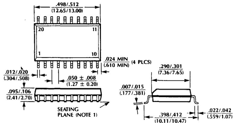
NOTE 1: SEATING PLANE LEAD COPLANARITY .005 (0.127) (BOTTOM OF LEADS).
