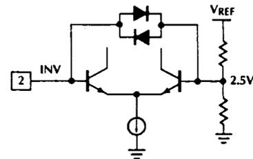
The Error Amplifier input contains protection diodes as shown above. INV should not be driven lower than  $2.5V - V_{BE}$  or higher than  $2.5V + V_{BE}$ .
