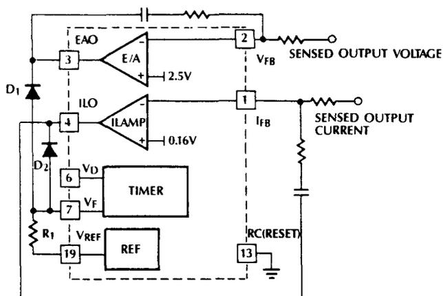
Figure 14. Auxiliary Output Current-Limiting
