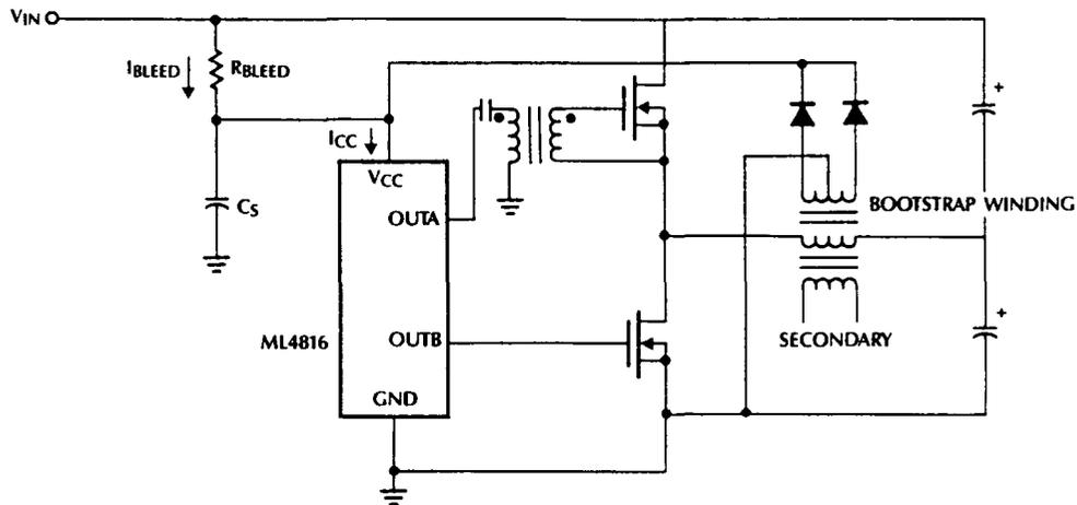
Figure 12. Simplified V<sub>CC</sub> Bootstrapping Scheme in Half-Bridge Configuration
