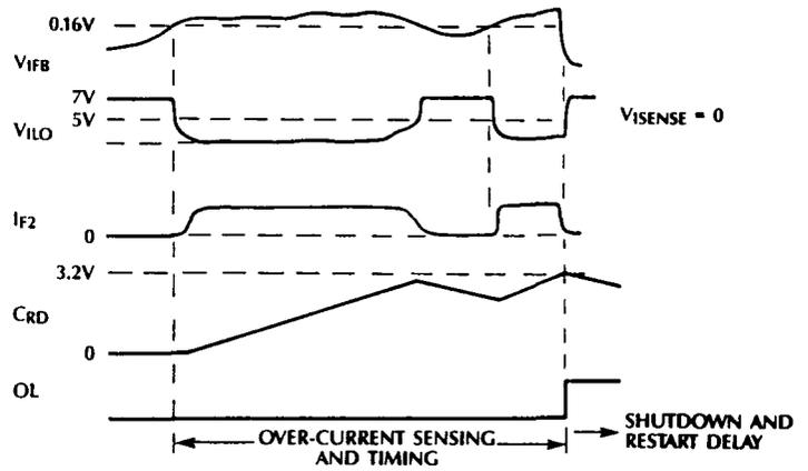
Figure 11. Secondary dc Current Sensing, Overload Shutdown and Restart Sequence (Non-Bootstrapped V<sub>CC</sub>)
