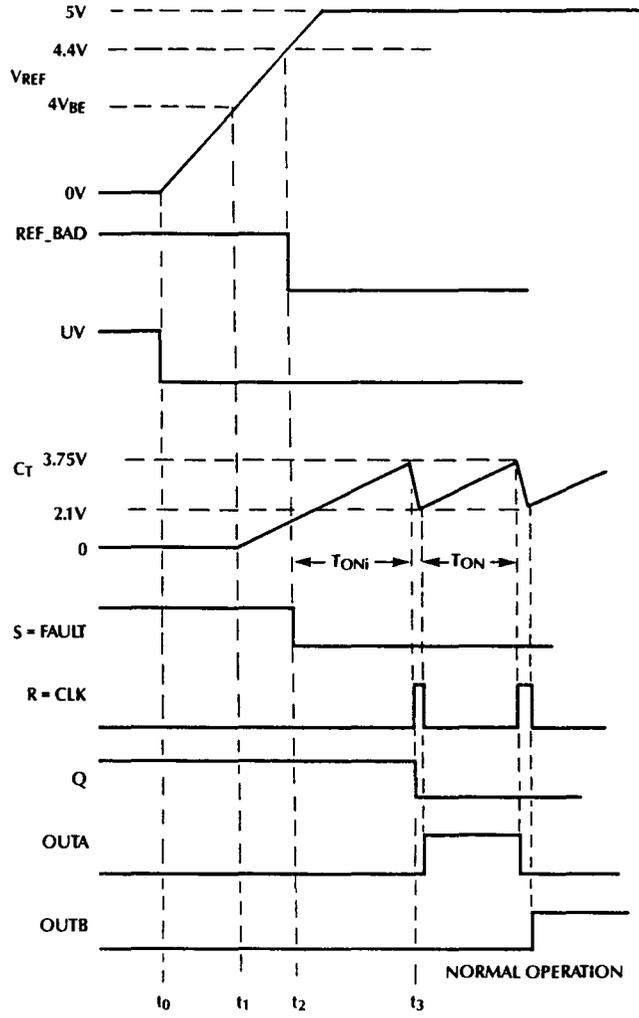
Figure 16. Timing Diagram Illustrating Initial Start-Up and the First-Pulse Inhibit
