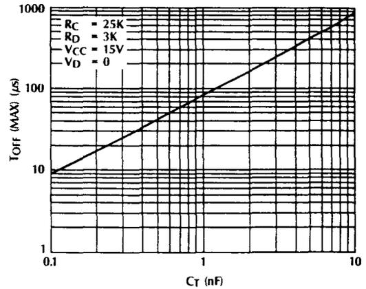
Figure 2a. Max ( $T_{OFF}$ ) vs.  $C_T$
