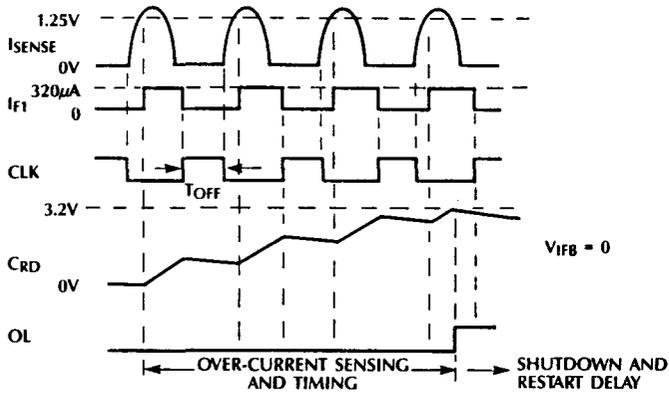
Figure 10. Over-Current Sensing, Overload Shutdown and Restart Sequence (Non-Bootstrapped V<sub>CC</sub>) (ZCS-QRC Transistor Current Shown)
