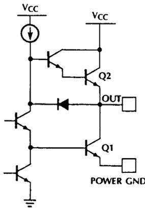
Figure 6. Power Driver Simplified Schematic
