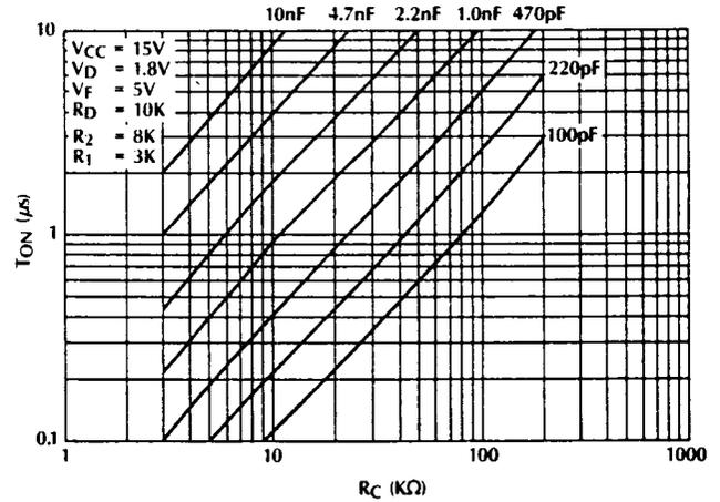
Figure 3a. Minimum  $T_{ON}$  for Constant Off-Time
