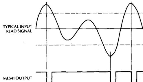
Pin R/WB must be high for the output logic to be active. The key element in the output logic is the D flip-flop. The flip-flop is clocked by the slope detector at the time of a zero crossing, which loads data from level detector. The flip-flop inputs only change state when the level detector detects a peak amplitude of a polarity opposite to the previous valid peak. Thus, through the output logic the slope detector determines output timing and the level detector determines pulse validity.
