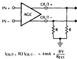
$$I_{OUT+} \text{ TO } I_{OUT-} = 4\text{mA} + \frac{8\text{V}}{R_{EXT}}$$
