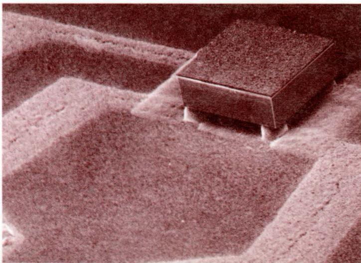
*Perhaps the most significant advancement in reducing the price and increasing the reliability of the SD line is the development of an advanced mounting technique that places the chip face down on the ceramic and gives the new technology its name—“flip chip.” With this process, the proven reflow solder method replaces the laborious hand operation of ultrasonically bonding the microscopic wires from the chip to the lead frame.*
