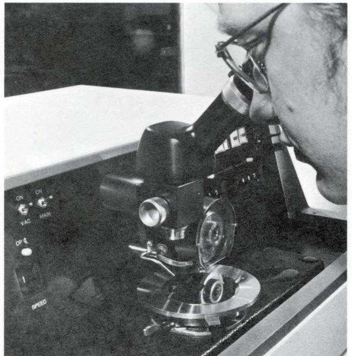
Silicon wafer separation by ultrahigh-speed saw insures the straight sides needed for the continued automated handling of the microscopic chips.
