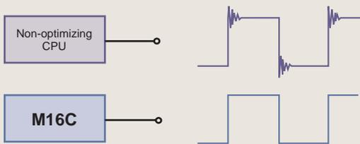
Even when using an external bus, EMI noise is kept to a minimum.
