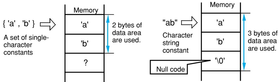
Figure 1.2.2 Difference between {'a', 'b'} and "ab"
