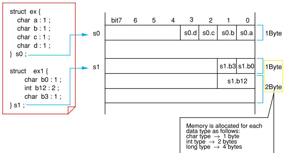
Figure 2.3.6 Example of memory allocation for bit fields
