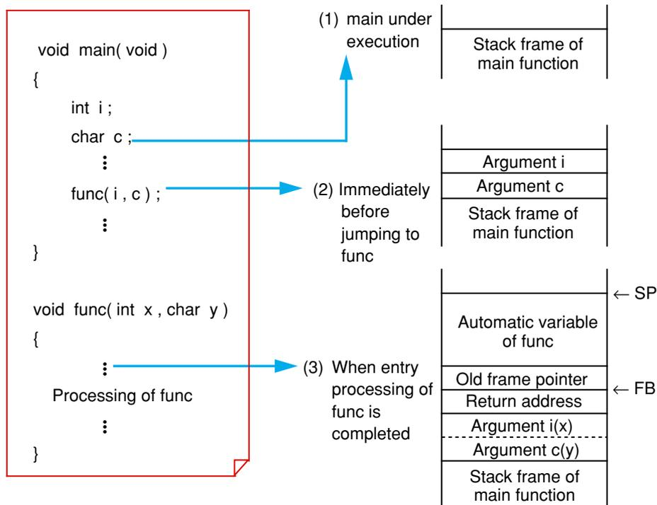
**Figure 2.4.3 Constructing a stack frame**
