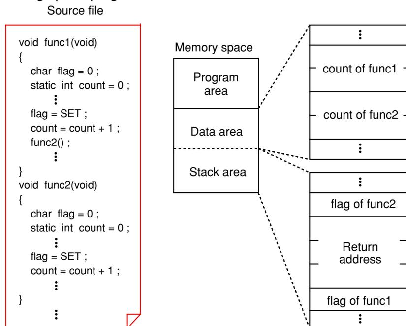
Figure 1.6.4 Storage classes of internal variable
