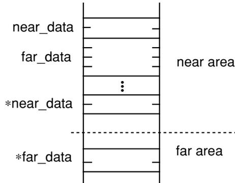
**Figure 2.3.3 Specifying address size stored in pointer**
