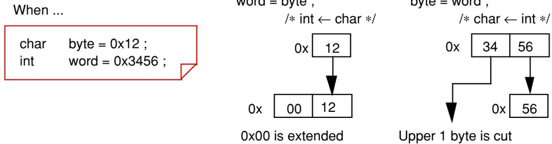
**Figure 1.3.1 Assign different types of data**
