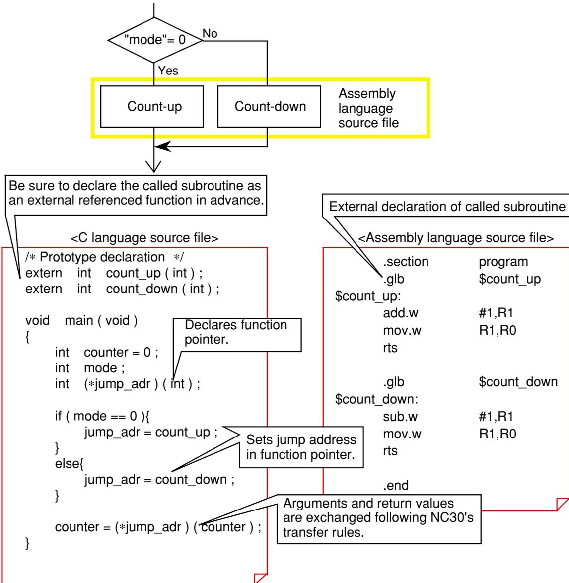
Figure 2.4.9 Calling a subroutine by indirect addressing
