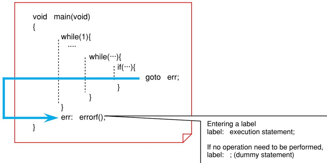
**Figure 1.4.10** Example of “goto” processing
