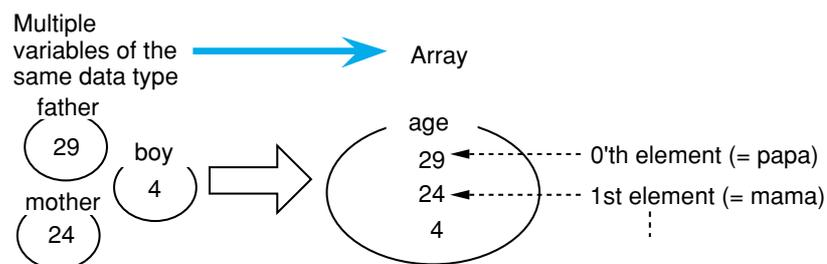
Figure 1.7.1 Concept of an array
