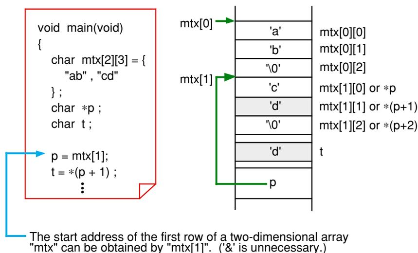
Figure 1.7.7 Pointer variables and two-dimensional array
