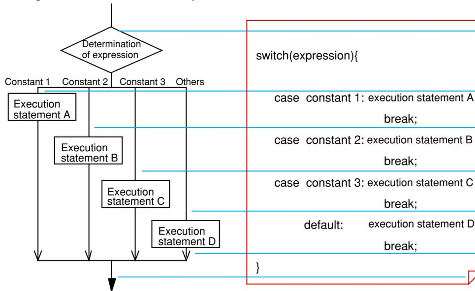
**Figure 1.4.3 Example of “switch-case” processing**
