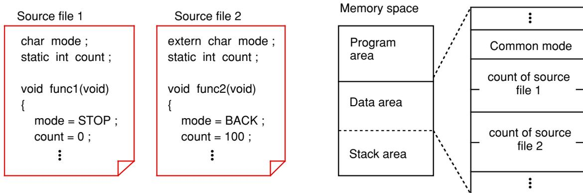
Figure 1.6.3 Storage classes of external variable
