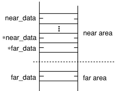
**Figure 2.3.4 Specifying area to locate the pointer**
