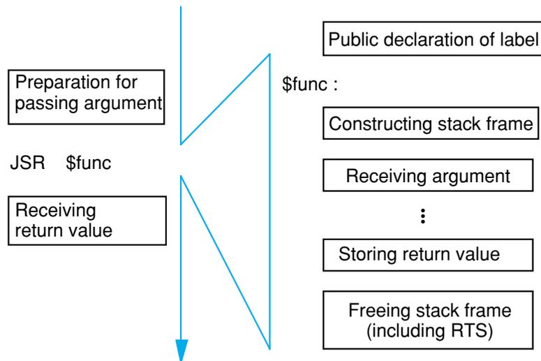
Figure 2.4.1 Operations for calling a function
