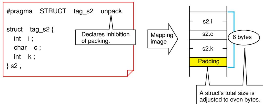
Figure 2.1.8 Inhibiting struct members from being packed
