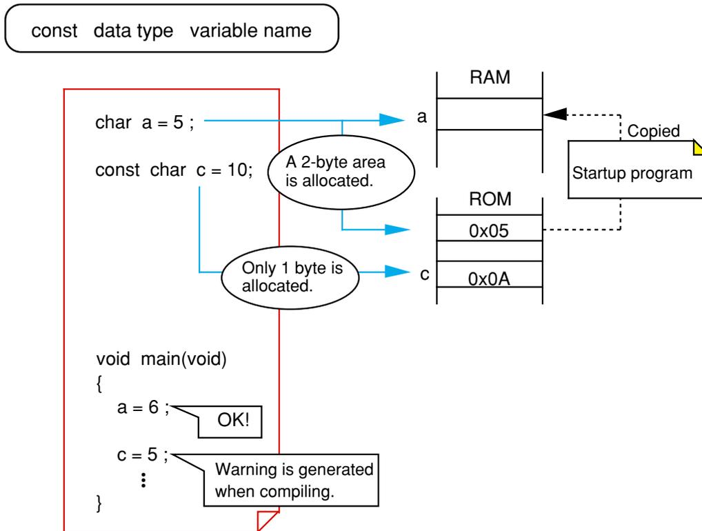
**Figure 2.1.6 const modifier and memory mapping**
