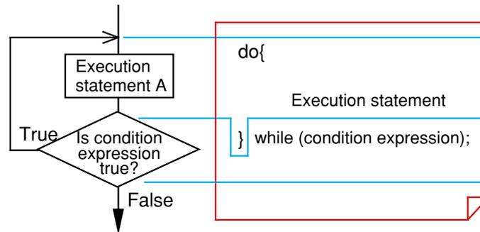
**Figure 1.4.7 Example of “do-while” processing**
