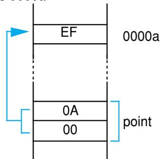
Figure 2.3.8 Specifying absolute addresses using a pointer
