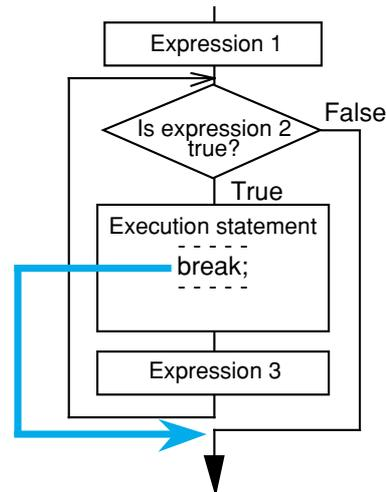
Figure 1.4.8 Example of "break" processing
