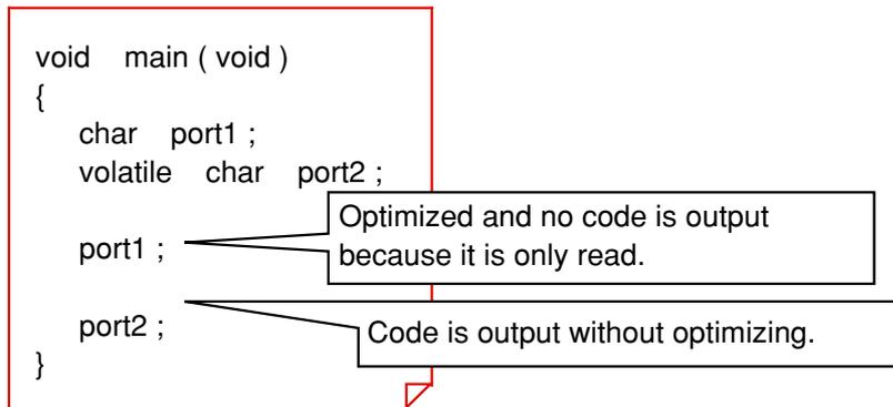
**Figure 1.2.6 Example for writing the type qualifier "volatile"**
