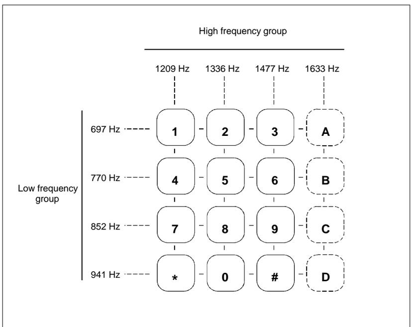
**Figure 1: The allocation of frequencies in the framework of the 4x4 matrix on the telephone keypad**
