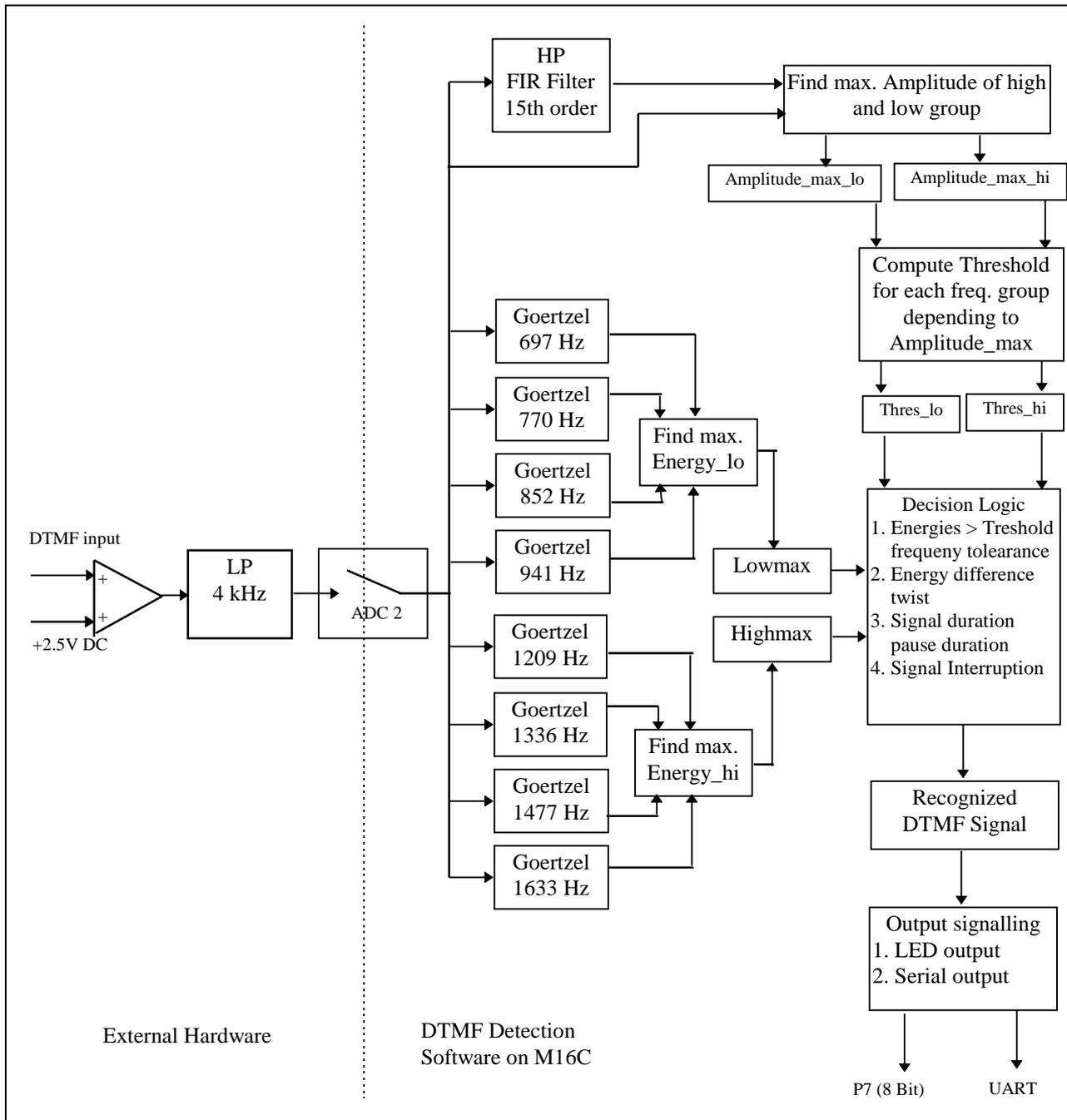
**Figure 3: Software concept and hardware interface connection**
