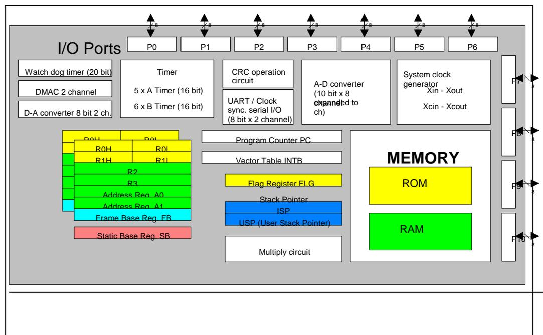
**Figure 2: The M16C/62 handles 8 VAX-MIPS at a clock frequency of 16MHz. The minimum instruction execution time is 62.5 ns.**
