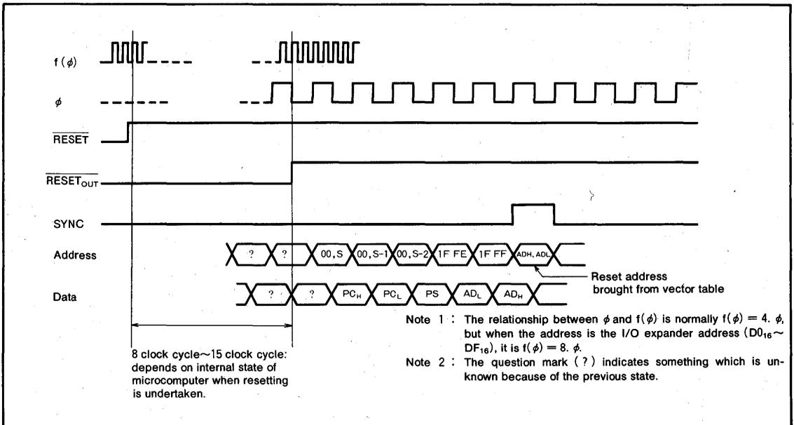
Fig.6 Timing diagram during resetting
