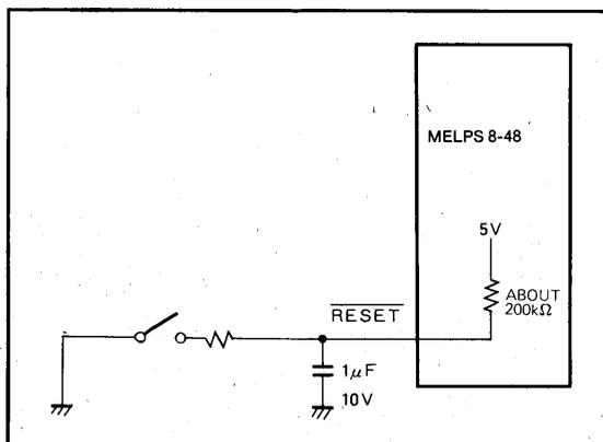
Fig. 13 Example of a reset circuit
