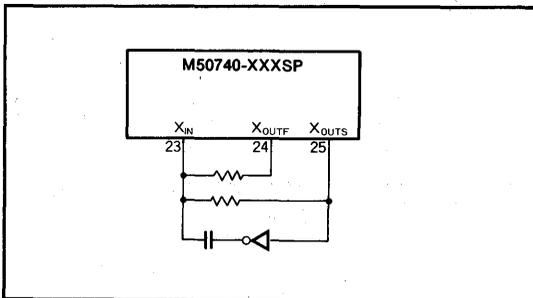
Fig.14 External RC circuit
