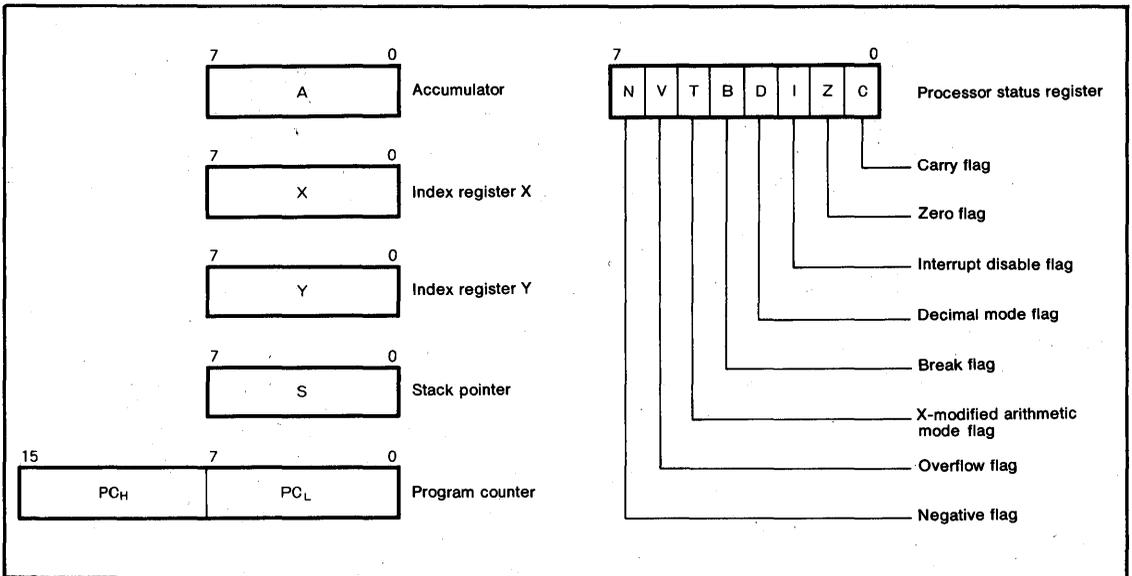
Fig.2 Register configuration
