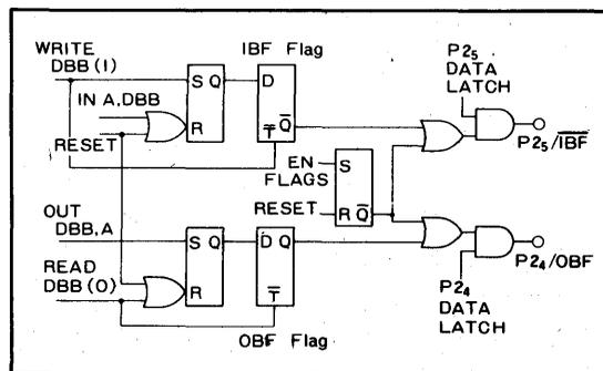
Fig.19 Internal configuration of IBF/OBF
