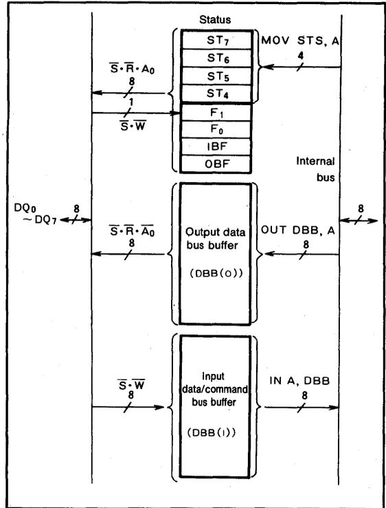
**Fig.7 Internal configuration of data bus**
