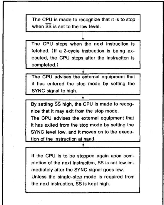
Fig.15 CPU operation in single-step mode
