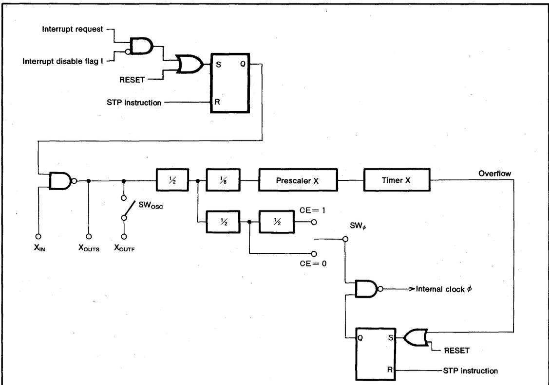
Fig.11 Block diagram of clock generator circuit
