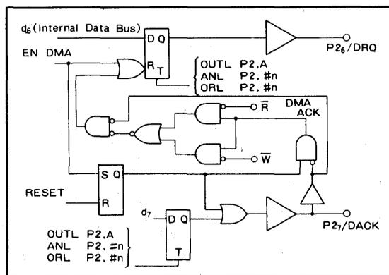
Fig.17 Internal configuration of DMA control
