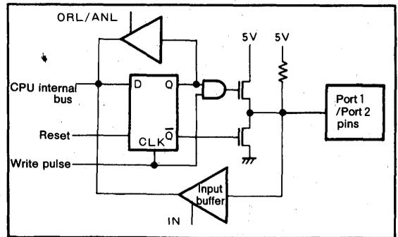
Fig.5 I/O port 1 and 2 circuit
