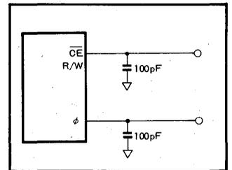
Fig.18  $\overline{CE}$ , R/W test circuit
