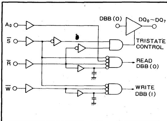
**Fig.6 Internal configuration of data bus control**
