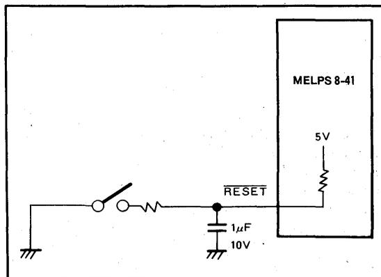
Fig.13 Example of reset circuit
