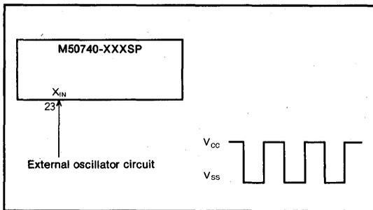
Fig.13 External clock input circuit
