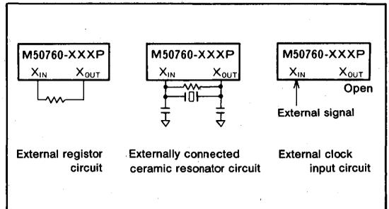
Fig.5 Clock generator circuits
