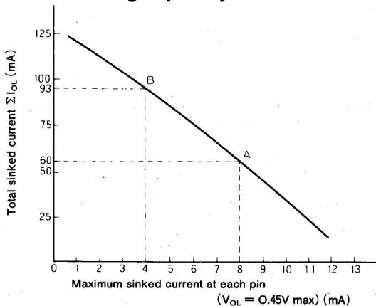
Each of the 16 I/O lines of the M5L8243P is capable of sinking 5mA simultaneously ( $V_{OL} = 0.45V\ max$ ). However, the drive capacity of each line depends upon whether all lines are sinking current simultaneously and on the degree of loading. This is illustrated in the curve shown.
