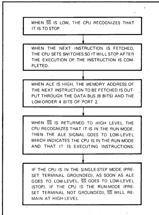
Fig. 15 CPU operation in single-step mode
