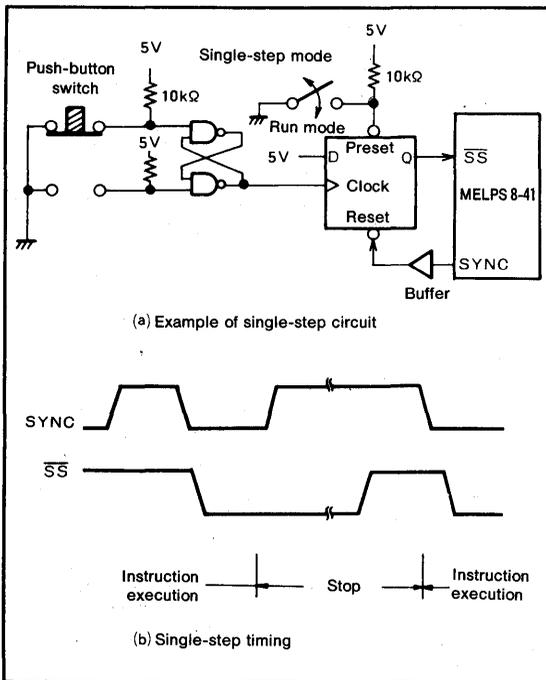
Fig.14 Single-step operation circuit and timing
