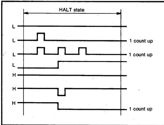
**Fig. 1 Counter operation in the HALT mode**
