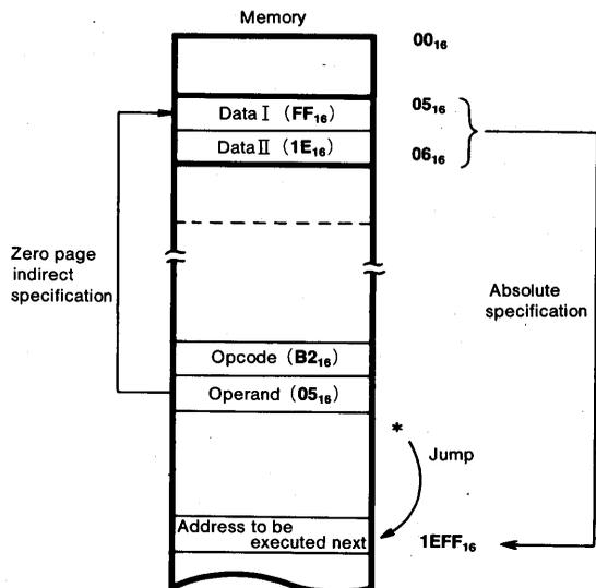
In this example, FF<sub>16</sub> as data I and 1E<sub>16</sub> as data II have been stored beforehand.
