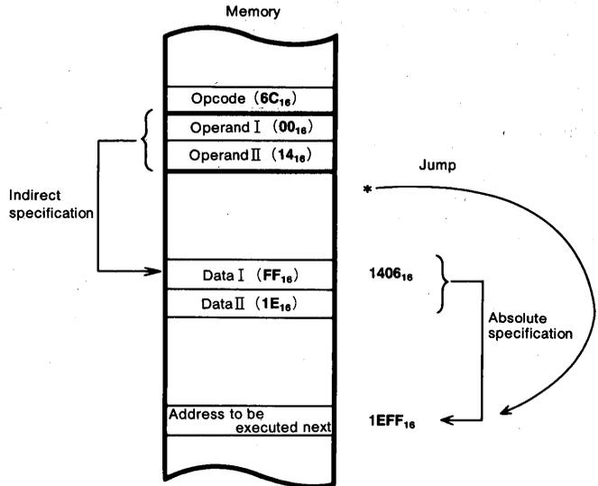
In this example, FF<sub>16</sub> as data I and 1E<sub>16</sub> as data II have been stored beforehand.
