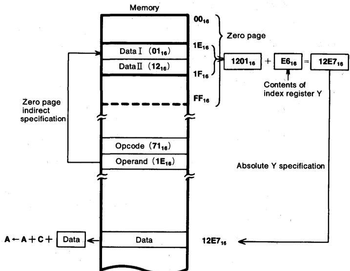
In this example, 00<sub>16</sub> as data I and 12<sub>16</sub> as Data II have been stored beforehand.
