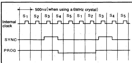
Fig.11 Clock and generated cycle signals
