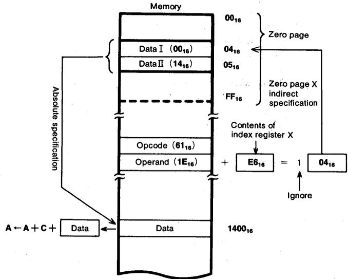
In this example, 00<sub>16</sub> as data I and 14<sub>16</sub> as data II have been stored beforehand.
