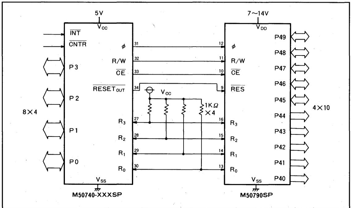
Fig.1 Example of connections between I/O expander (M50790SP) and microcomputer (M50740-XXXSP)
