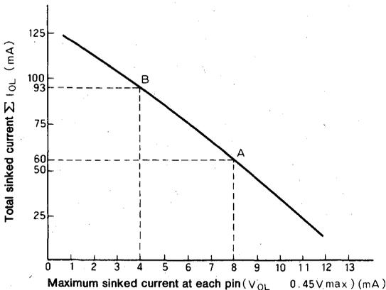
Each of the 16 I/O lines of the M5M82C43P is capable of sinking 5mA simultaneously ( $V_{OL} = 0.45V_{max}$ ). However, the drive capacity of each line depends upon whether all lines are sinking current simultaneously and on the degree of loading. This is illustrated in the curve shown.
