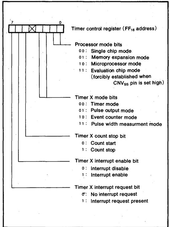
Fig.5 Configuration of timer control register
