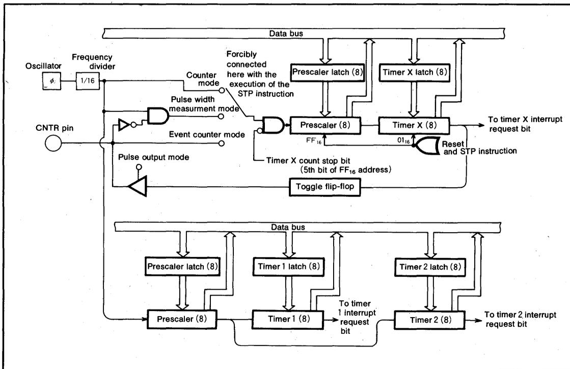
Fig.4 Block diagram of timer X, timer 1, timer 2
