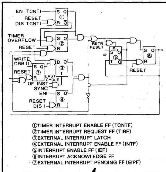
Fig.8 Interrupt control section configuration
