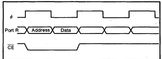
Fig.10 Timing diagram of port R
