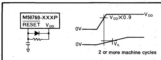
Fig.4 Power-on resetting circuit
