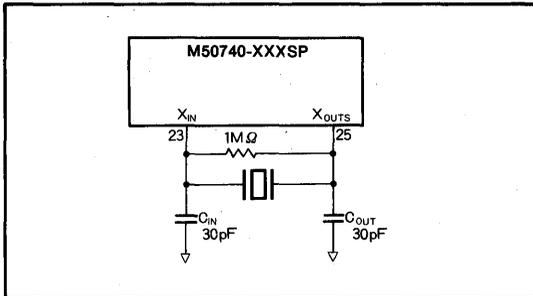
Fig.12 Externally connected ceramic resonator circuit
