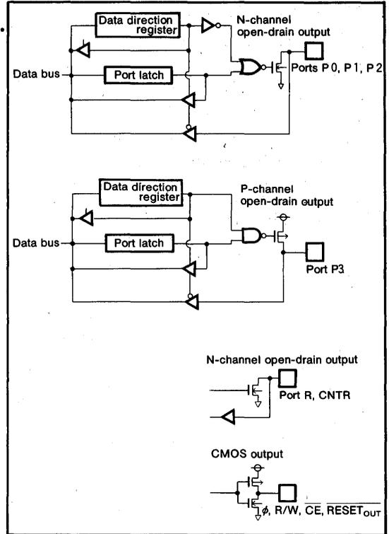
Fig.9 Block diagram of port P0~P3 (single chip mode) and output formats of port R, CNTR, R/W,  $\overline{CE}$  and  $\overline{RESET}_{OUT}$
