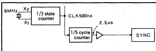
Fig.10 Clock generator circuit
