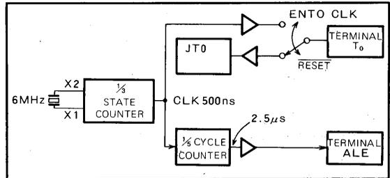
Fig.10 Clocking cycle generation
