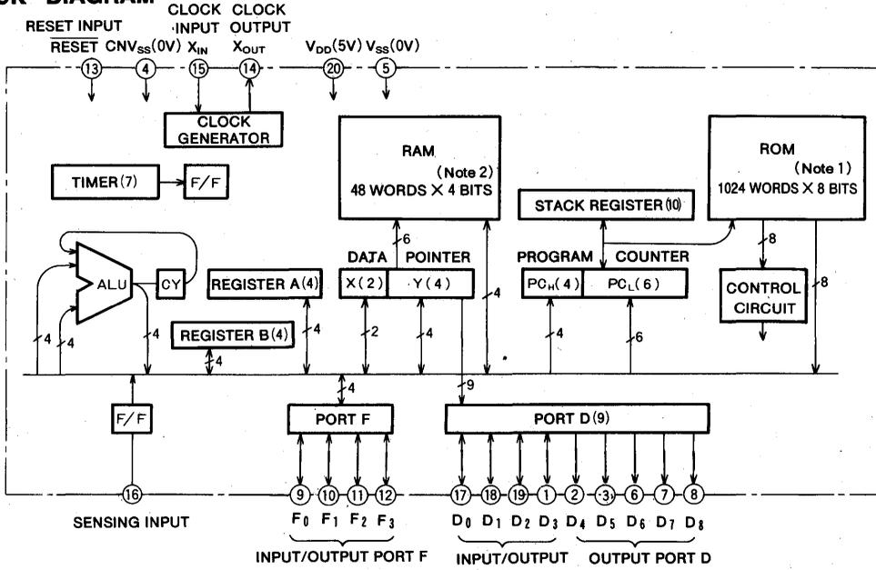
Note 1 : The M50761-XXXP has a ROM capacity of 512 words  $\times$  8 bits.
