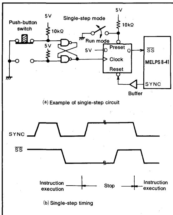
Fig.14 Single-step operation circuit and timing
