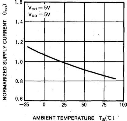
**NORMARIZED SUPPLY CURRENT ( $I_{DD}$ )
