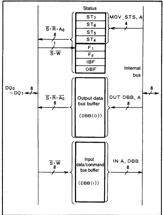
**Fig.7 Internal configuration of data bus**
