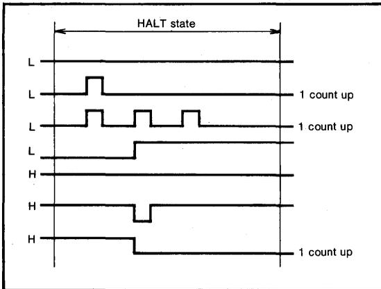
**Fig. 1 Counter operation in the HALT mode**
