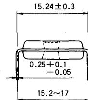
**TYPE 40P4B 40-PIN MOLDED PLASTIC DIL (LEAD PITCH 1.78mm)**
