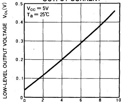
LOW-LEVEL OUTPUT CURRENT  $I_{OL}$ (mA)
