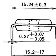
TYPE 52P4B 52-PIN MOLDED PLASTIC DIL (LEAD PITCH 1.78mm)
