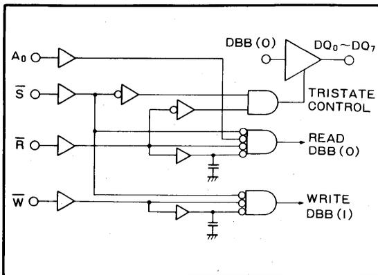
**Fig.6 Internal configuration of data bus control**
