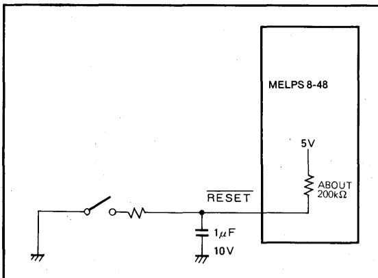
Fig. 13 Example of a reset circuit
