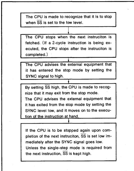
Fig.15 CPU operation in single-step mode
