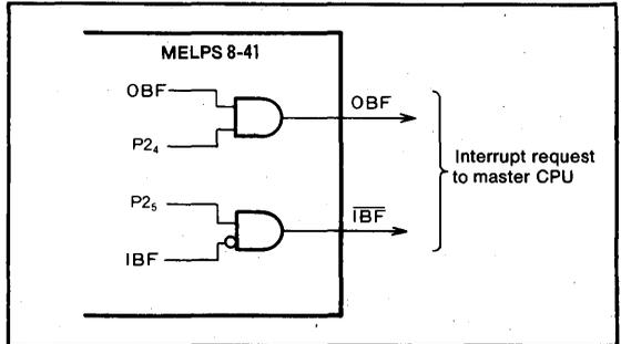
Fig.18 Interrupt request to master CPU
