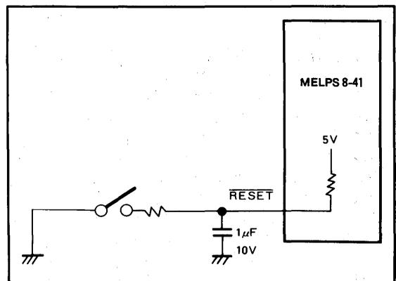
Fig.13 Example of reset circuit
