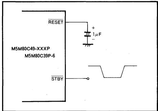
**Fig. 2 Control circuit example for standby mode**
