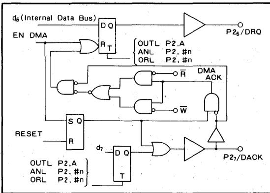
Fig.17 Internal configuration of DMA control
