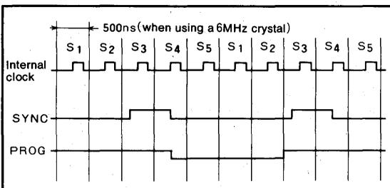
Fig.11 Clock and generated cycle signals
