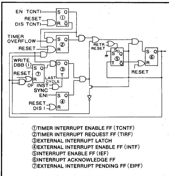
Fig.8 Interrupt control section configuration
