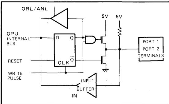
**Fig. 8 I/O ports 1 and 2 circuit**
