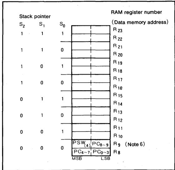
Fig.3 Relationship between program counter stack and stack pointer
