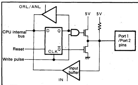
Fig.5 I/O port 1 and 2 circuit
