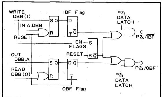
Fig.19 Internal configuration of IBF/OBF
