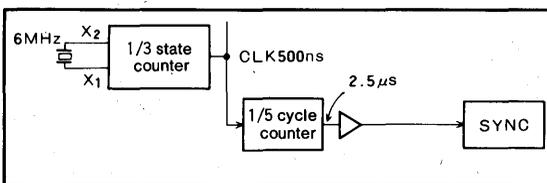
Fig.10 Clock generator circuit
