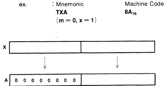
(Note) When the data length differ between the transfer-from and transfer-to locations, data is transferred at the data length for the transfer-to location. If, however, the index register is specified as the transfer-to location and the x flag is set to 1, 0016 is sent as the upper byte value.
