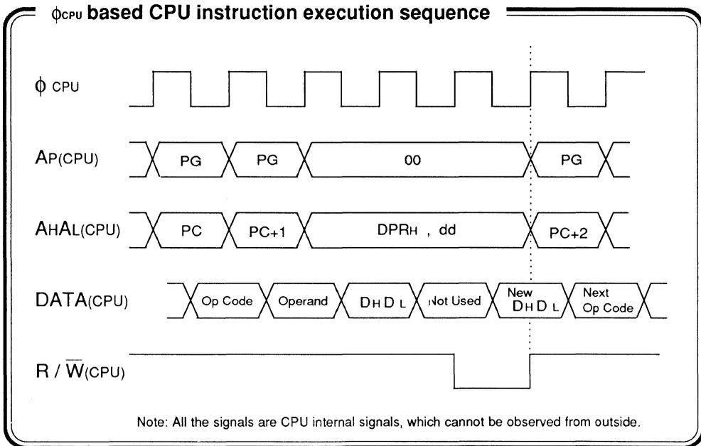
The following examples 1-1 to 1-6 are examples of the  $\phi_{CPU}$  based instruction execution sequences under various conditions.
