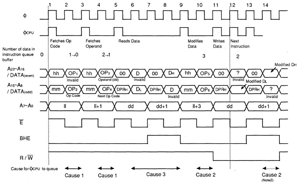
Note1. The operation when internal ROM and internal RAM are used, will be as shown above, regardless of the level of the BYTE terminal. However, the address/data bus, BHE, R/W signal cannot be observed from outside, when the mode is single chip mode.
