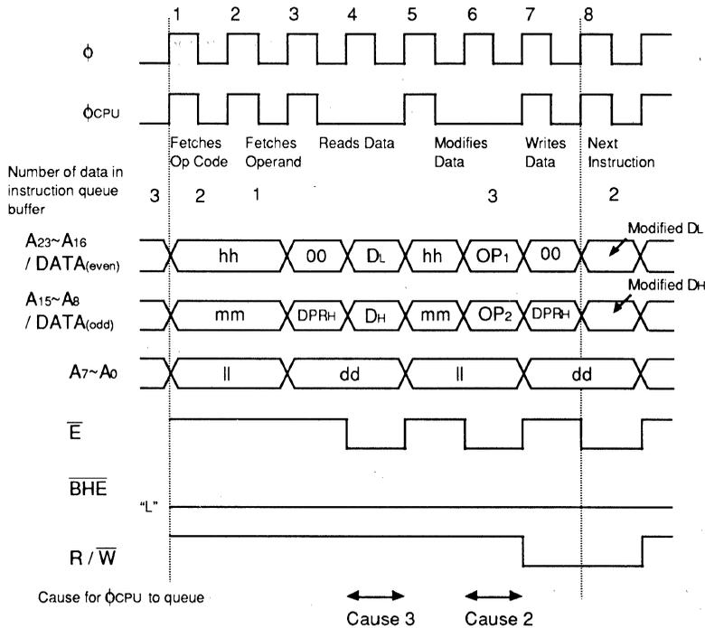
Note. The operation when internal ROM and internal RAM are used, will be as shown above, regardless of the level of the BYTE terminal. However, the address/data bus,  $\bar{BHE}$ , R/W signal cannot be observed from outside, when the mode is single chip mode.
