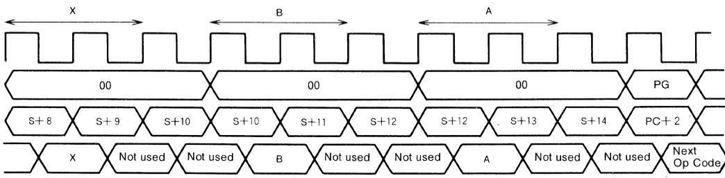
(Note) This figure is an example pulled all the registers by PUL instruction. If some register is not pulled, its cycle (→) is nothing.
