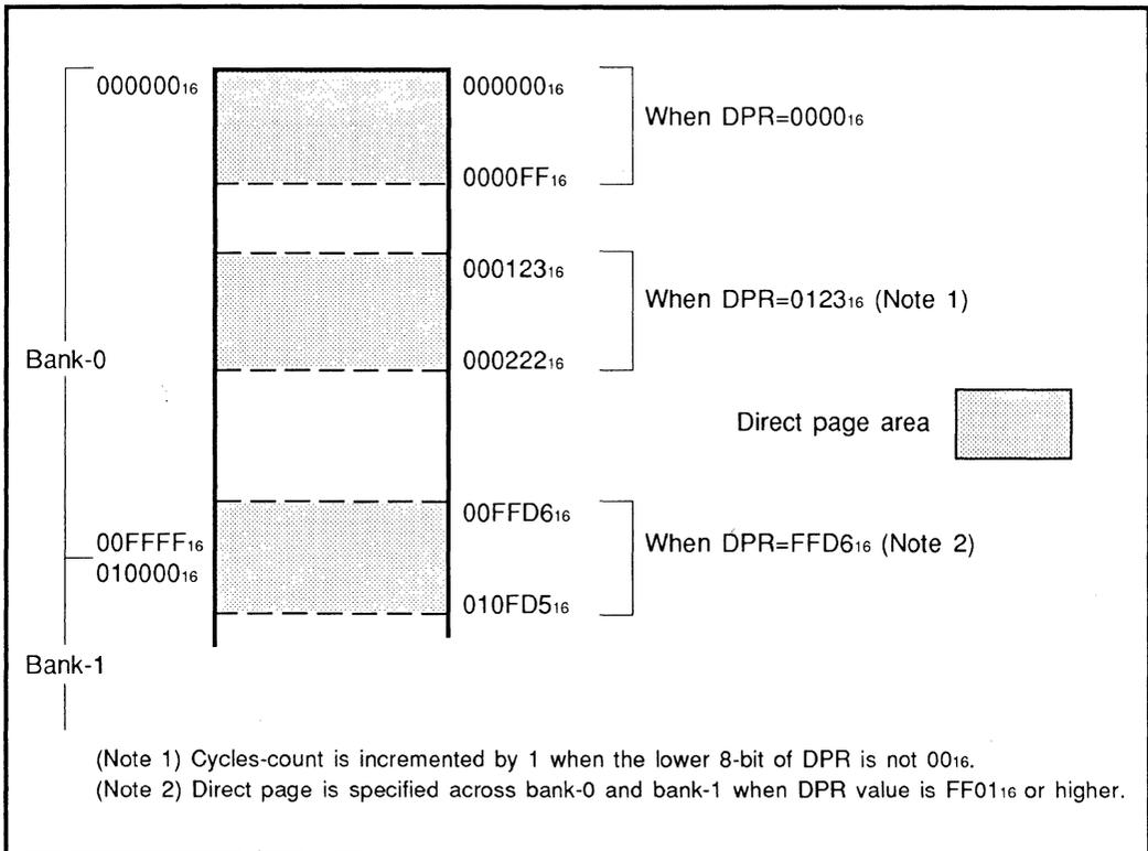
Fig. 2.2 Setting Direct Page by Direct Page Register
