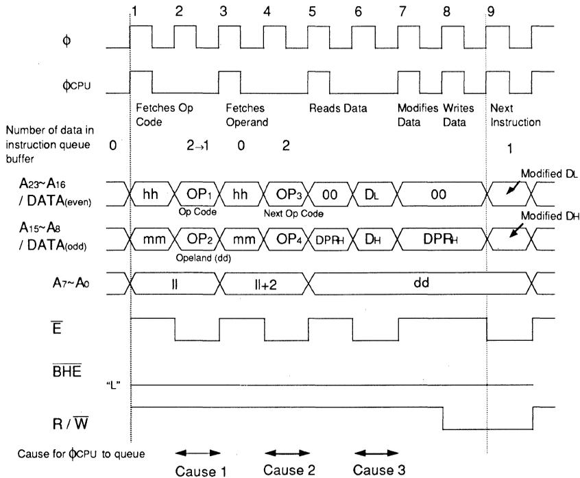
Note. The operation when internal ROM and internal RAM are used, will be as shown above, regardless of the level of the BYTE terminal. However, the address/data bus,  $\overline{BHE}$ , R/ $\overline{W}$  signal cannot be observed from outside, when the mode is single-chip mode.
