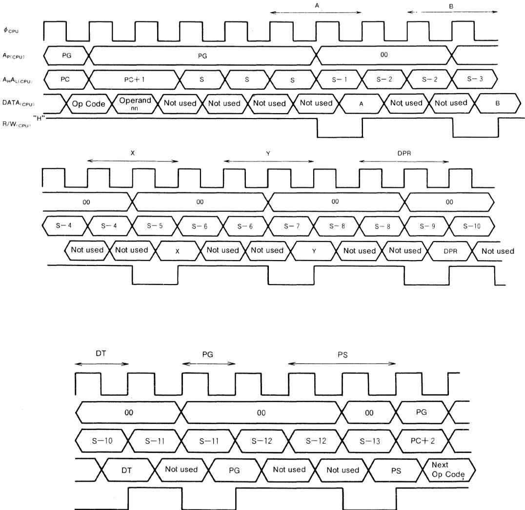
(Note) This figure is an example pushed all the registers by PSH instruction. If any register is not pushed, its cycle ( $\leftrightarrow$ ) is nothing.
