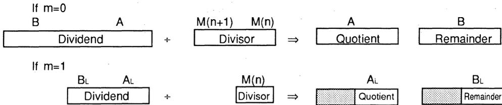
**Description** : When the data length selection flag m is set to 0, a 32-bit data stored in the accumulators B (upper 16 bits) and A (lower 16 bits) are divided by a 16-bit data in memory. The quotient is placed in the accumulator A, and the remainder is placed in the accumulator B.
