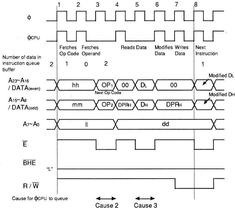
Note. The operation when internal ROM and internal RAM are used, will be as shown above, regardless of the level of the BYTE terminal. However, the address/data bus, BHE, R/W signal cannot be observed from outside, when the mode is single chip mode.
