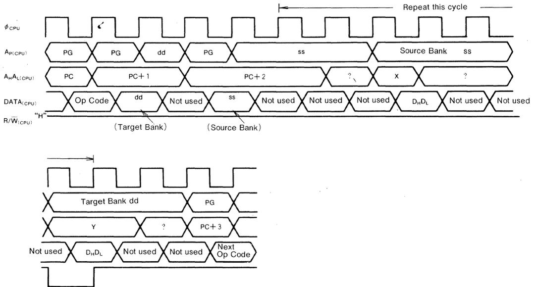
(Note) This figure is shown that transferred the 2-bytes data started from even address. If transferred more than 3-bytes data, the cycle (↔) is repeated each 2-bytes.
