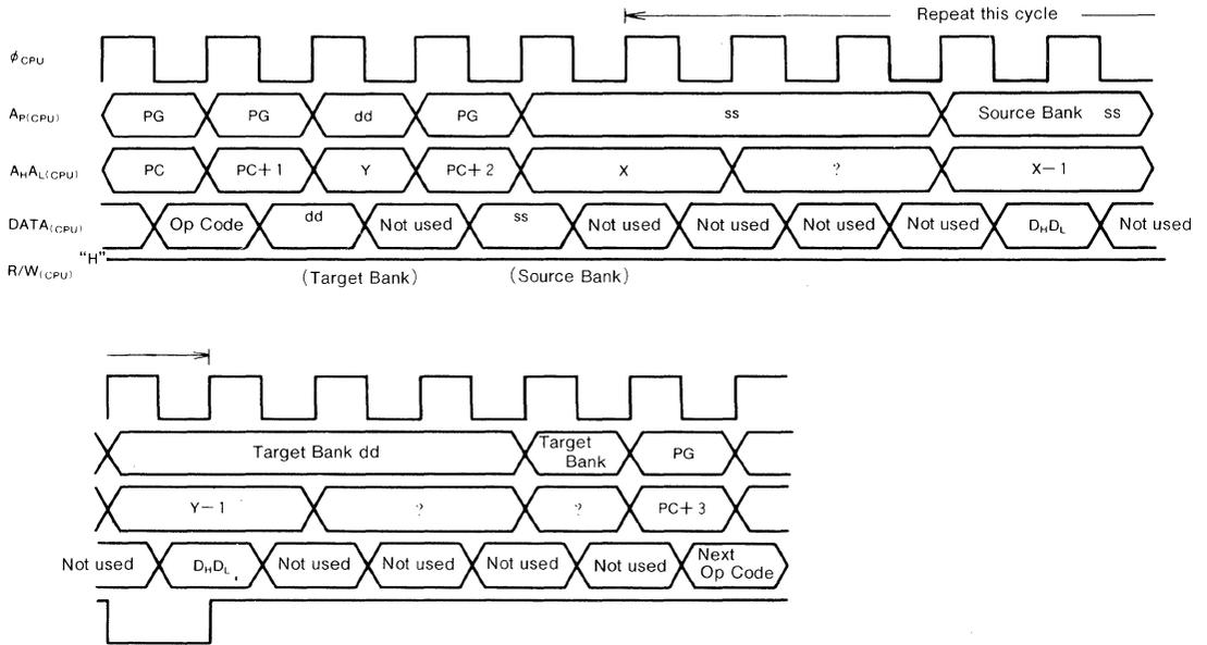
(Note) This figure is shown that transferred the 2-bytes data started from even address. If transferred more than 3-bytes data, the cycle(↔) is repeated each 2-bytes.
