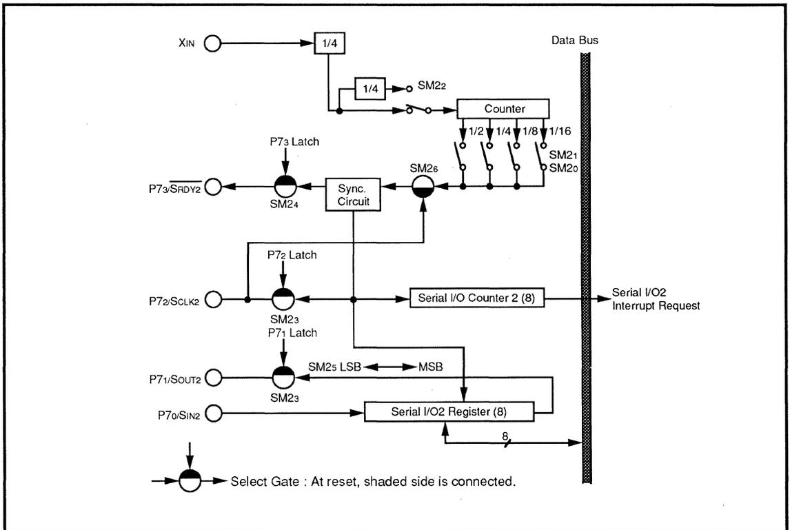
Fig. 2.8.1 Block Diagram of Clock Synchronous Serial I/O2 Function
