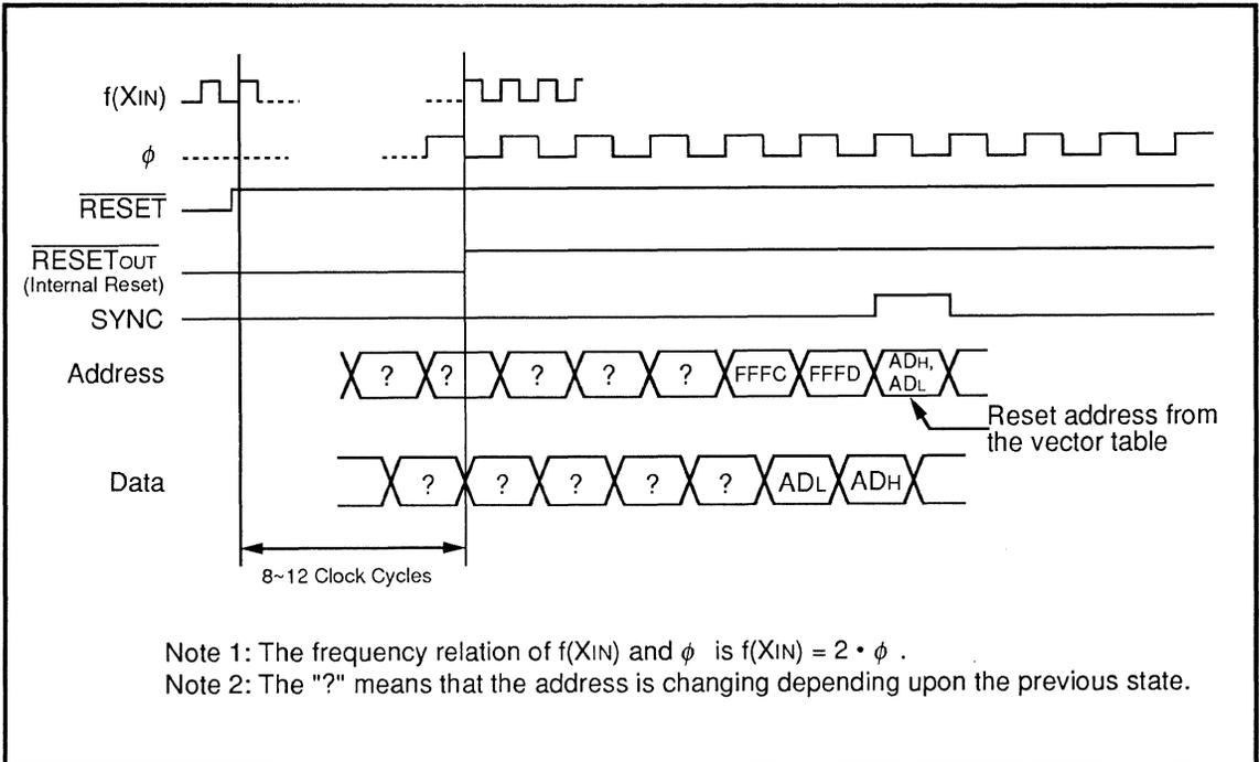
Fig. 2.11.1 Internal Processing Sequence after Reset
