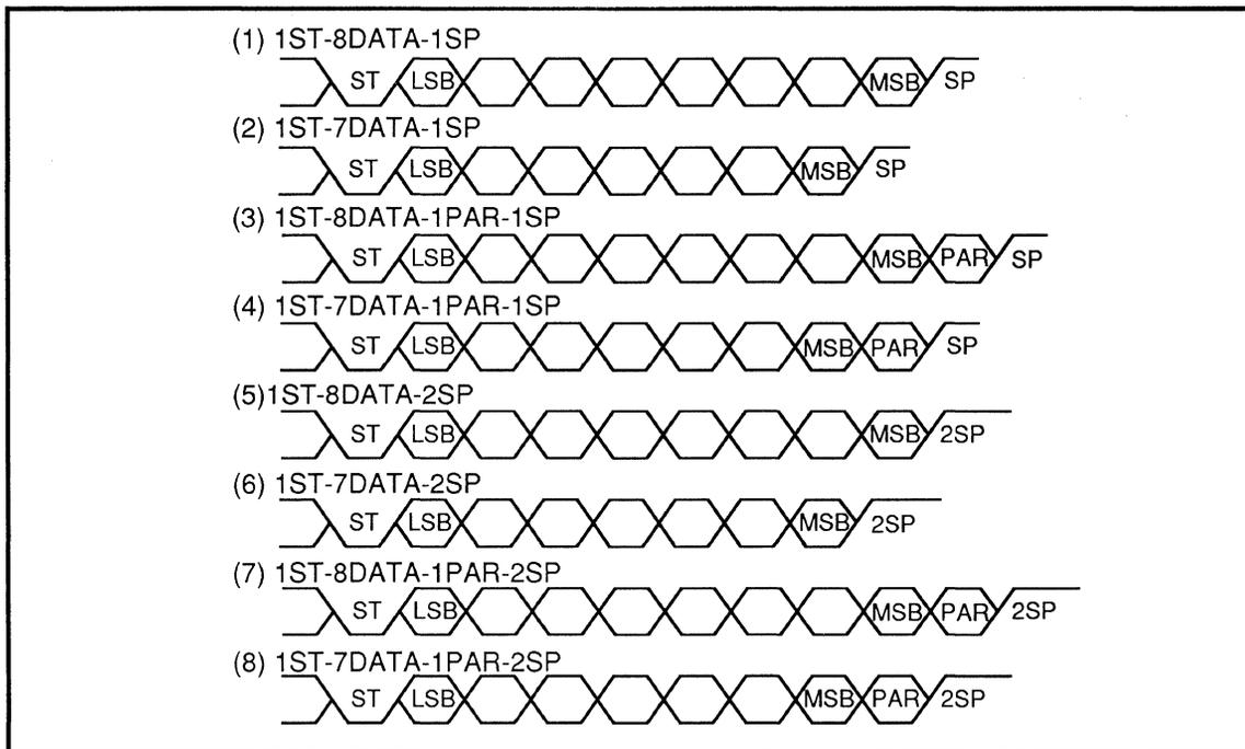
Fig. 2.7.10 Serial Data Transfer Format
