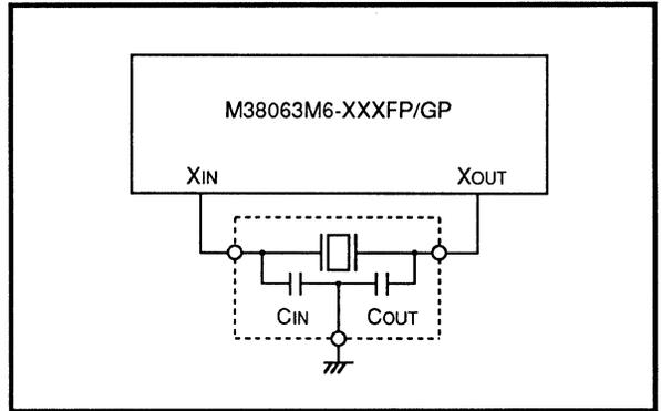
Fig. 2.12.3 Example of Oscillation Circuit with Internal Capacitors
