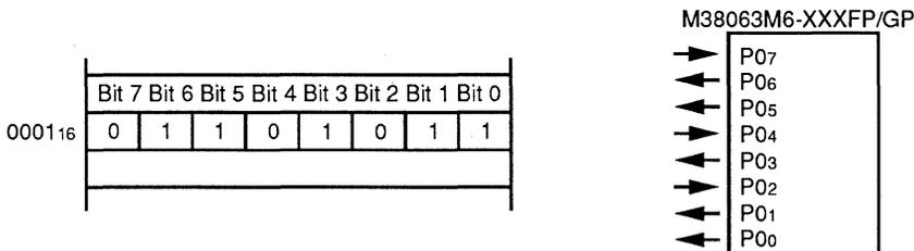
Note that the direction registers should not be read. Do not use the set bit or clear bit commands on the direction registers, and do not try to use the direction registers for logical operations, arithmetic operations, condition judgements, or address calculations.
