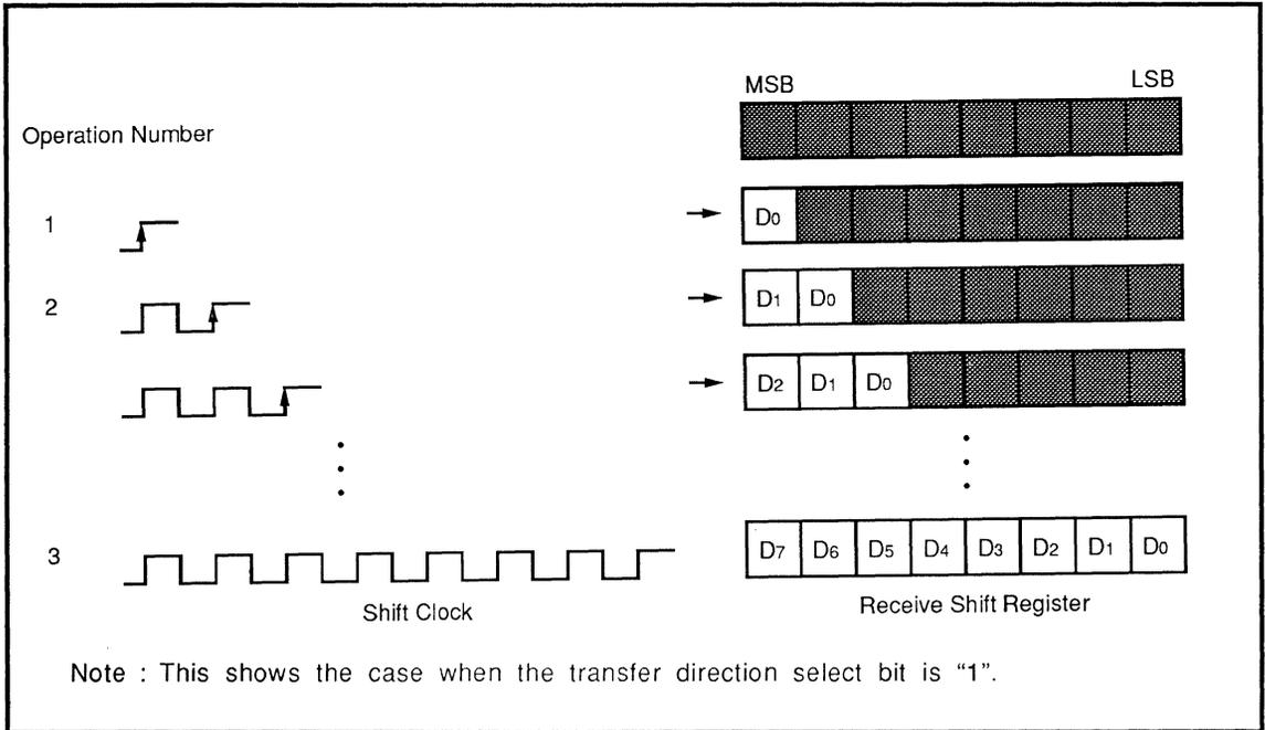
Fig. 2.8.2 Serial I/O2 Reception Operation
