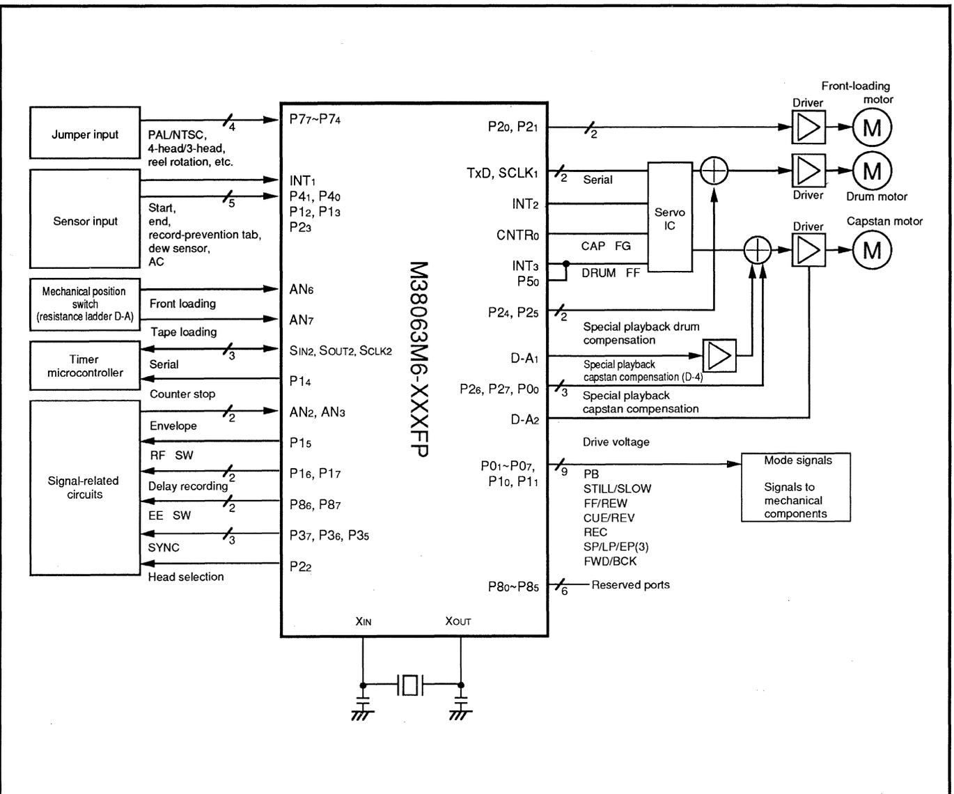
Fig. 4.1.2 Example of VCR System Controller System
