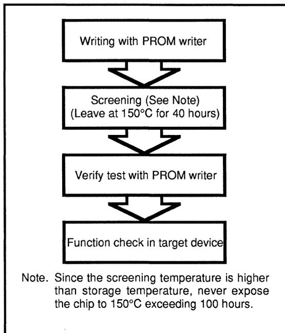
Fig. 3.4.1 Flow of Writing and Testing of One-Time Programmable Versions
