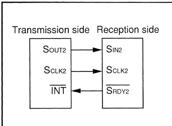
Fig. 2.8.5 Connection for Serial I/O2 Function
