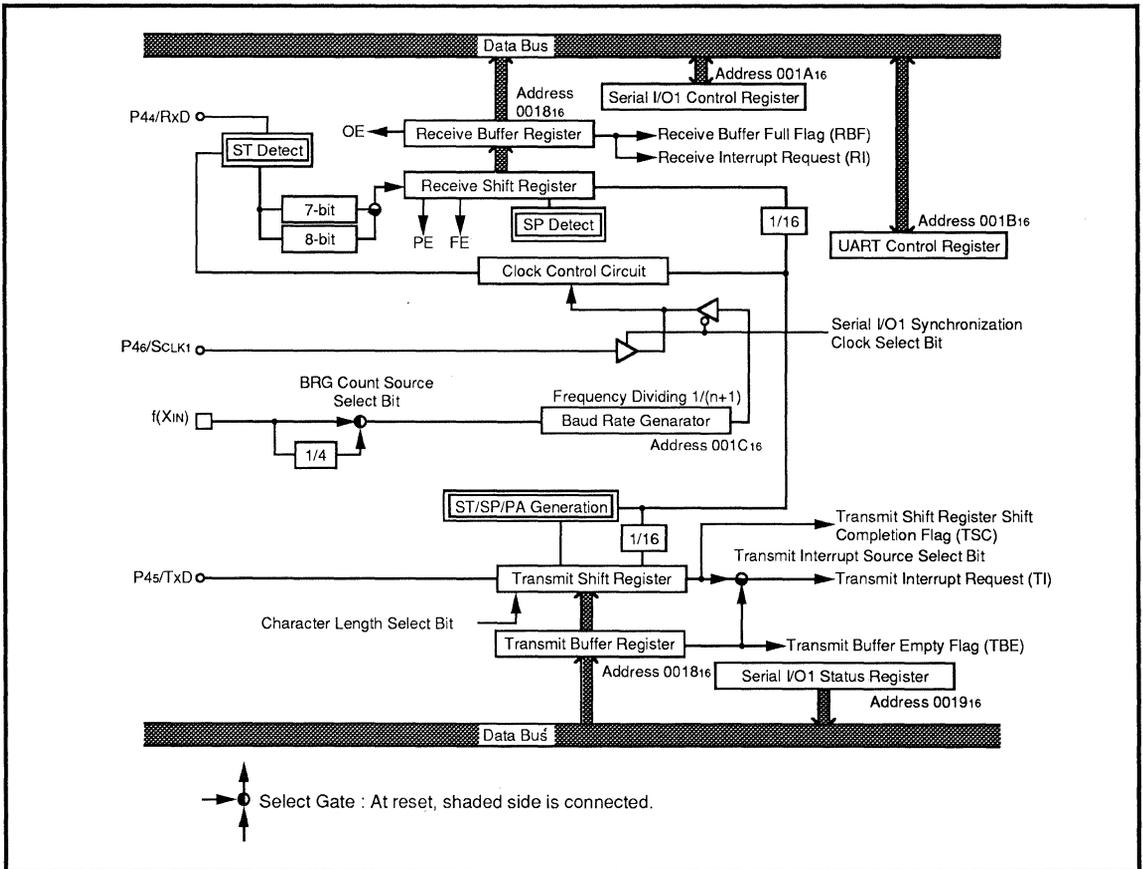
Fig. 2.7.8 Block Diagram of Clock Asynchronous Serial I/O Function
