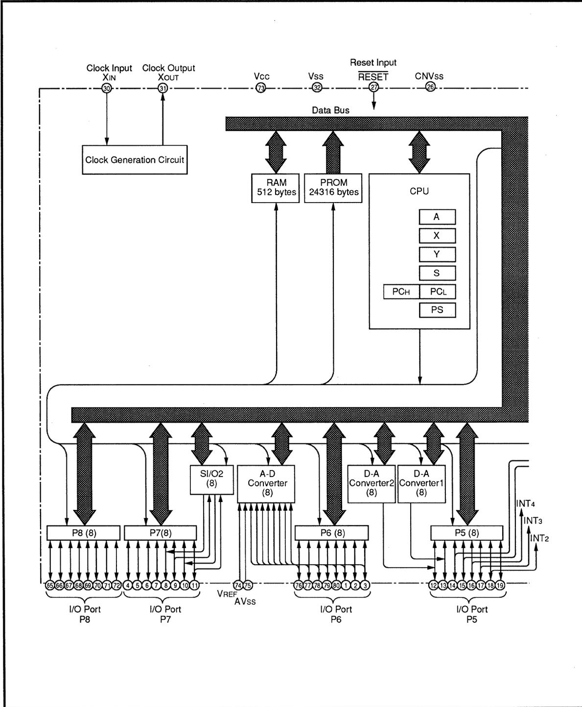
Fig. 3.3.1 Functional Block Diagram of Internal PROM Version
