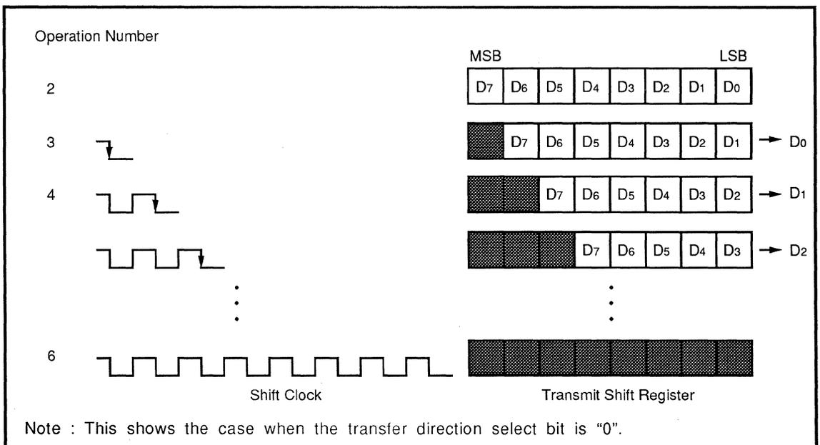
Note : This shows the case when the transfer direction select bit is "0".
