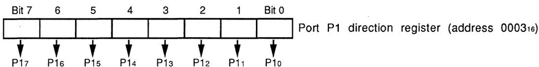
When "0" is written to the bit corresponding to a pin, that pin becomes an input pin; when "1" is written to that bit, that pin becomes an output pin.
