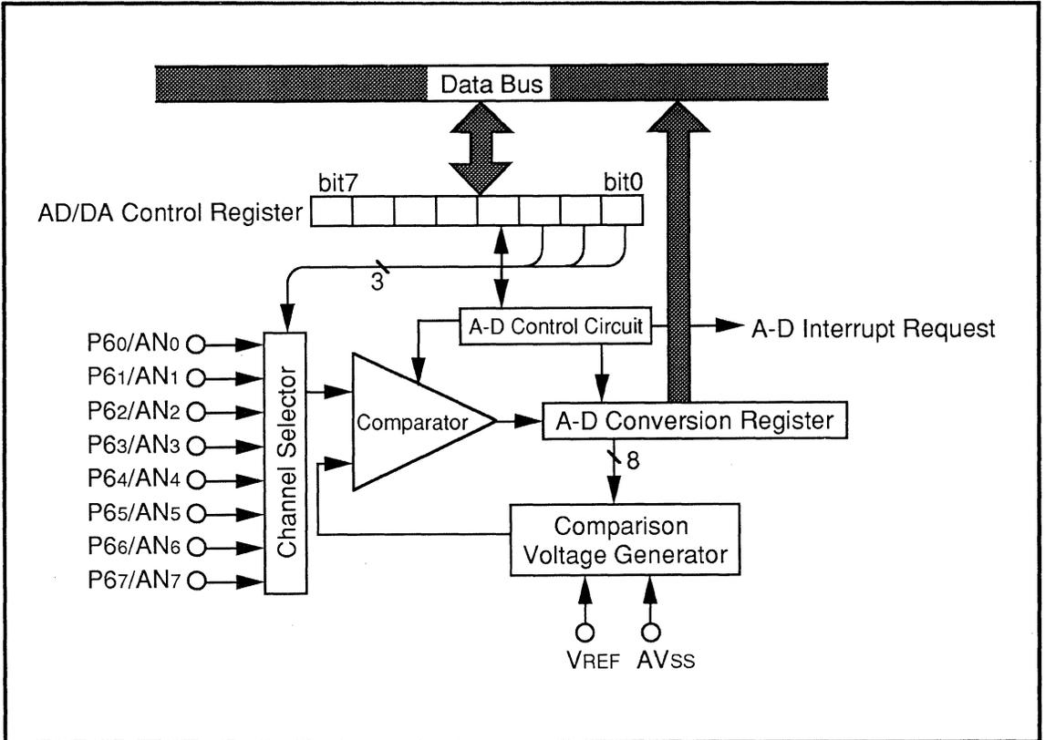
Fig. 2.9.1 Block Diagram of A-D Converter
