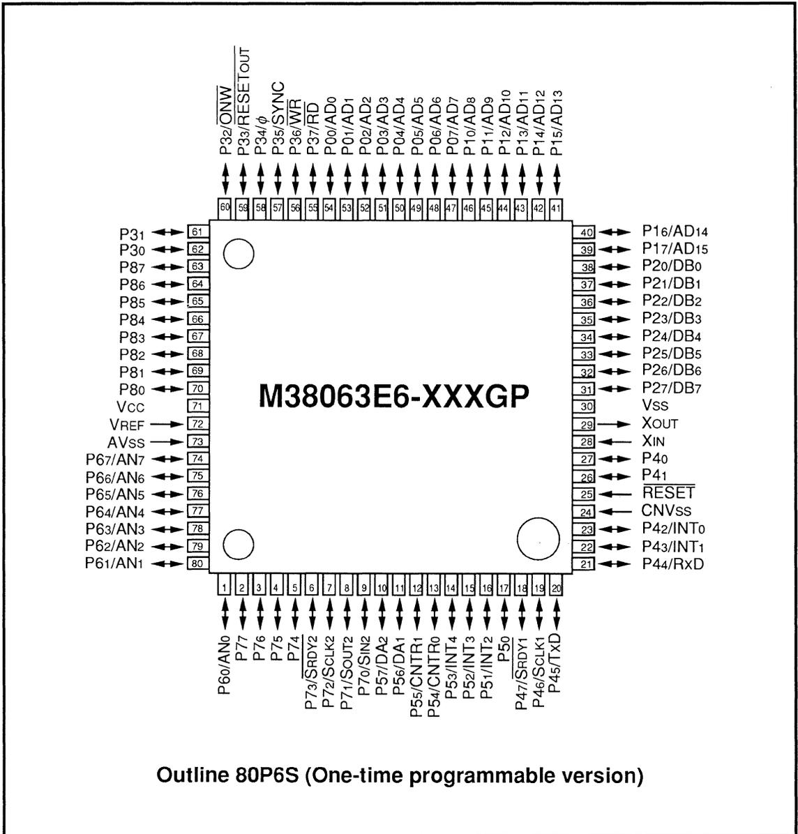
Fig. 3.2.2 0.65mm-pitch Type Pin Configuration (Top View)
