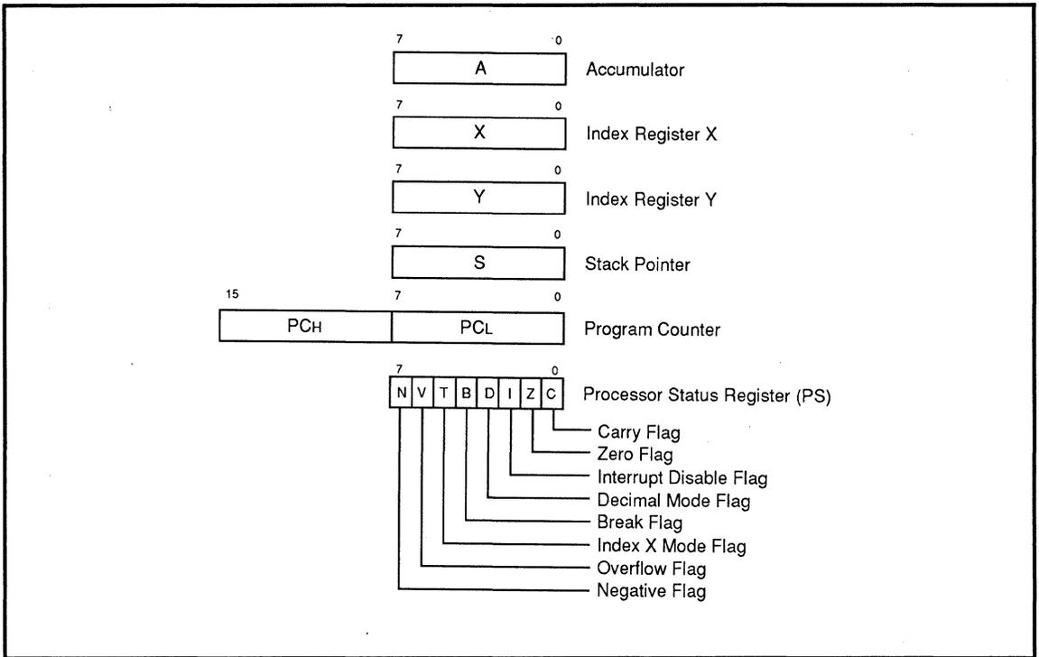
Fig. 2.1.1 Register Structure
