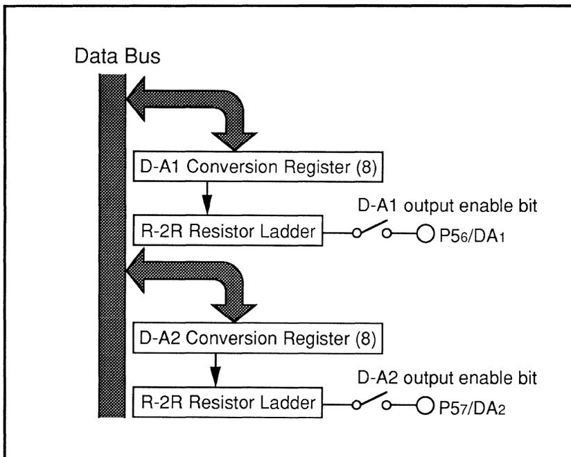
Fig. 2.10.1 Block Diagram of D-A Converter
