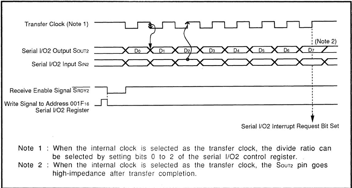
Fig. 2.8.4 Timing of Serial I/O2 Function (With LSB-First Selected)
