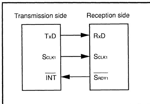
Fig. 2.7.7 Connection for Single Direction Data Transfer
