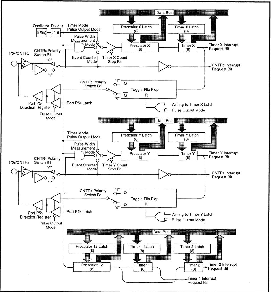
Fig. 2.6.1 Block Diagram of Timer X, Timer Y, Timer 1, and Timer 2
