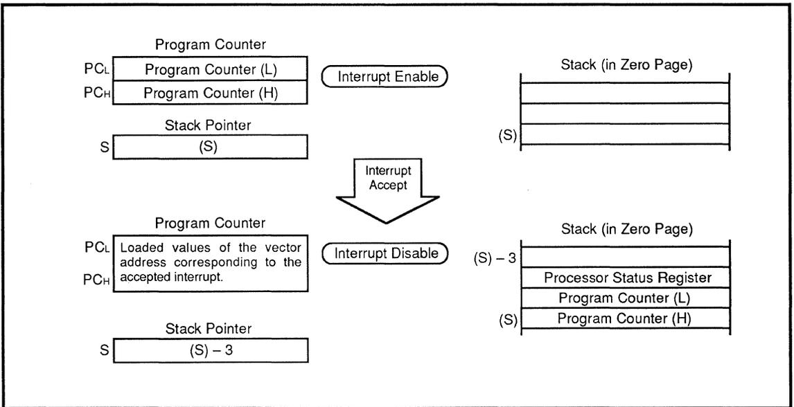
Fig. 2.5.2 Stack Pointer and Program Counter Change in Interrupt Sequence
