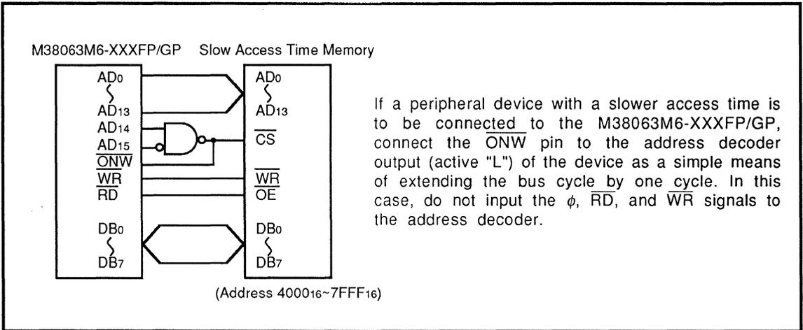
Fig. 2.4.5 Example of Circuit Using the  $\overline{\text{ONW}}$  Function
