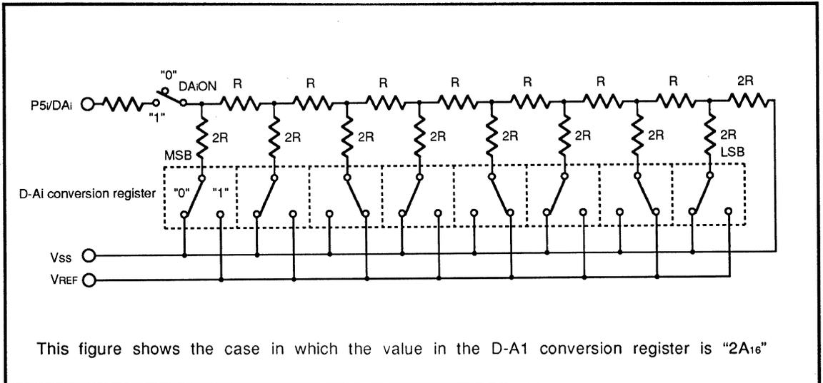
Fig. 2.10.2 Equivalent Connection Circuit of D-A Converter
