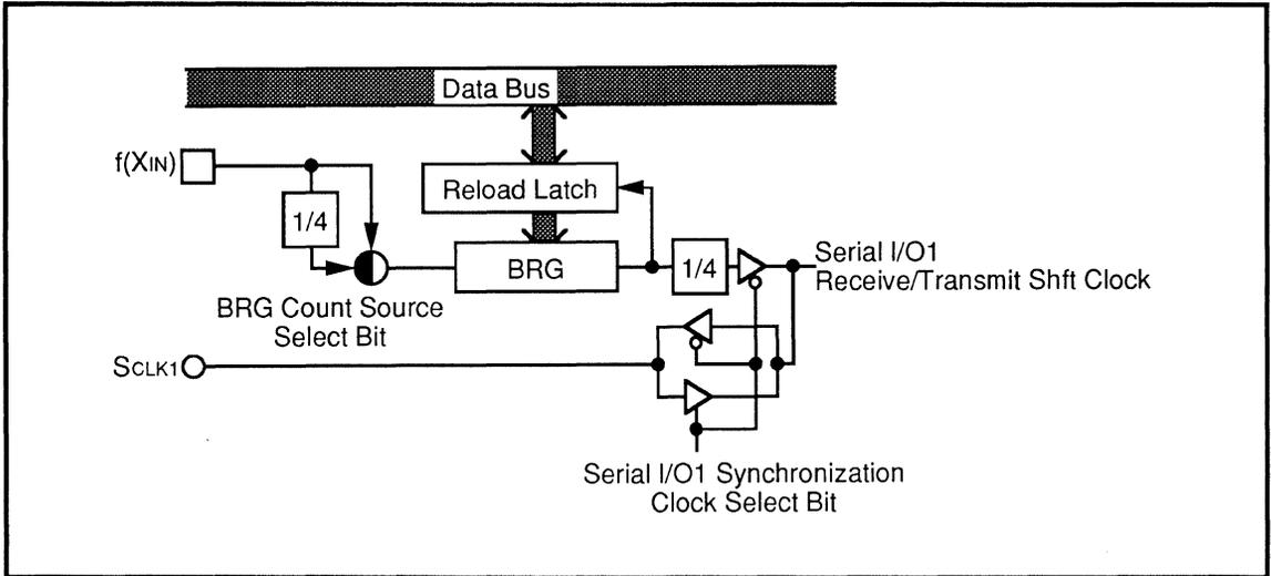
Fig. 2.7.2 Block Diagram of Baud Rate Generator
