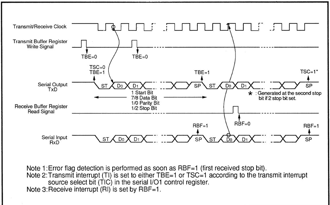
Fig. 2.7.11 Timing of Clock Asynchronous Serial I/O Function
