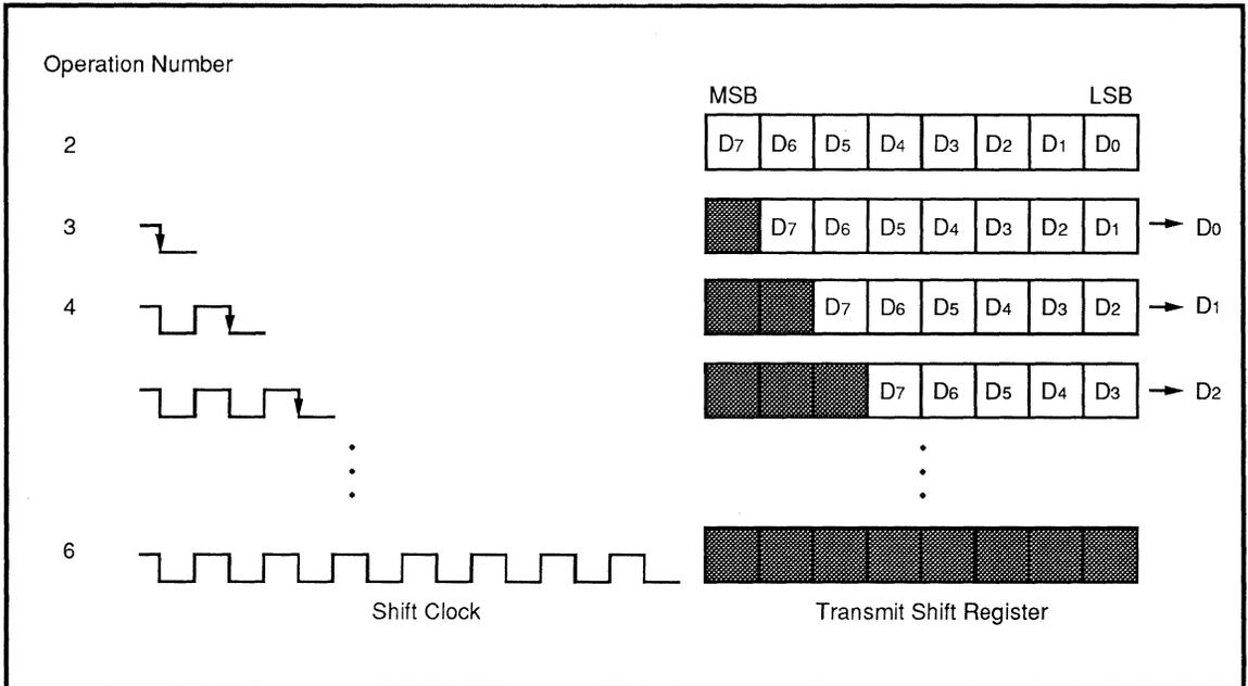
Fig. 2.7.4 Serial I/O1 Transmitter Operation
