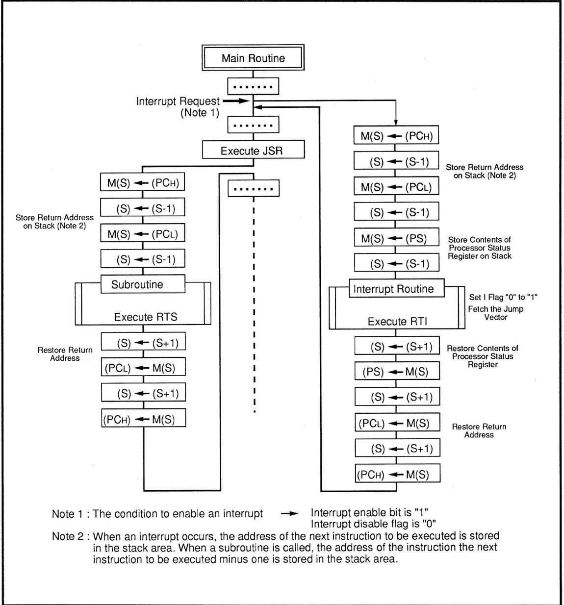
Fig. 2.1.2 Register Push and Pop when servicing interrupts and calling subroutines
