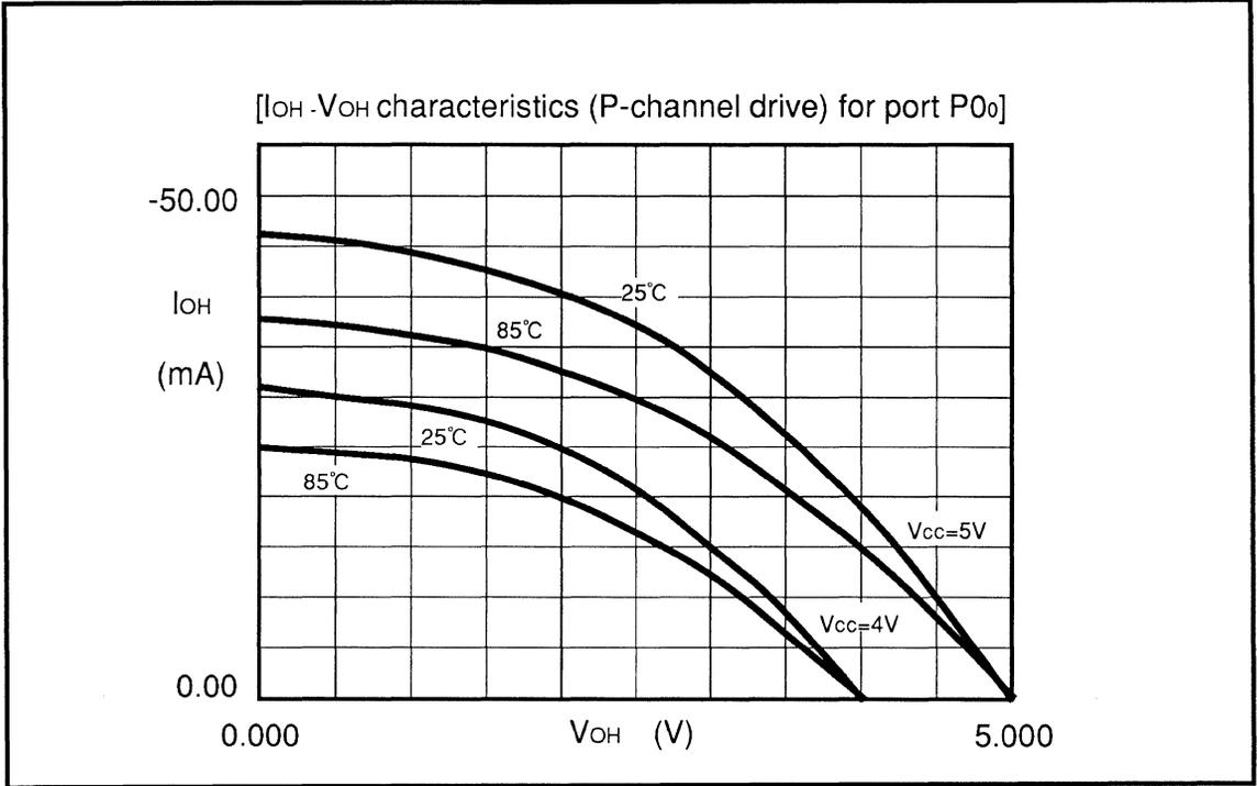
Fig. 5.2.2 Typical Characteristics of Port P0 P-Channel Output Transistor
