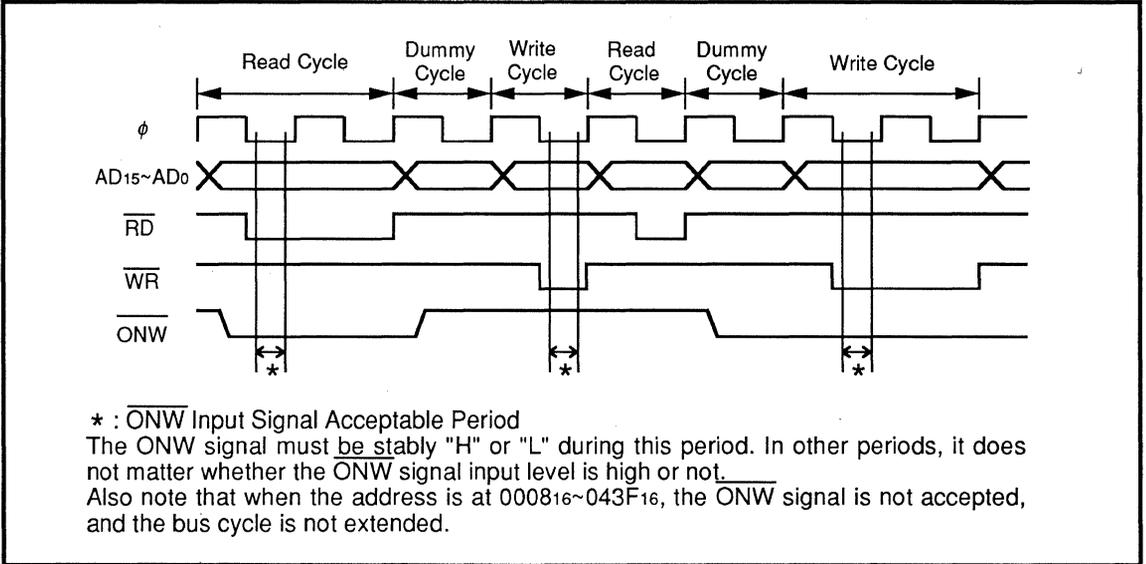
Fig. 2.4.4  $\overline{\text{ONW}}$  Function Timing
