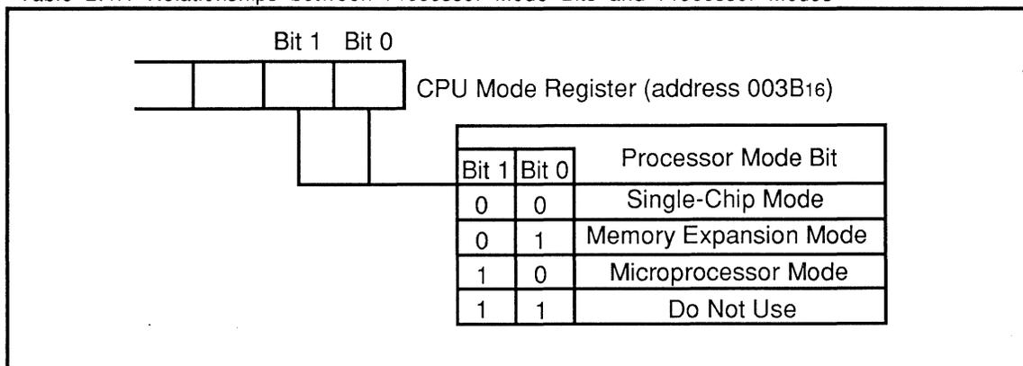
If the system is reset with the CNV<sub>SS</sub> pin connected to V<sub>CC</sub>, the processor mode bits are automatically set to (1, 0), and the system will operate only in microprocessor mode.
