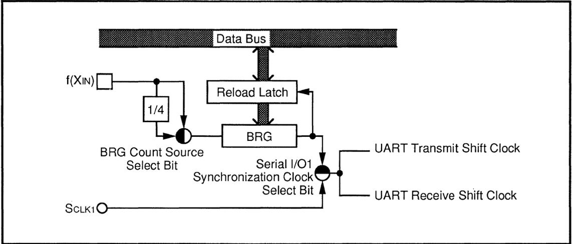
Fig. 2.7.9 Structure of Baud Rate Generator
