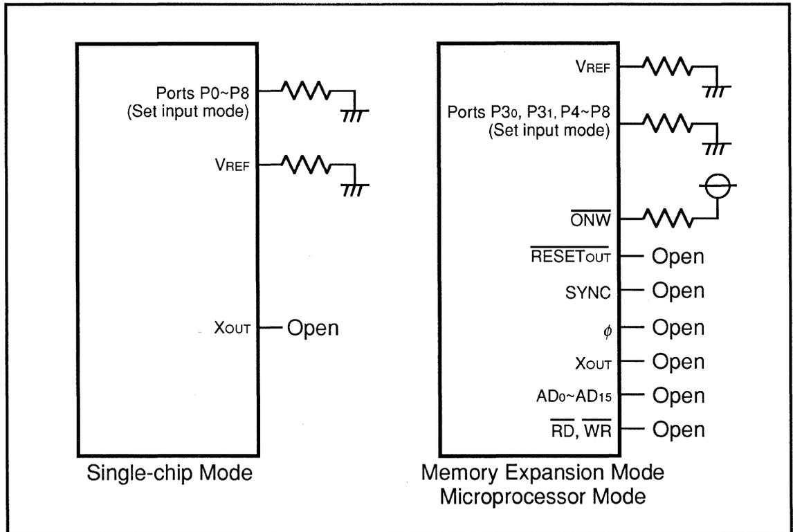
Fig. 1 Example of Handling of Unused Pins in the M38063M6-XXXXFP/GP
