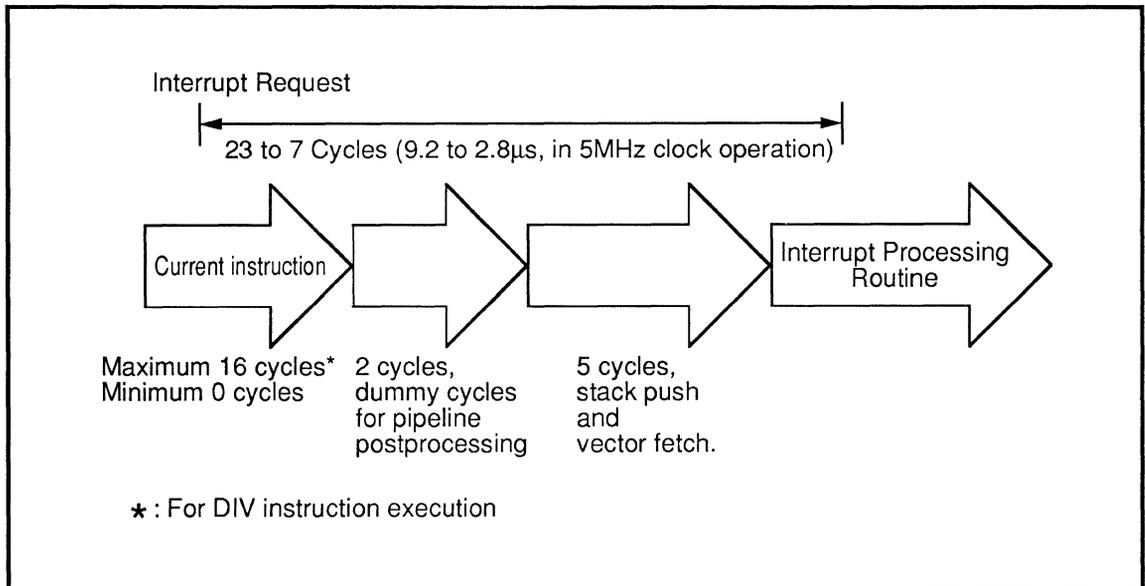
Fig. 2.5.4 Execution Time prior to Interrupt Service Routine
