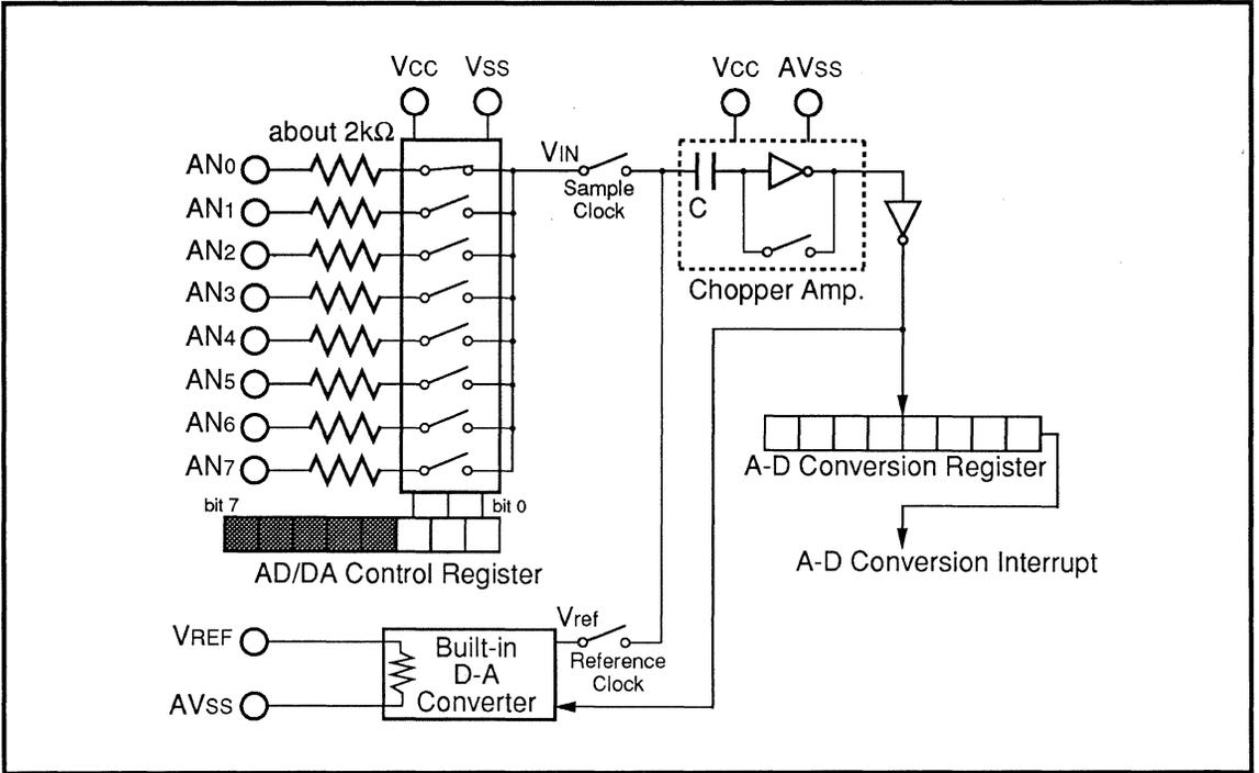
Fig. 2.9.3 Equivalent Connection Circuit of A-D Converter
