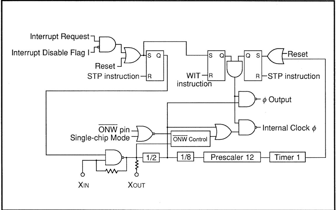
Fig. 2.12.1 Block Diagram of Clock Generation Circuit
