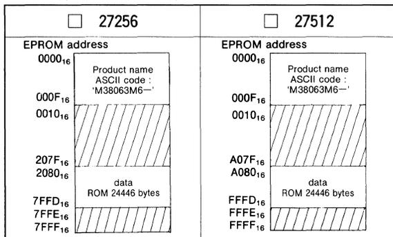
In the address space of the microcomputer, the internal ROM area is from address A080<sub>16</sub> to FFFD<sub>16</sub>. The reset vector is stored in addresses FFFC<sub>16</sub> and FFFD<sub>16</sub>.
