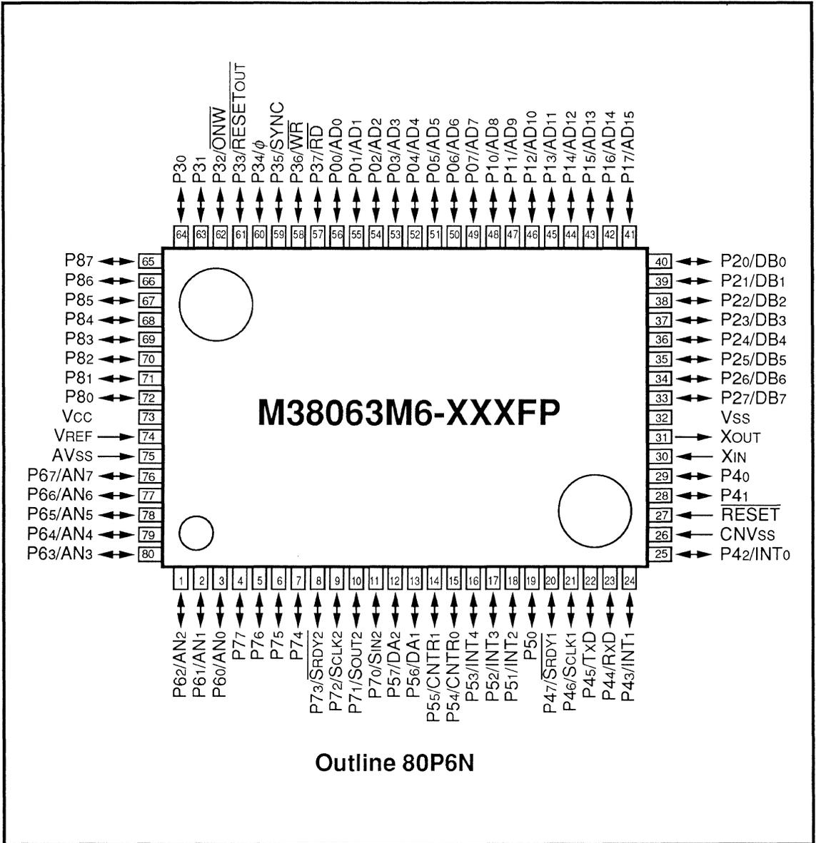
Fig. 1.3.1 M38063M6-XXXFP Pin Configuration (Top View)
