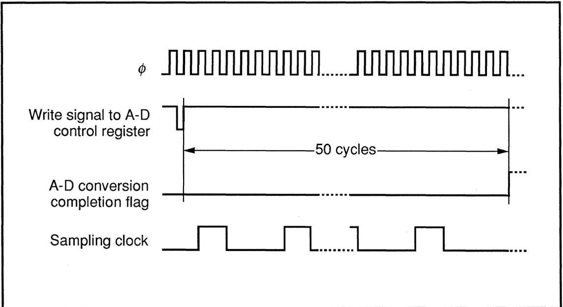
Fig. 2.9.4 Timing of A-D Conversion
