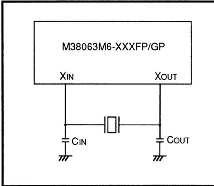
Fig. 2.12.2 Example of Oscillation Circuit
