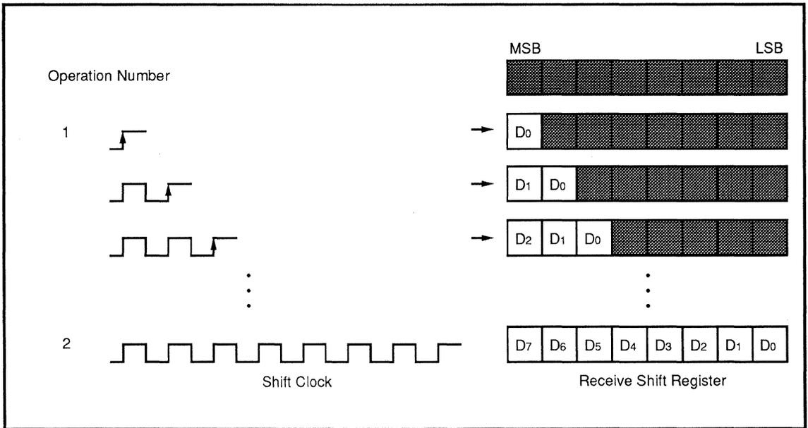
Fig. 2.7.3 Serial I/O1 Receiver Operation
