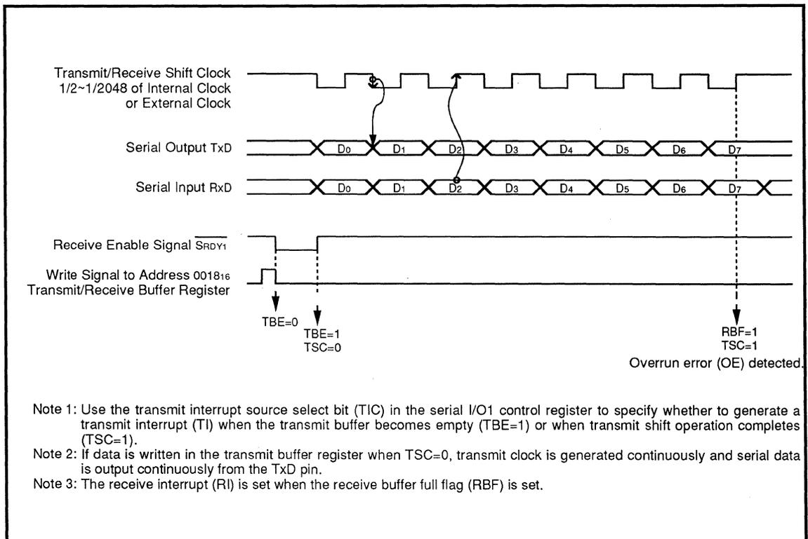
Fig. 2.7.5 Timing of Clock Synchronous Serial I/O1 Function
