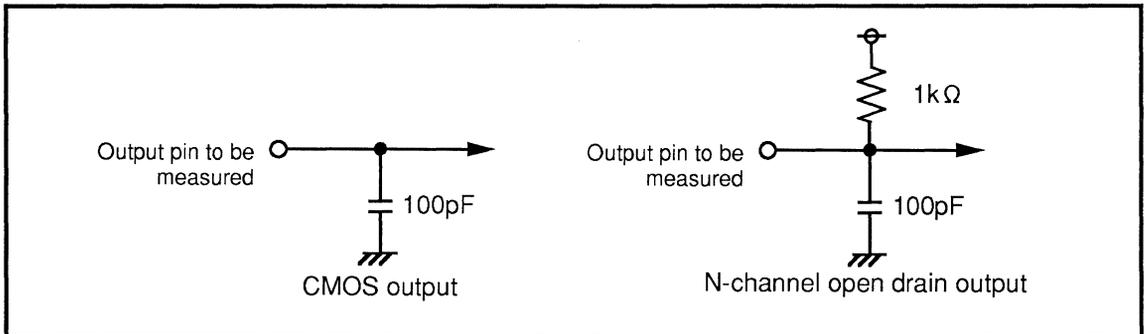
Fig. 5.1.1 Circuit for Measuring Output Switching Characteristics
