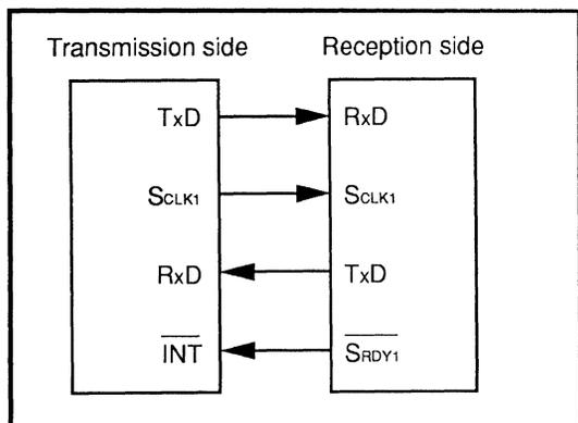
Fig. 2.7.6 Connection for Full Duplex Data Transfer
