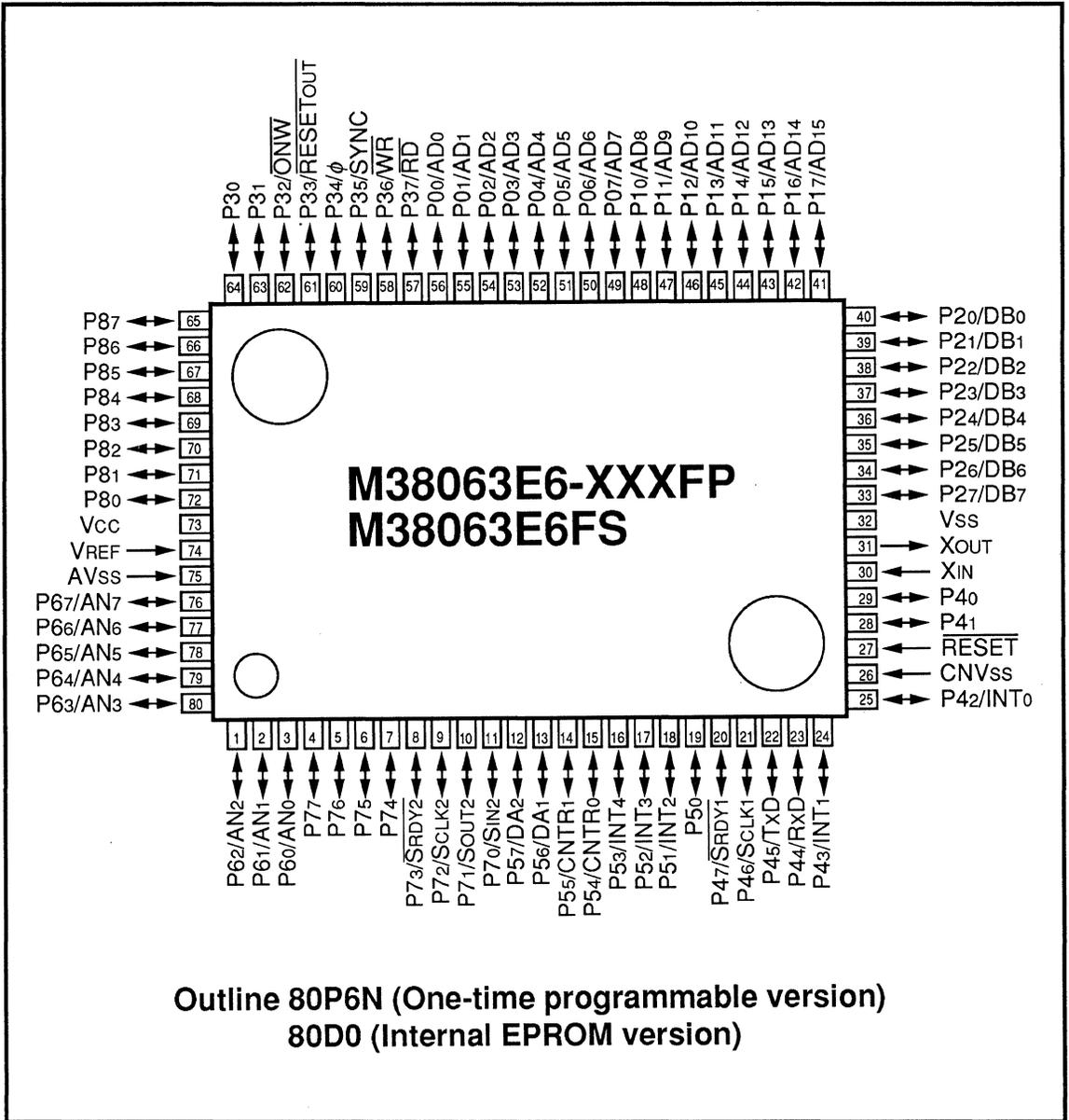
Fig. 3.2.1 0.8mm-pitch Type Pin Configuration (Top View)
