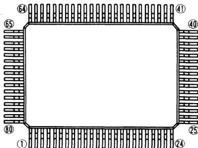
Note1: If the special mark is to be printed, indicate the desired layout of the mark in the left figure. The layout will be duplicated as close as possible. Mitsubishi lot number (6-digit) and mask ROM number (3-digit) are always marked.
