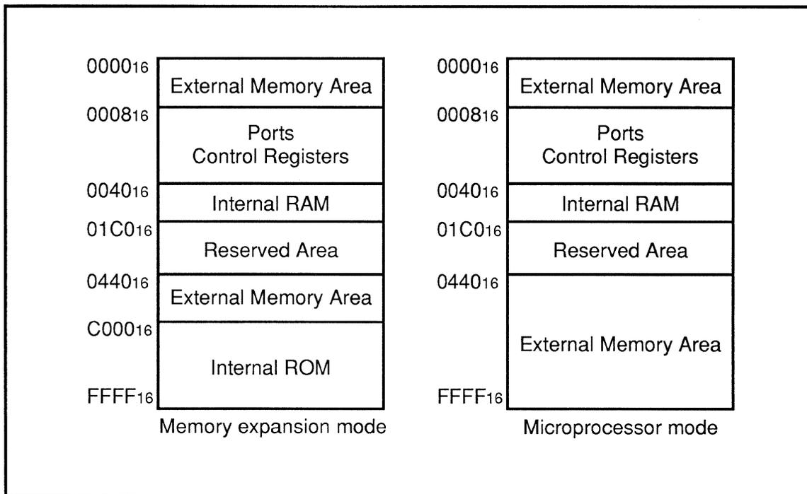
Fig. 2.4.2 Memory Allocations in Non-Single-Chip Modes
