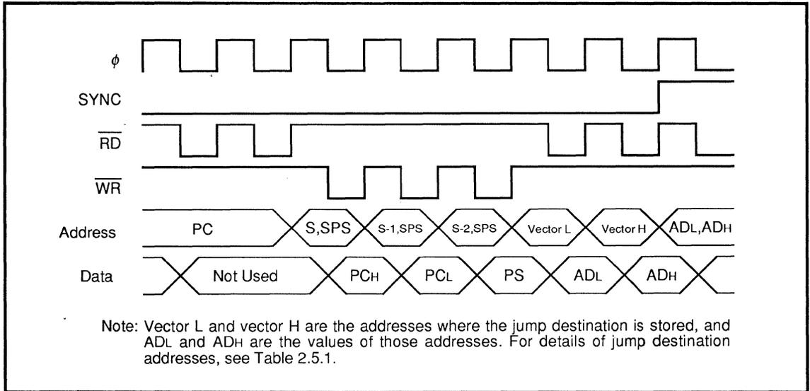
Fig. 2.5.3 Timing after Interrupt
