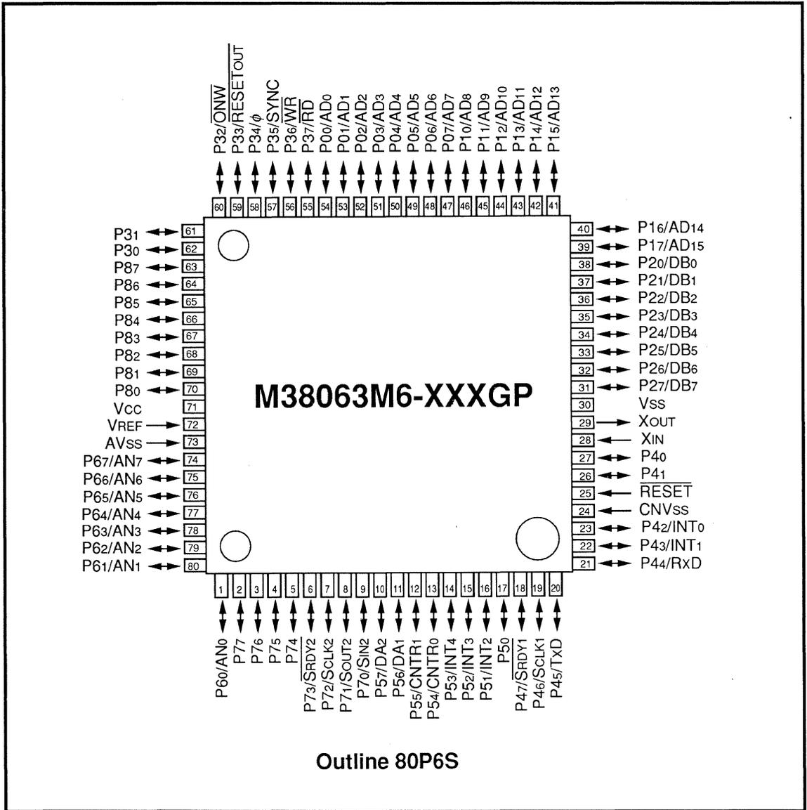
Fig. 1.3.2 M38063M6-XXXGP Pin Configuration (Top View)
