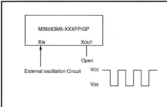
Fig. 2.12.4 External Clock Input Circuit
