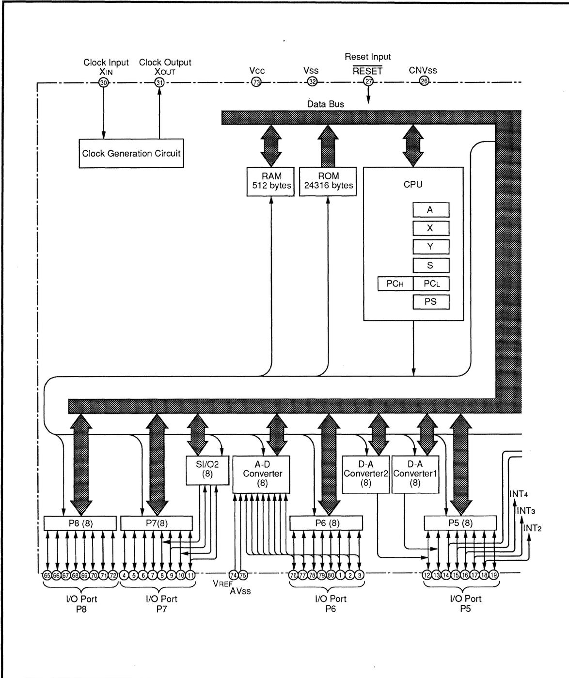
Fig. 1.5.1 Functional Block Diagram of M38063M6-XXXFP
