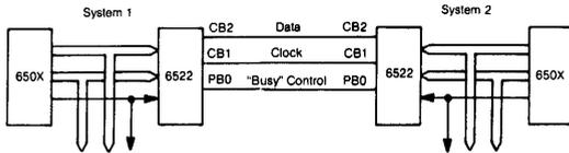
**Figure 17. Using Shift Register for Inter-System Communication**
