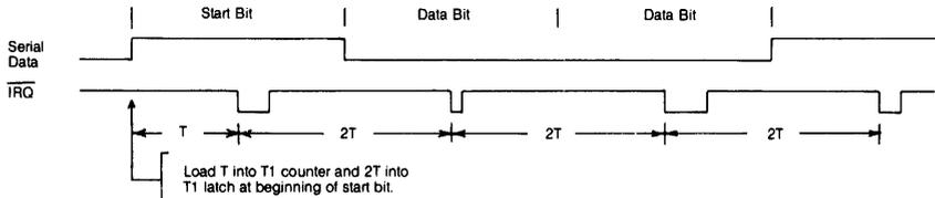
**Figure 14. Detecting Asynchronous Data Using Timer 1**
