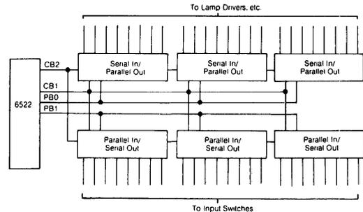
**Figure 19. Expanding System I/O Using Shift Register**
