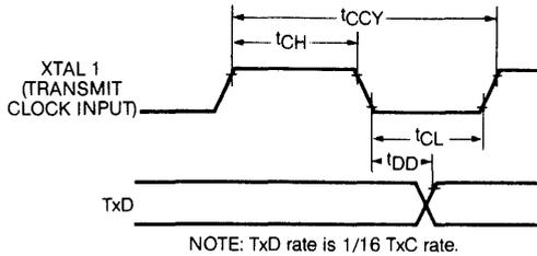
**Figure 4a. Transmit Timing with External Clock**
