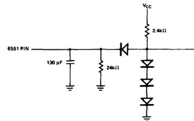
**Test Load for Data Bus (DB<sub>0</sub>-DB<sub>7</sub>)
