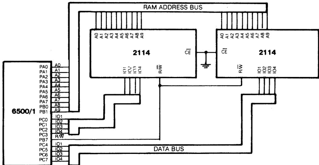
Figure 1 — Schematic for 1K Byte Expansion
