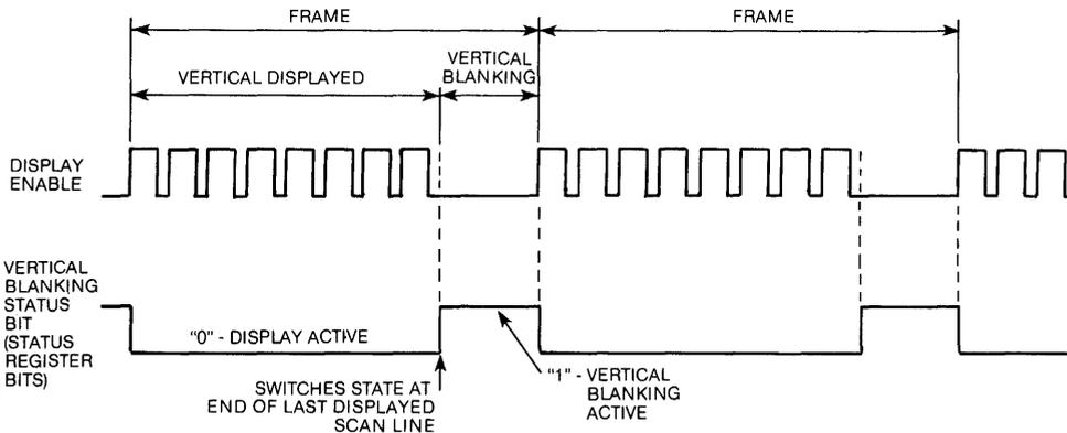
**Figure 8. Operation of Vertical Blanking Status Bit**
