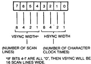
Control of these parameters allows the 6545-1 to be interfaced to a variety of CRT monitors, since the HSYNC and VSYNC timing signals may be accommodated without the use of external one-shot timing.
