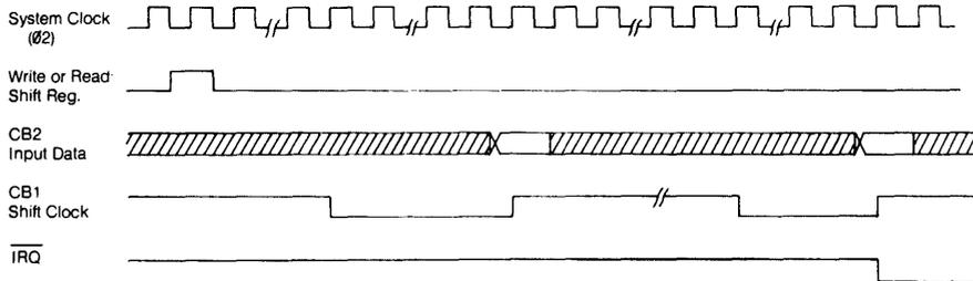
Figure 8. Shifting in Under Control of T2
