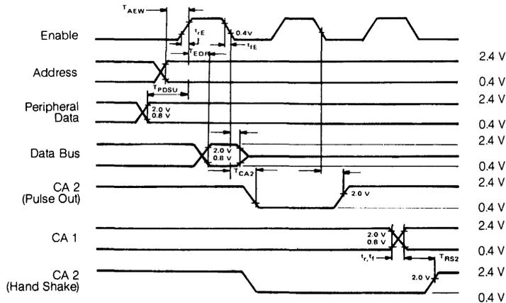
**FIGURE 2 — WRITE TIMING CHARACTERISTICS**
