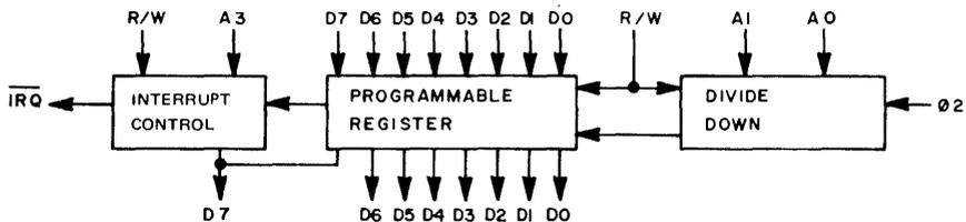
**Figure 4. Basic Elements of Interval Timer**
