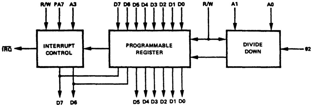
The interval time can be programmed to count up to 255 time intervals. Each time interval can be either 1T, 8T, 64T or 1024T increments, where T is the system clock period. When a full count is reached, an interrupt flag is set to a logic "1". After the interrupt flag is set the internal clock begins counting down to a maximum of - 255T. Thus, after the interrupt flag is set, a Read of the timer will tell how long since the flag was set up to a maximum of 255T.
