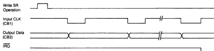
Figure 13. Shifting out under Control of External Clock
