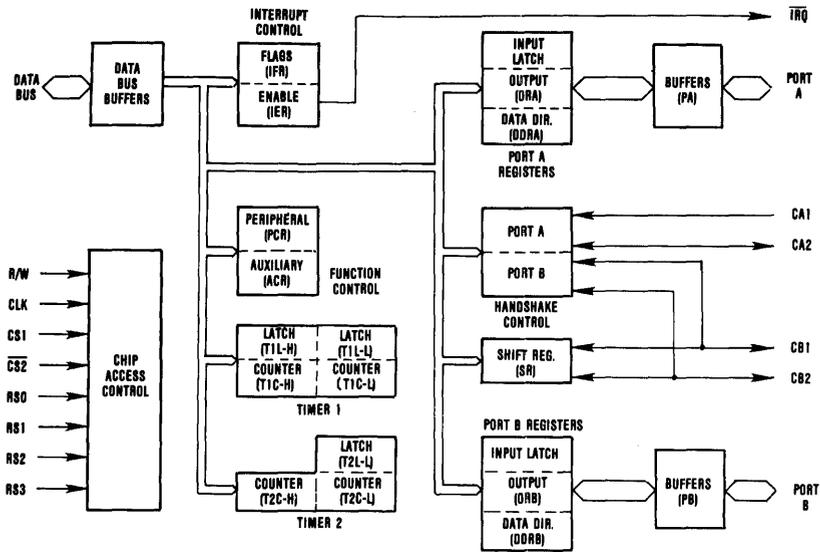
Figure 1. 6522 Block Diagram
