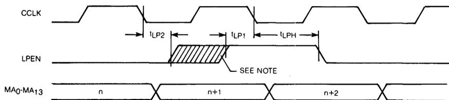
NOTE: "Safe" time position for LPEN positive edge to cause address n+2 to load into Light Pen Register.
