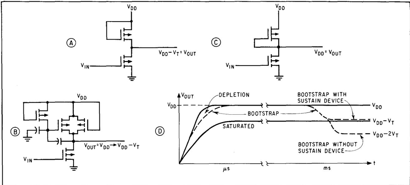
**3. Widest swing.** Depletion-mode inverter circuit, C, attains  $V_{DD}$  as most negative output level, while bootstrap circuit, B, and enhancement-mode inverter, A, do not offer as wide a range on a dc basis. Depletion-mode circuit also has best speed-power product.
