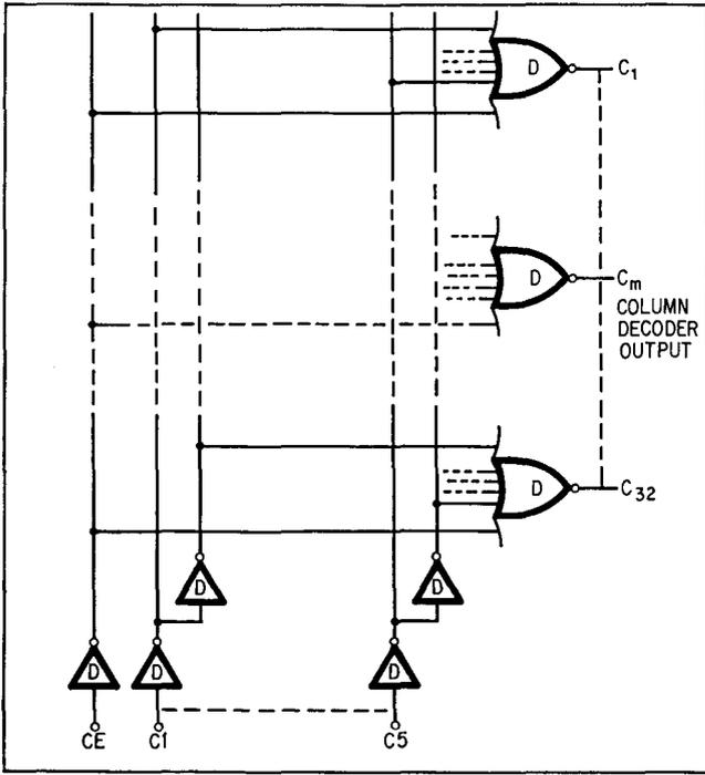
**6. Column decoder.** Depletion-load inverters drive depletion-mode NOR gates. Decoder uses 32 six-input NOR gates. Selected column is driven by one gate (the only one that provides an output at  $V_{DD}$ ). D indicates circuits with depletion-mode devices.
