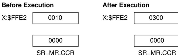
**Explanation of Example:** Prior to execution, the 16-bit X memory location X:\$FFE2 (I/O Port B Data Register) contains the value \$0010. Execution of the instruction tests the state of the bits 4,8,9 in X:\$FFE2, does not set the carry bit C in CCR because all of these bits were not set, and then complements the bits.
