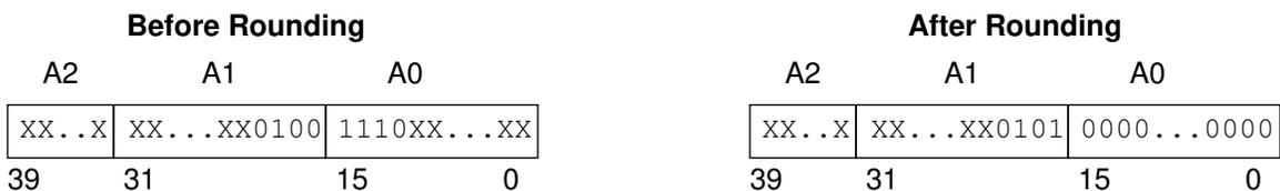
**Figure 3-12 Two's Complement Rounding (No-scaling)**
