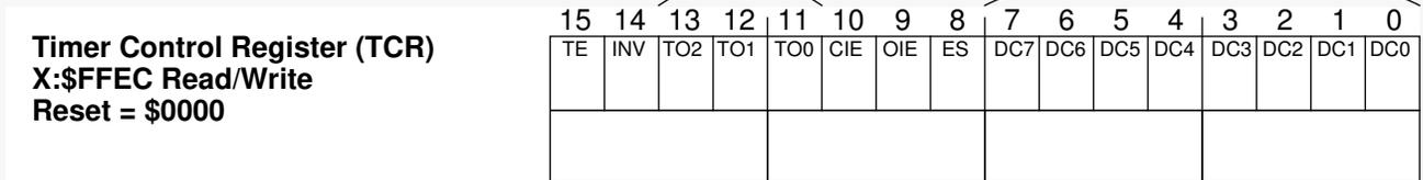
Figure C-8 Timer Control Register (TCR)
