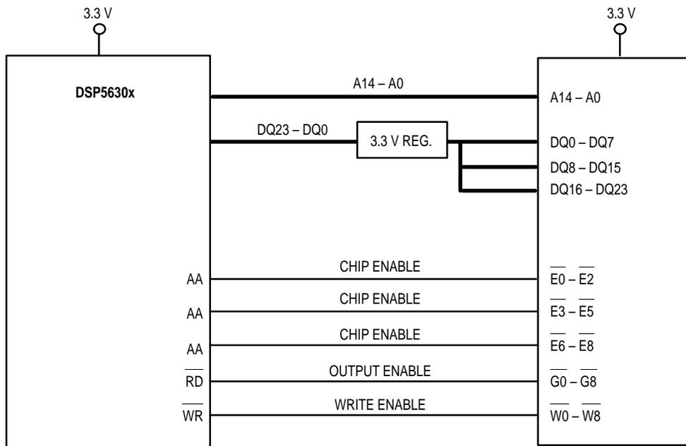
Figure 4. DSP5630x Connection to (32K x 8) Based Module on X, Y, or P Memory
