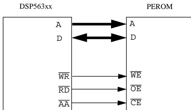
On the DSP56303EVM, the code in flash memory is run at reset. Though the following sections do not give an example of Flash PEROM usage, the program `flash.asm` is included with all DSP563xxEVMs. This program allows you to download any desired program into the flash memory so that it can be run at processor reset. Information on using `flash.asm` is given in each EVM/ADM user's manual.
