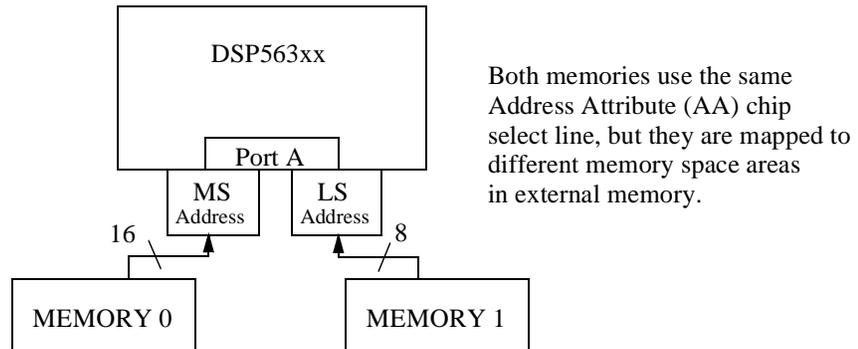
The EVM boards are not set up for Address Muxing (i.e. with different memories connected to the same address line as diagrammed in **Figure 2-3**), so Address Muxing is simulated in this example. We use the same memory setup as in previous examples, but when the external access occurs, only eight of the address bits are used. As **Figure 2-4** shows, this example sends data from Y:\$0 to P:\$200000 using DMA.
