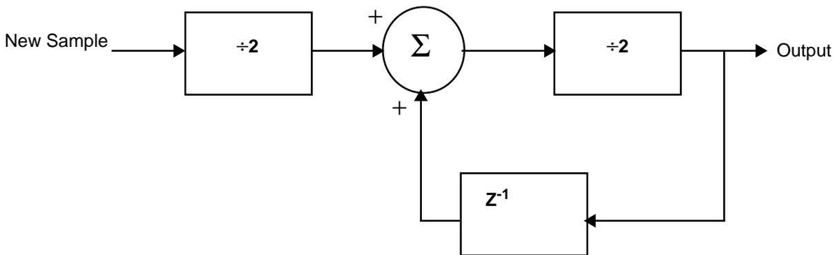
**Figure 3.** Block Diagram of a Delayed Sample (Echo)
