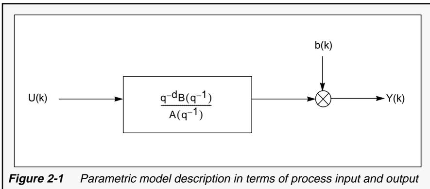
**Figure 2-1** Parametric model description in terms of process input and output
