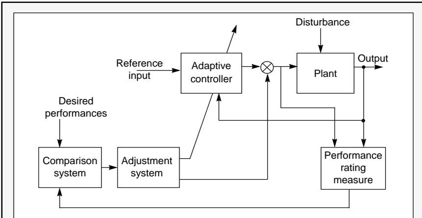
**Figure 1-1 Basic principles of adaptive control**
