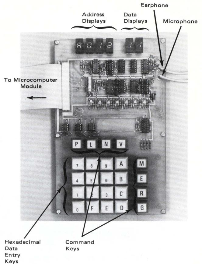
FIGURE 1-1-3b. Keyboard/Display Module
