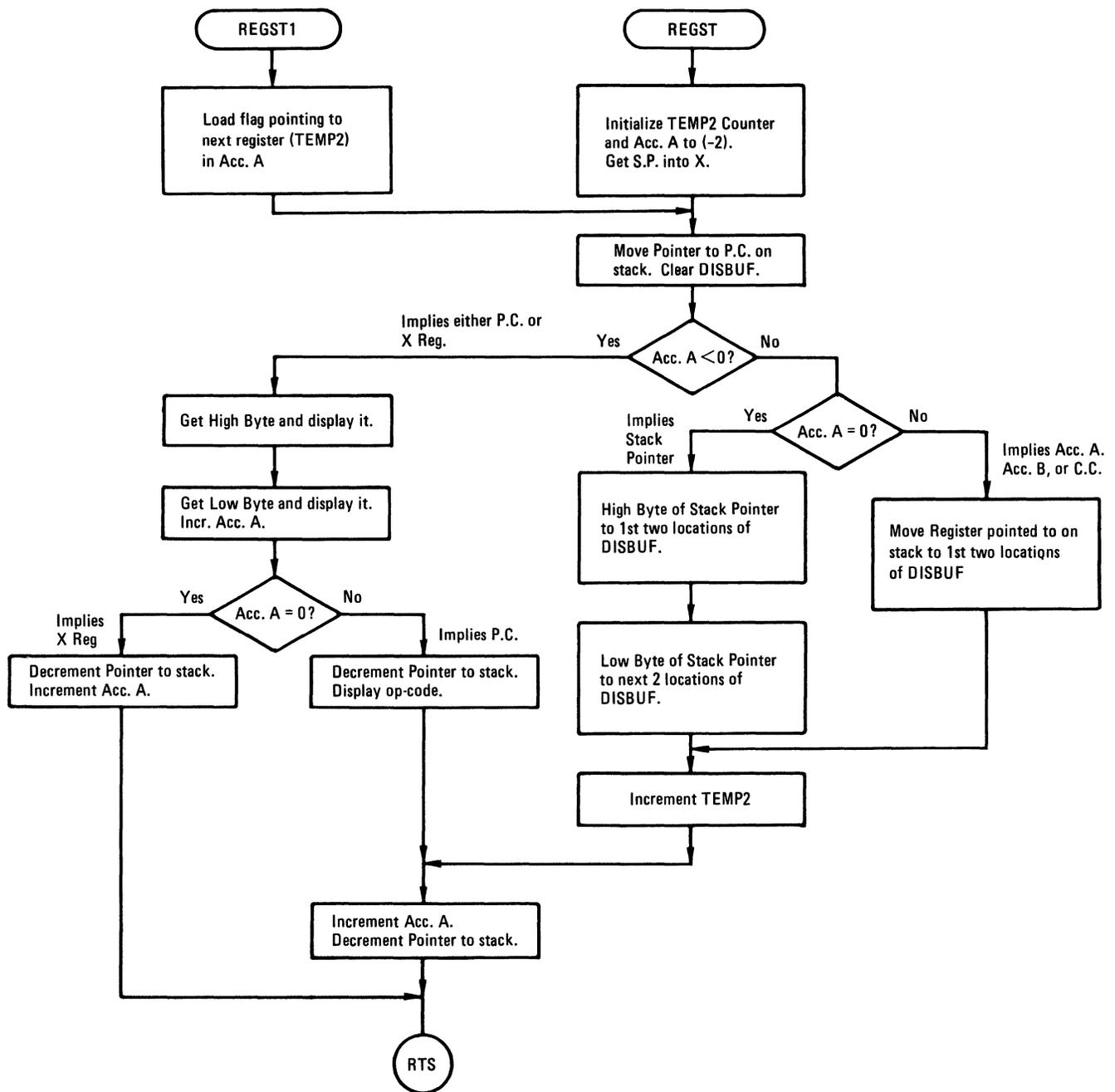
FIGURE 3-6-1. Program Flow for Register Display Function
