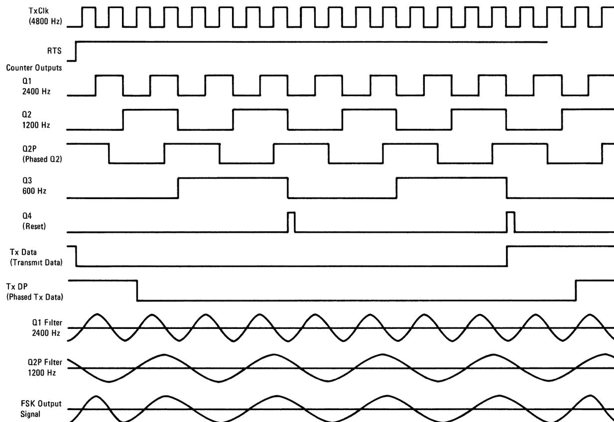
FIGURE 2-7-2. Transmit Waveforms
