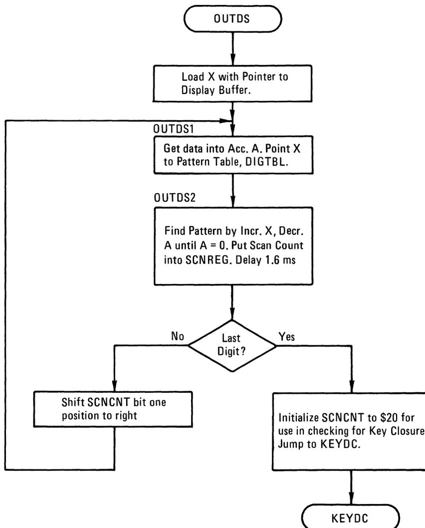
FIGURE 3-3-1. Program Flow for Output Display Routine
