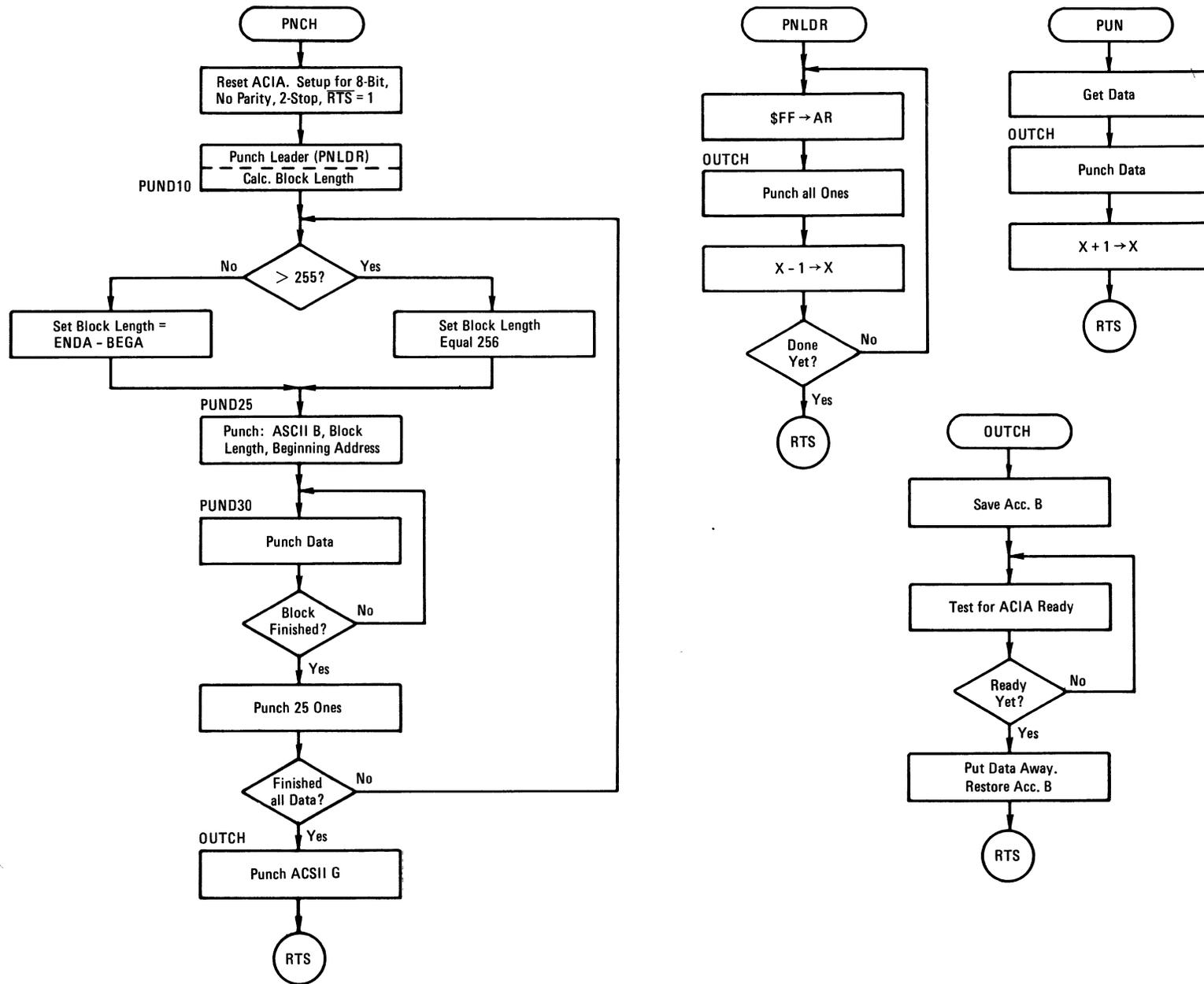
FIGURE 3-7-1. Program Flow for PUNCH Function
