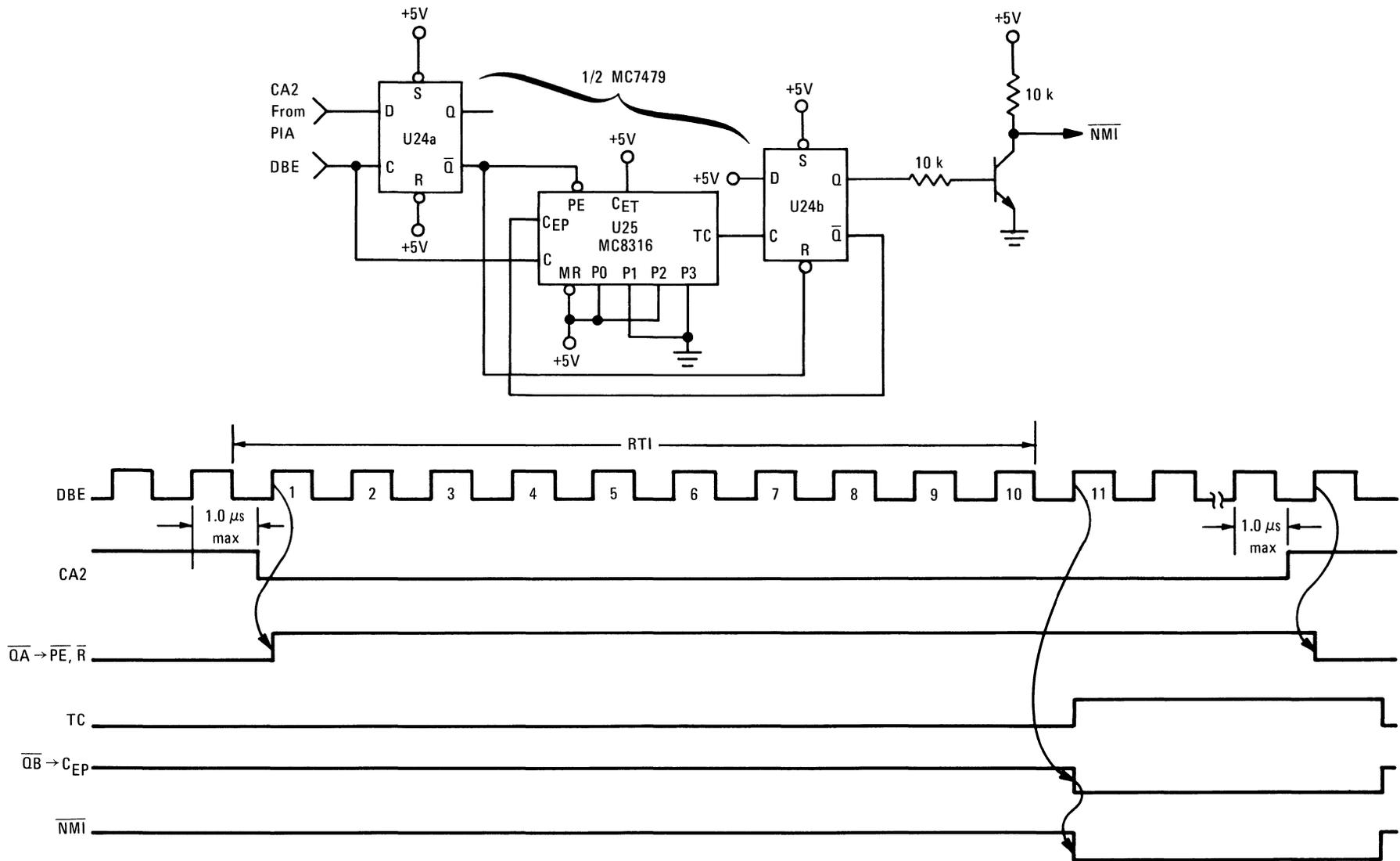
FIGURE 2-6-1. Trace Circuitry and Timing Waveforms
