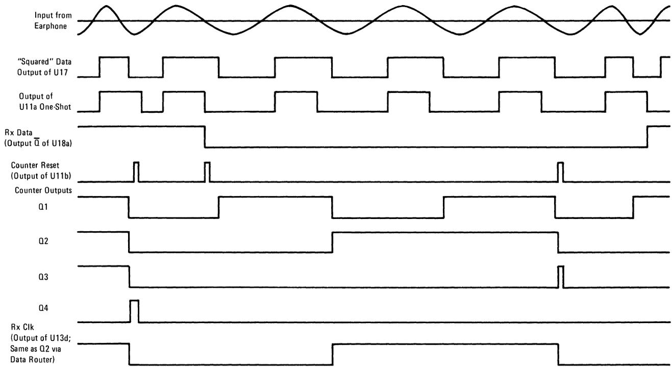
**FIGURE 2-7-4. Receive Waveforms, Mark-to-Space Transition**
