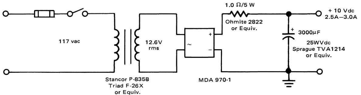
Note: Ground filter capacitor return lead near negative terminal of rectifier to minimize ground loops.
