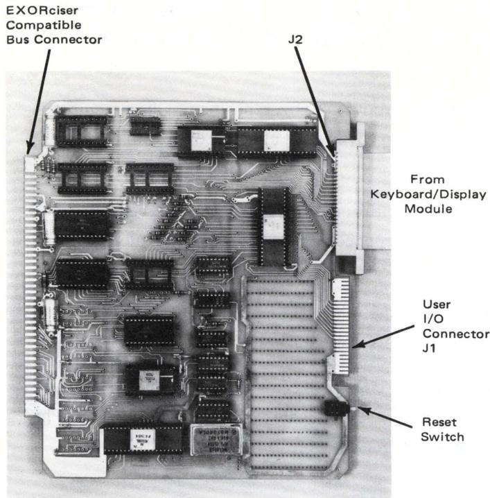
FIGURE 1-1-3a. Microcomputer Module
