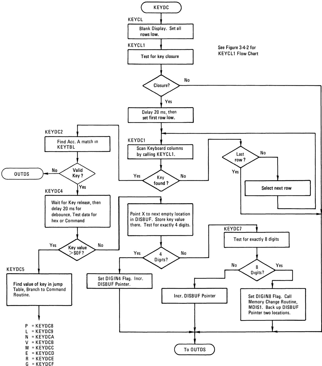
FIGURE 3-4-1. Program Flow for Keyboard Scan and Decode Routine
