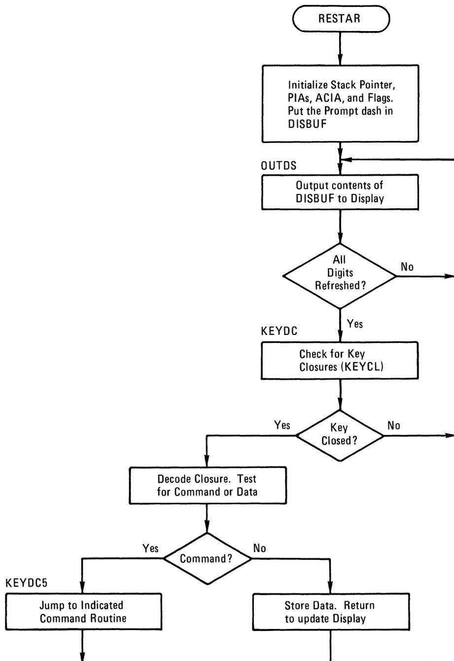
FIGURE 3-1-1. Overall Program Flow for JBUG Monitor
