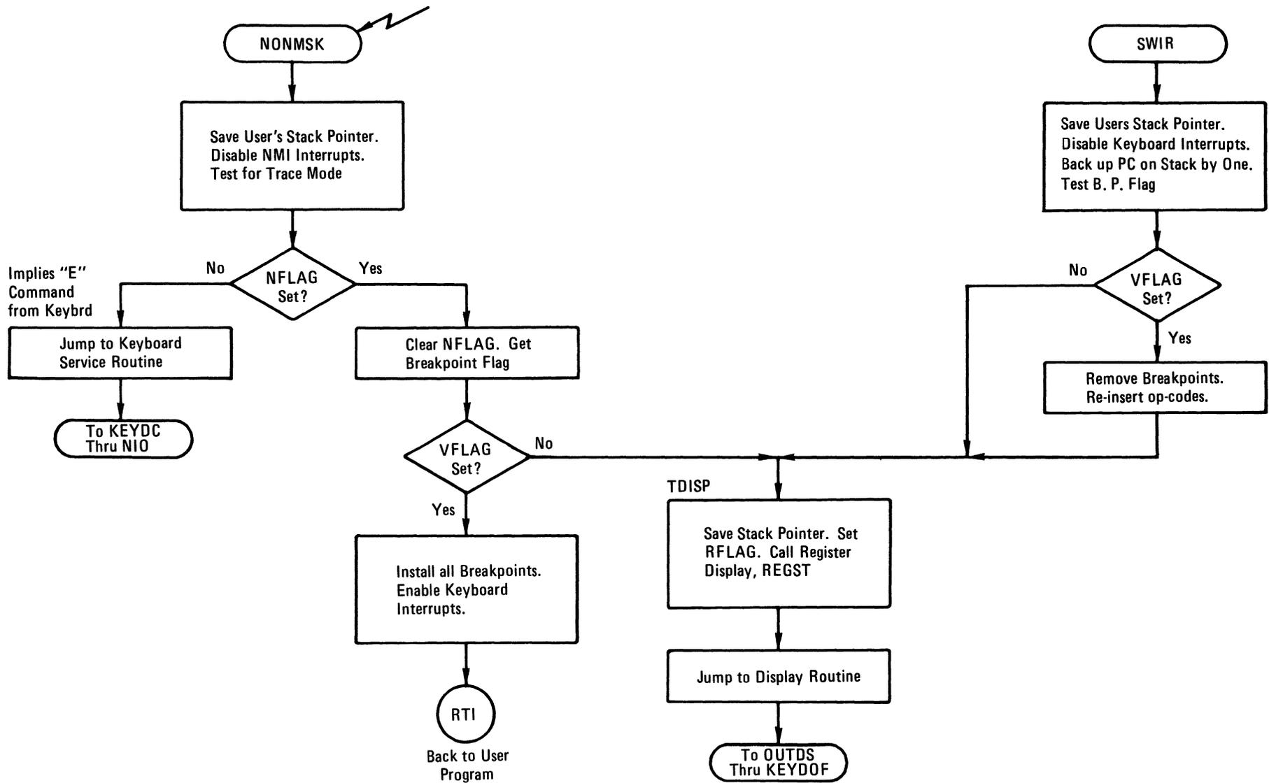
FIGURE 3-8-1. Program Flow for NMI and SWI Interrupt Handling
