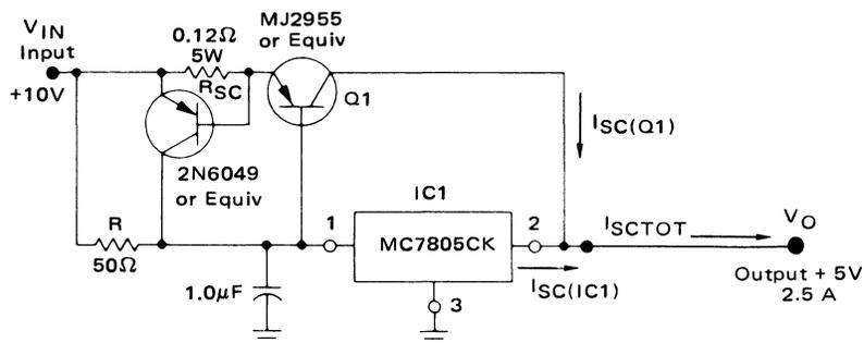
R: used to divert IC regulator bias current and determines at what output current level Q1 begins
