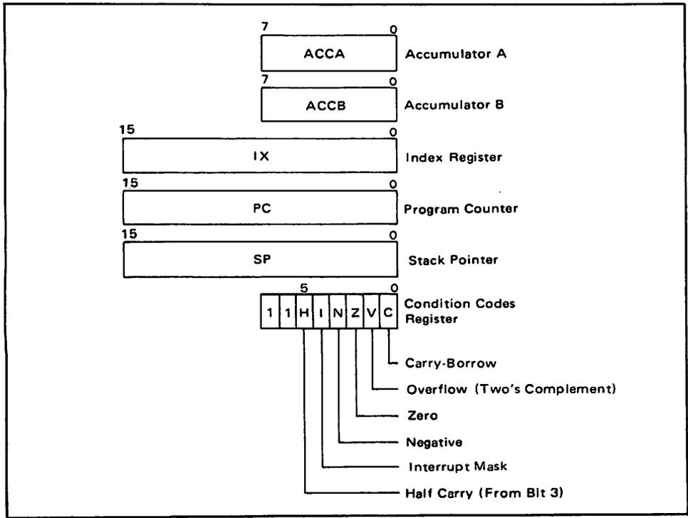
FIGURE 2-2. Programming Model of the M6800 Microprocessor
