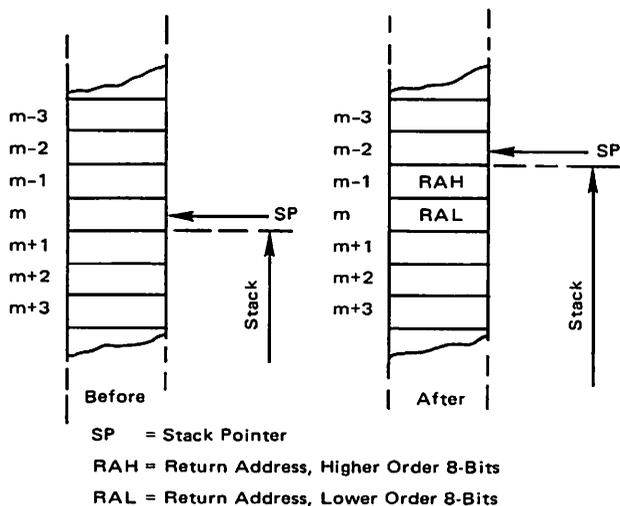
FIGURE 3-4. Saving a Return Address in the Stack
