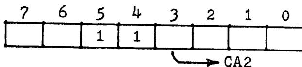
Assume that to communicate with some external device CA2 is to go to the HIGH state for 1 millisecond, then go LOW. Also assume that the instruction JSR MILSEC (subroutines will be covered in the next chapter) will cause a delay of 1.0 milliseconds. Write the necessary instructions assuming that CA2 is presently LOW.
