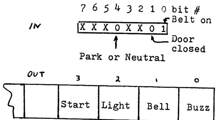
By grouping the Gear Shift and Door checks together the single instruction BIT A #00010010 will cause a branch via BEQ OKTOGO if and only if both bits are 0.
