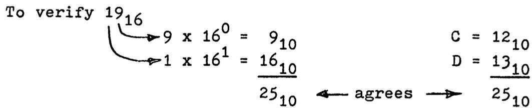
To add 2 column hex numbers each column is added separately, as in decimal. If the right column produces a carry it is added to the left column
