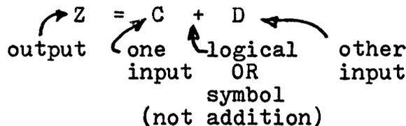
The instruction ORA A #5C will perform the logical OR operation with ACC A contents and the mask word, 08, as inputs. The result will reside in ACC A. If 144A contains \$CA, what will be the result after execution of
