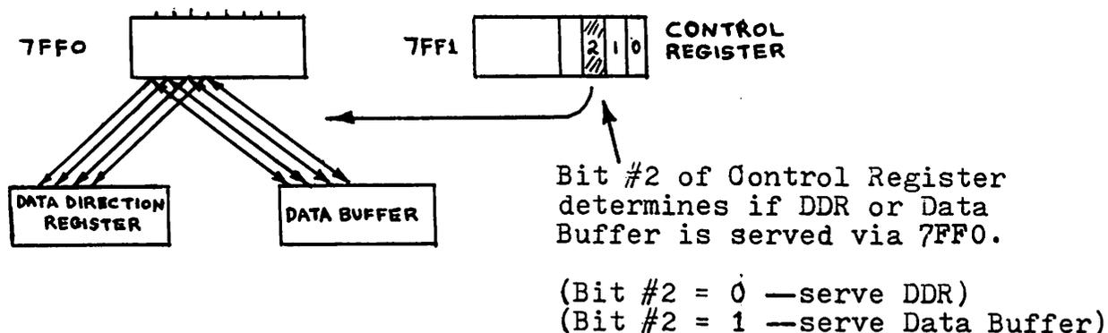
Let's assign symbolic addresses to these two memory addresses, PIABFA being the "A" half Data Buffer (and DDR too) at address 7FF0. Similarly PIACRA would be the "A" half of Control Register at 7FF1. For the "B" half the corresponding symbolic addresses would be PIABFB (Data Buffer and DDR) at 7FF2, and PIACRB (Control Register) at 7FF3.
