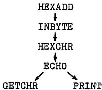
When HEXCHR detects an invalid hex character the C bit is set and HEXCHR returns to INBYTE. INBYTE immediately checks the C bit and, noting that the C bit is set, returns immediately to HEXADD, which also checks the C bit. HEXADD, on noting that the C bit is set, immediately restarts. In summary, a wrong key immediately restarts HEXADD, preferably after a printed message such as BAD HEX.
