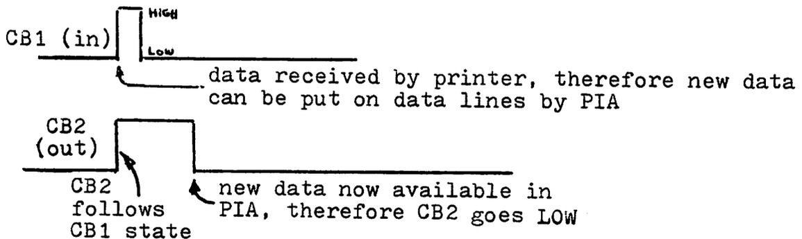
Again the hand shaking operation permits optimum data flow. Although the printer would not normally store more than 132 characters for one complete line of text, the data rate within this line could be as high as 50 000 characters/second, limited by the computer's clock and the number of instructions per loop.
