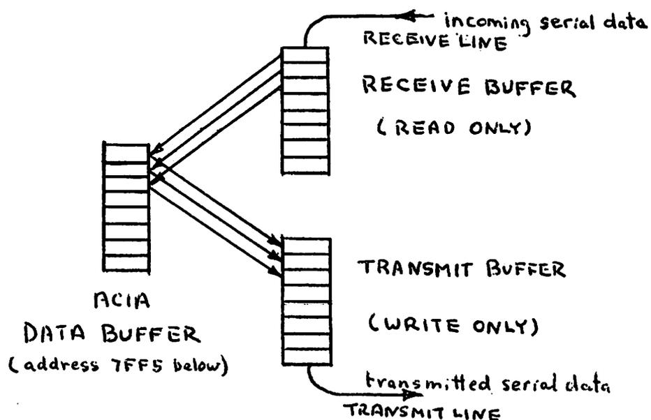
Write an instruction which sends data, now in ACC A to the ACIA where it will be automatically put into serial form and transmitted to some external device.
