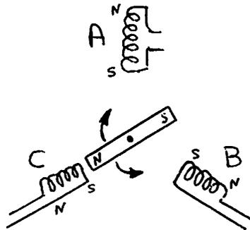
Each of electromagnets A, B and C are directly under control of a PIA Data Buffer bit, as shown in the diagram below. A magnet is ON when the appropriate bit is in the 1 state, and OFF when the bit is 0. Energizing magnet C causes the North pole of the central magnet to rotate to the South pole at C.
