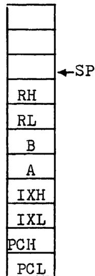
Within OBYTE sub. RH and RL are return address bytes. H = high, L = low. CCR data on the stack is overwritten but only after it is in ACC A for printing.
