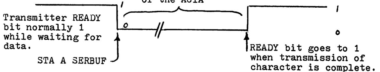
Note that the transmitter, while dormant, is normally READY, waiting for data from the computer. In contrast, the receiver in the dormant state is normally not READY, since it is waiting for new serial data from the external device.
