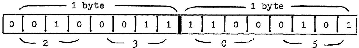
Approaching this from a "top-down" direction, assume that we have a subroutine INBYTE which would return with  $23_{16}$  in ACC A when two keys, 2 and 3, are struck. Write the subroutine HEXADD which calls INBYTE and produces the 16 bit binary contents in the two memory locations, ADDRESS and ADDRESS+1.
