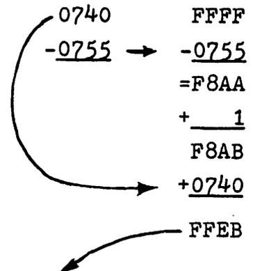
but FFEB (in 2 byte format) becomes EB in 1 byte format (see Chapter 1). Normally JMP NEXCHR rather than BRA NEXCHR would be used to avoid offset calculations.
