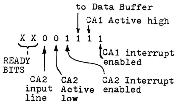
When an interrupt is produced by CA1 of the PIA the service routine is to store bits #0 to 3 of the Data Buffer in LODATA. An interrupt by CA2 should store bits #4 to 7 in HIDATA. Assume that CA1 and CA2 are the only source of interrupts. Write the service routines.
