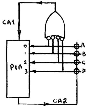
Here is an application of the PIA to detect which of the 4 keys, A, B, C or D was depressed. CA2 provides logic 0 to all 4 intersections, the depressed key passing on this 0 state to the appropriate input. The symbol at the top of the diagram is an "inverted input OR gate" whose output goes to the 1 state if one or more of the inputs go to 0. PIA lines 4 to 7 are not needed.
