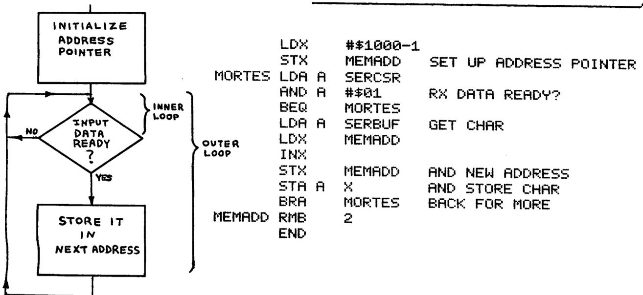
Here we see an inner loop testing the READY bit and an outer loop storing data. This is known as a "nested" loop format.
