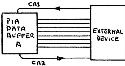
inform the PIA, acting as a data receiver, that data is now available. When this data is read by the PIA, CA2 could inform the external device that data has been read; therefore another byte could be
