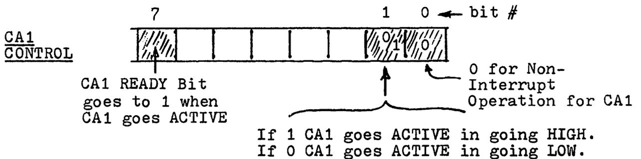
The 3 bits associated with CA1 are shown above. We are not using interrupt at this time; hence bit #0 = 0. Bit #1 determines whether CA1 sets the READY bit (#7) when CA1 goes LOW (if bit #1 = 0) or HIGH (if bit #1 = 1). The CA1 READY bit (also called IRQA1 in Motorola literature) indicates, when going to the 1 state, that CA1 has gone ACTIVE.
