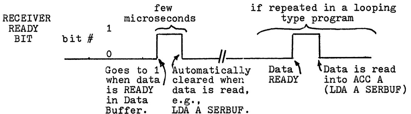
Although the rate of transmitting and receiving data bits is fixed there may be long time gaps between successive characters. Hence the term "asynchronous" in the ACIA, meaning no specified number of characters per second.
