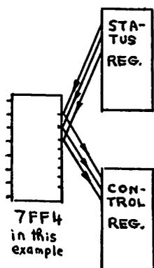
Selection of data rates and control operations are possible via the Control Register, a "WRITE ONLY" register which shares the same address as the "READ ONLY" Status Register. The diagram at the left depicts these registers, assuming 7FF4 as the assigned address. Hence LDA A \$7FF4 reads from the Status Register, while STA A \$7FF4 stores in the Control Register. The common symbolic address in previous examples has been SERCSR.
