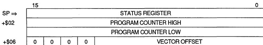
**Figure 6-3. Format \$0 — Four-Word Stack Frame**
