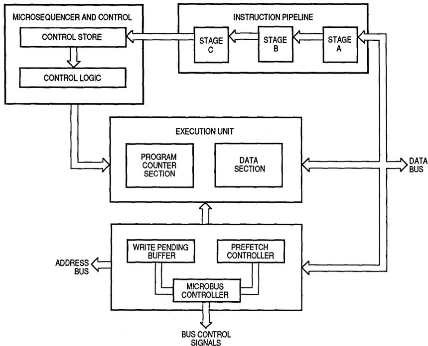
**Figure 8-1. Block Diagram of Independent Resources**
