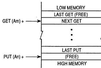
To implement a queue as a circular buffer, the relevant address register should be checked and (if necessary) adjusted before performing a "put" or "get"
