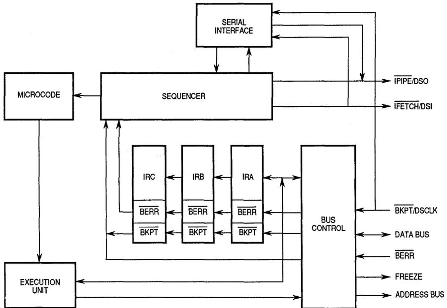
Figure 7-3. BDM Block Diagram
