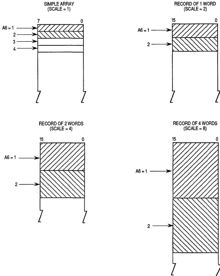
NOTE: Regardless of array structure, software increments index to point to next record.
