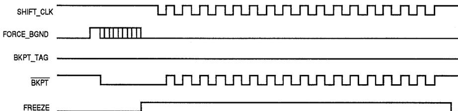
**Figure 7-8.  $\overline{\text{BKPT}}$  Timing for Forcing BDM**
