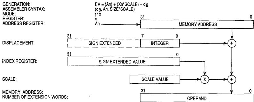
"Ri" specifies a general data or address register used as an index register. The index operand is derived from the index register. The index register is a data register if bit [15] = 0 in the first extension word and an address register if bit [15] = 1. The index register number is given by extension word bits [14:12].
