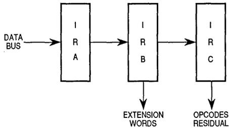
**Figure 7-11. Functional Model of Instruction Pipeline**
