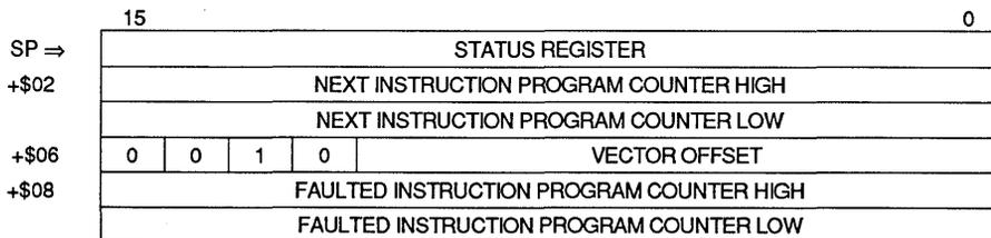
**Figure 6-4. Format \$2 — Six-Word Stack Frame**
