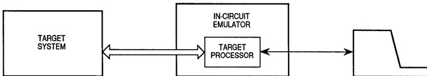
**Figure 7-1. In-Circuit Emulator Configuration**
