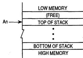
To implement stack growth from low to high memory, use  $(A_n) +$  to push data on the stack,  $-(A_n)$  to pull data from the stack.
