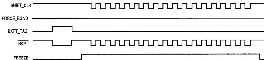
**Figure 7-7.  $\overline{\text{BKPT}}$  Timing for Single Bus Cycle**
