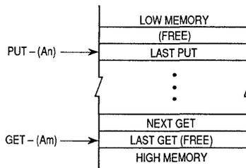
To implement the queue as a circular buffer, the "get" or "put" operation should be performed first, and then the relevant address register should be checked and (if necessary) adjusted. The address register is adjusted by adding the buffer length (in bytes) to the register contents.
