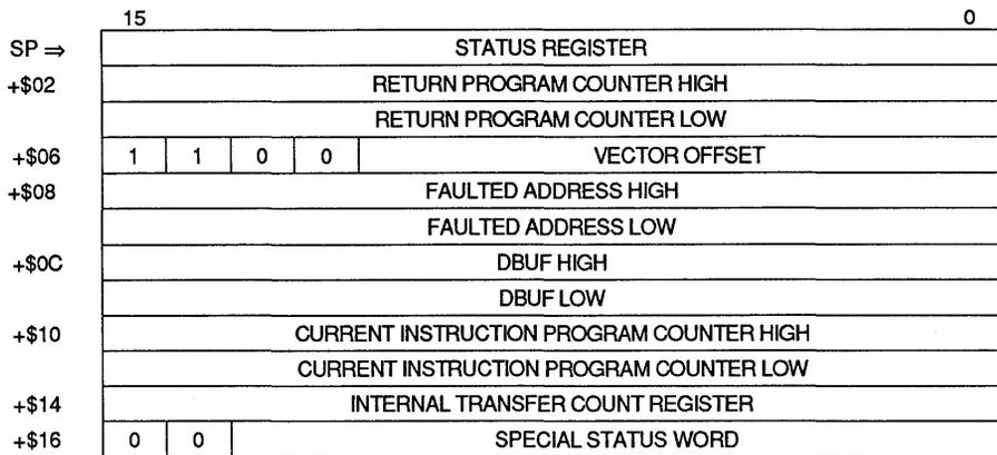
**Figure 6-6. Format \$C — BERR Stack for Prefetches and Operands**
