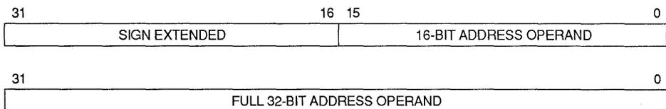
**Figure 2-5. Address Organization in Address Registers**
