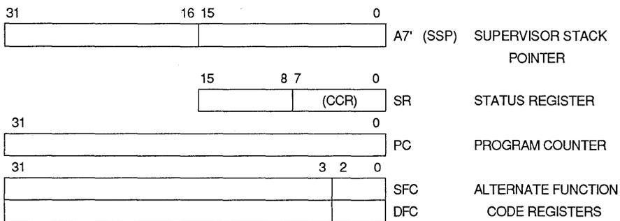
Figure 2-2. Supervisor Programming Model Supplement
