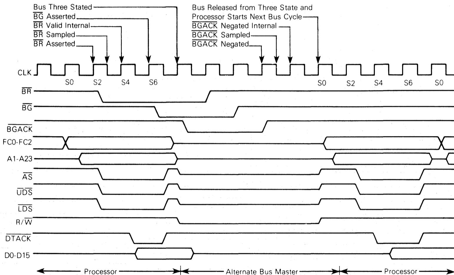
Figure 4-16. Bus Arbitration Timing Diagram — Processor Active
