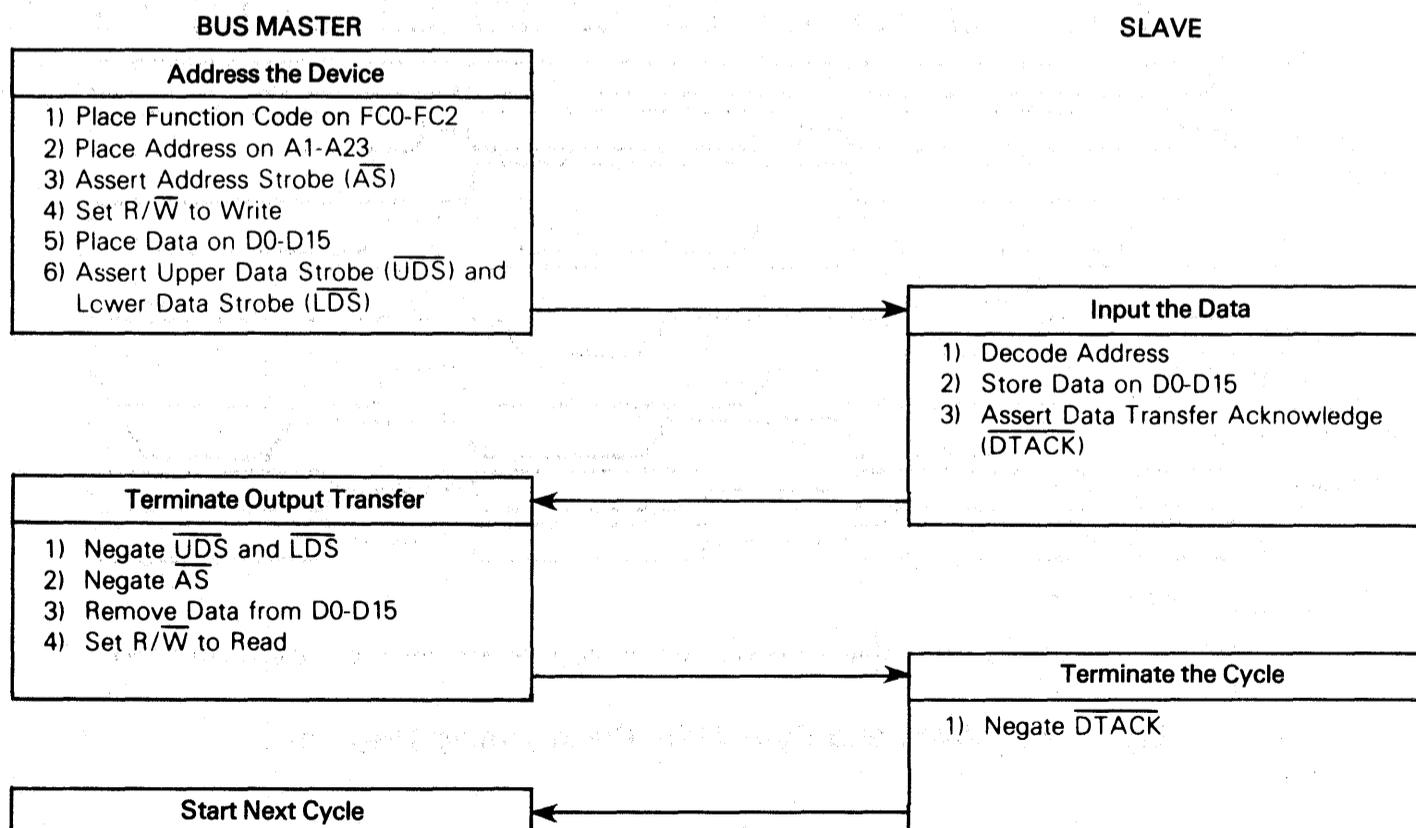
Figure 4-6. Word Write Cycle Flowchart
