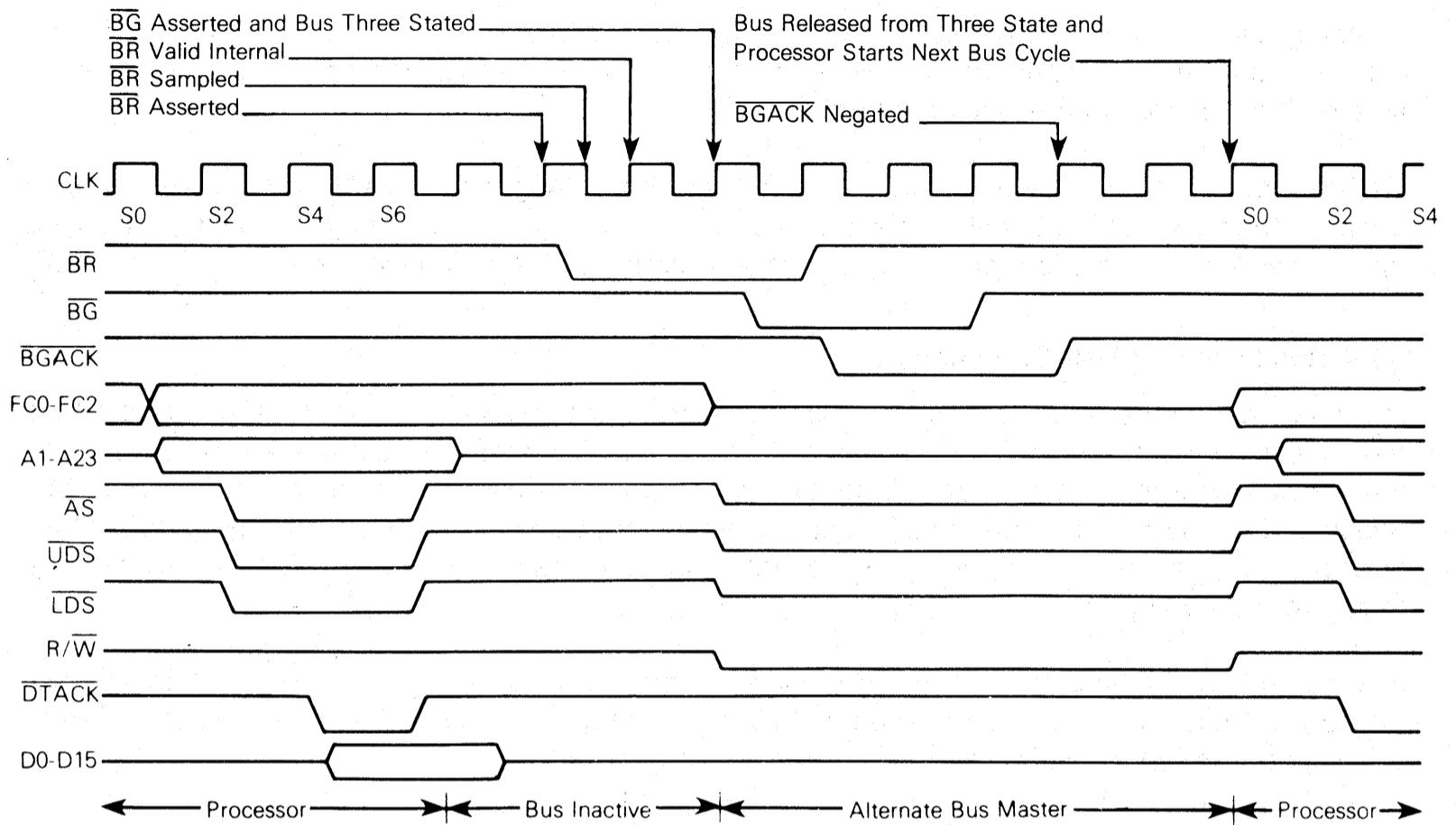
Figure 4-17. Bus Arbitration Timing Diagram — Bus Inactive
