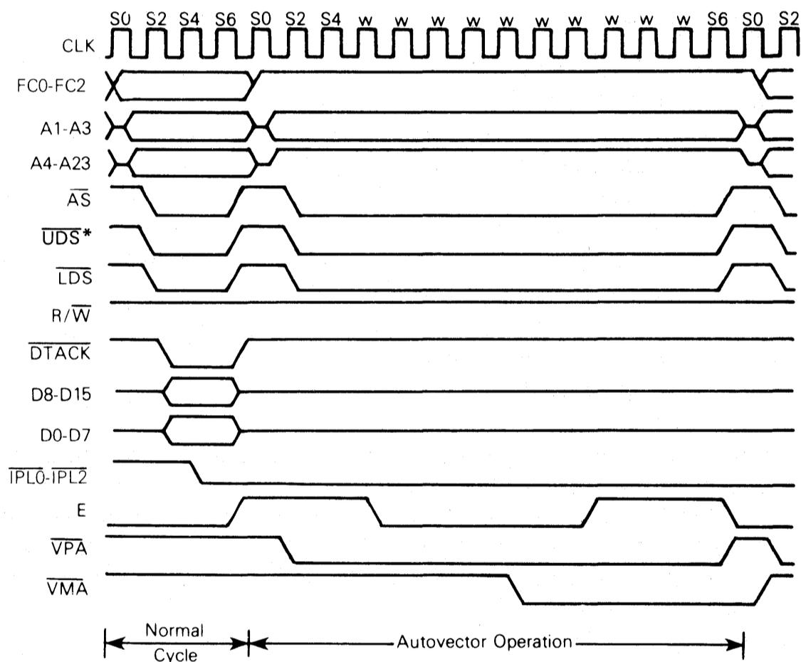
\* Although a vector number is one byte, both data strobes are asserted due to the microcode used for exception processing. The processor does not recognize anything on data lines D0 through D15 during autovector cycles.
