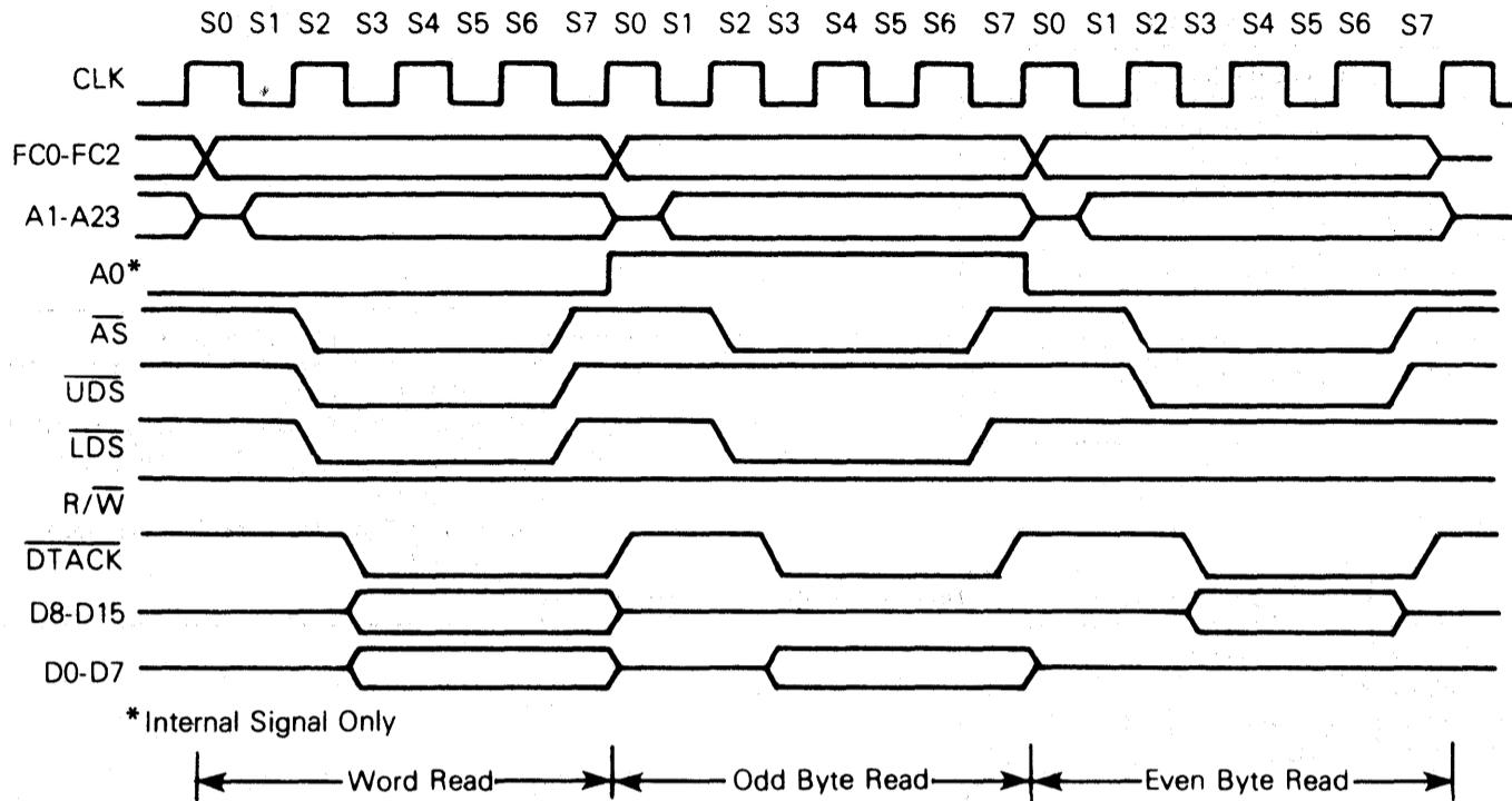
Figure 4-5. Word and Byte Read Cycle Timing Diagram
