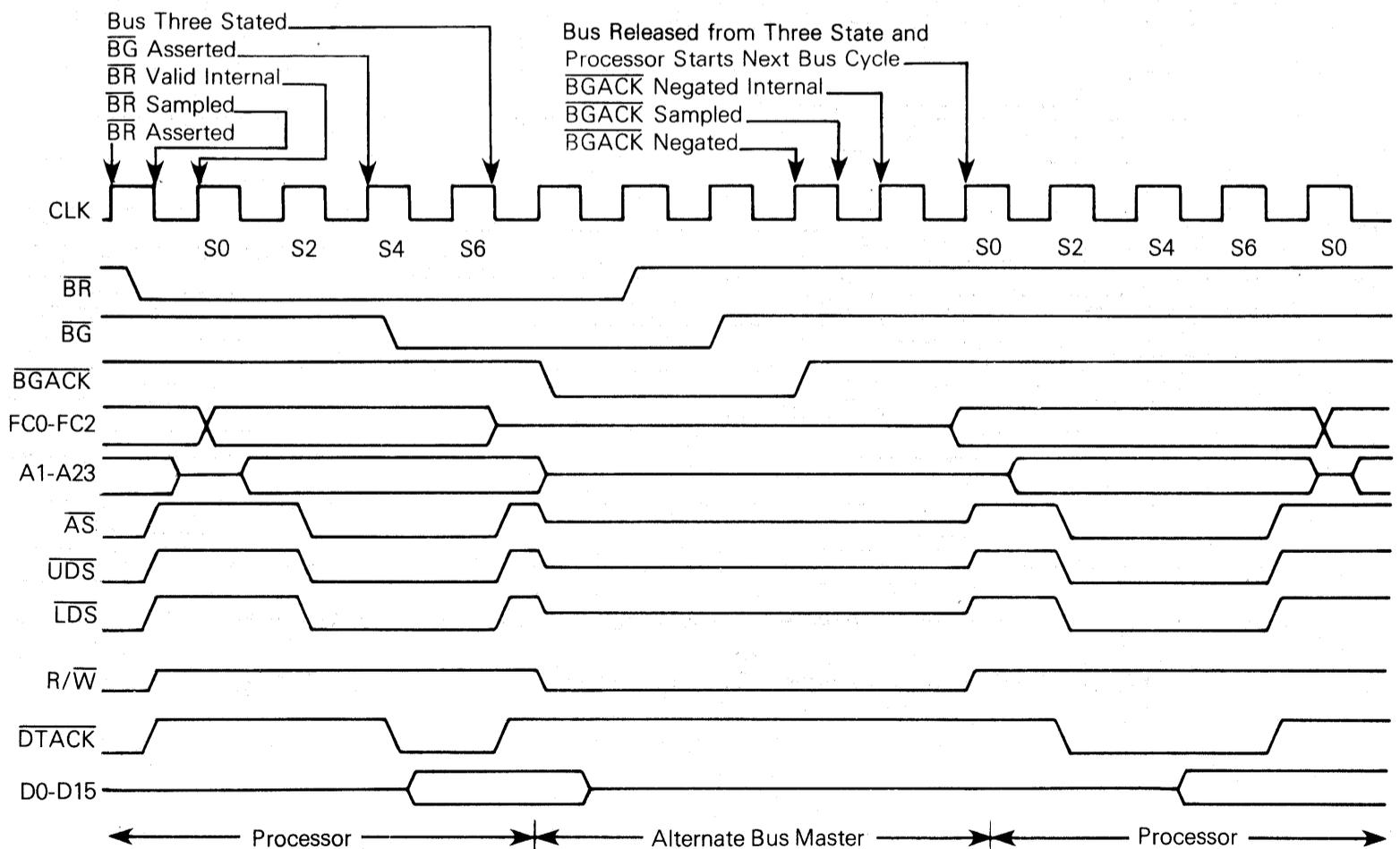
Figure 4-18. Bus Arbitration Timing Diagram — Special Case
