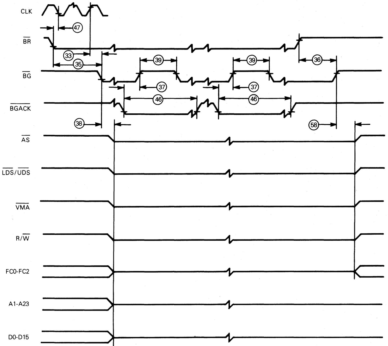
Figure 8-12. Bus Arbitration Timing — Multiple Bus Requests
