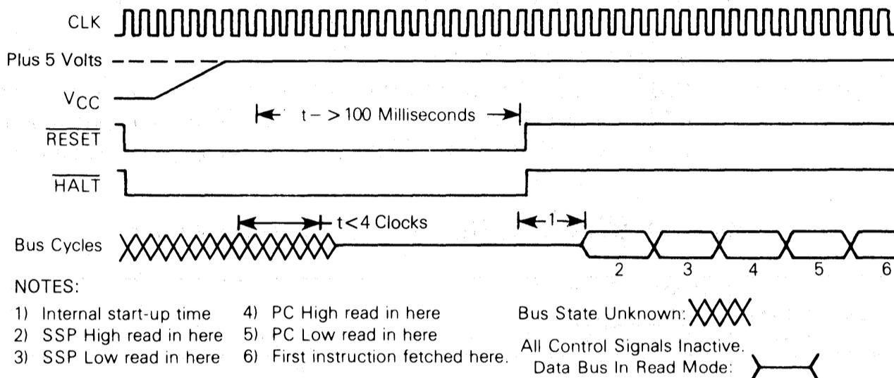
Figure 4-24. Reset Operation Timing Diagram
