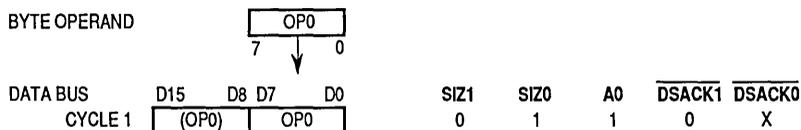
For a read operation, the slave responds by placing data on bits 7–0 of the data bus and asserting  $\overline{DSACK1}$  to indicate a 16-bit port. The MC68340 then reads the operand byte from bits 7–0 and ignores bits 15–8.
