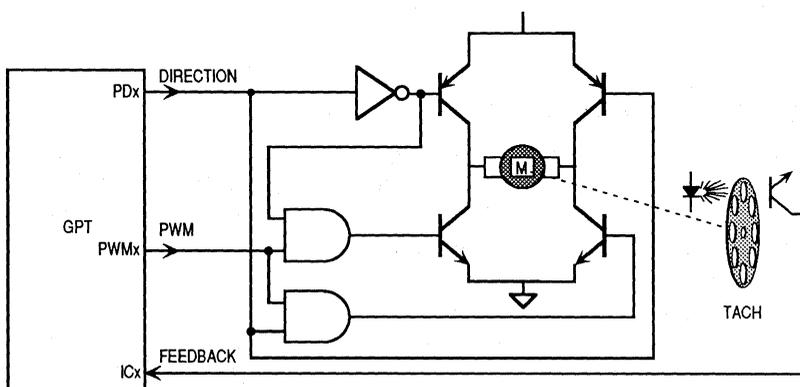
Figure 10-1. Motor Control Example
