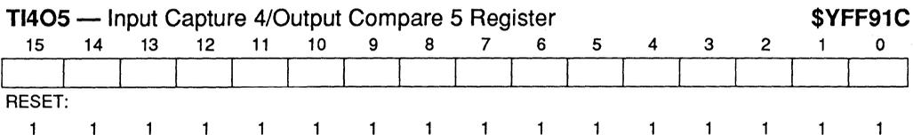
**Figure 3-4. Input Capture 4/Output Compare 5 Register (TI4O5)**
