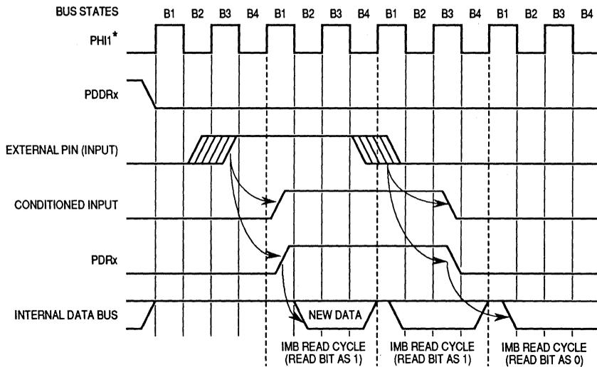
\*PH11 is the same frequency as the system clock; however, it does not have the same timing.
