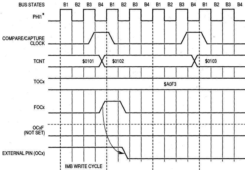
\*PHI1 is the same frequency as the system clock; however, it does not have the same timing.
