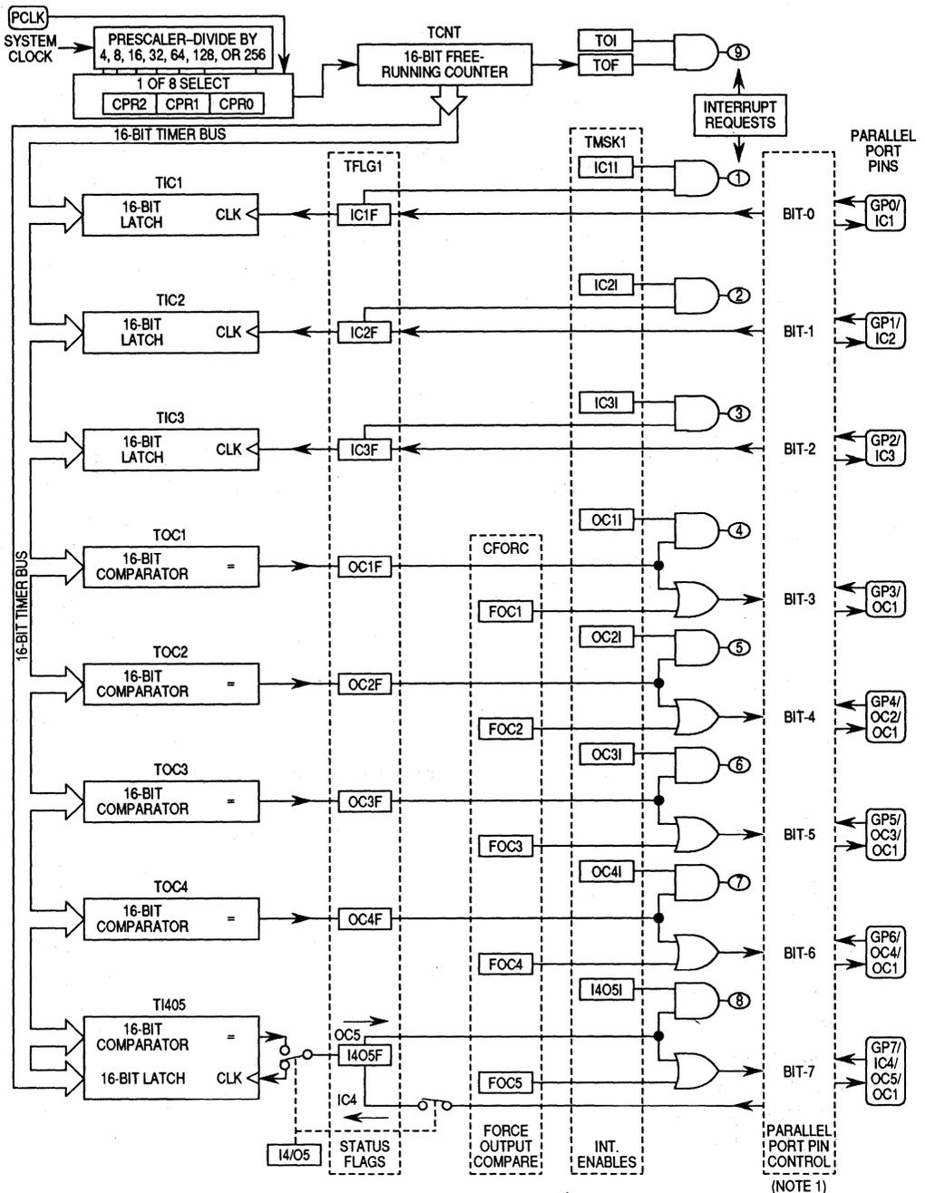
NOTE: Parallel port pin actions are controlled by DDR, OC1M, OC1D, and TCTL1 registers.
