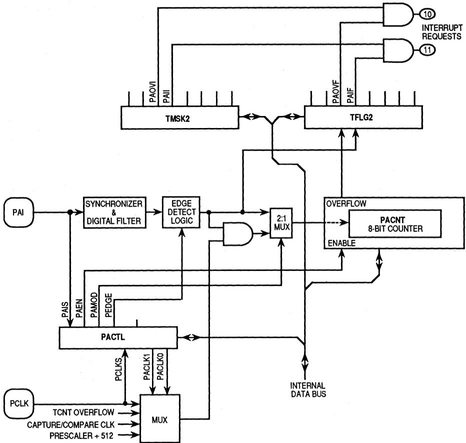
Figure 4-1. Pulse Accumulator Block Diagram
