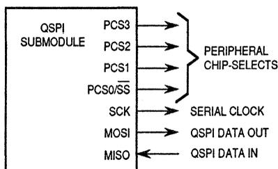
**Figure 2. Master Mode Representation of the QSPI**
