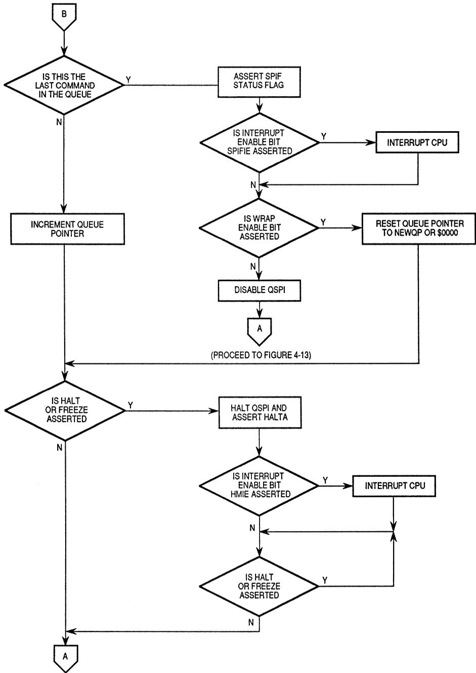
Figure 4-14. Flowchart of QSPI Slave Operation (Part 2)
