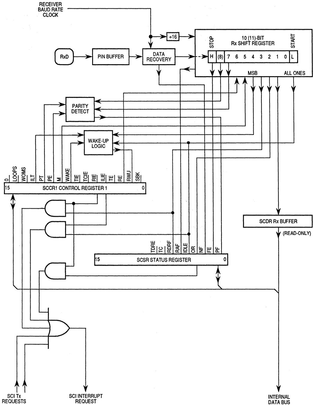
Figure 5-1. SCI Receiver Block Diagram
