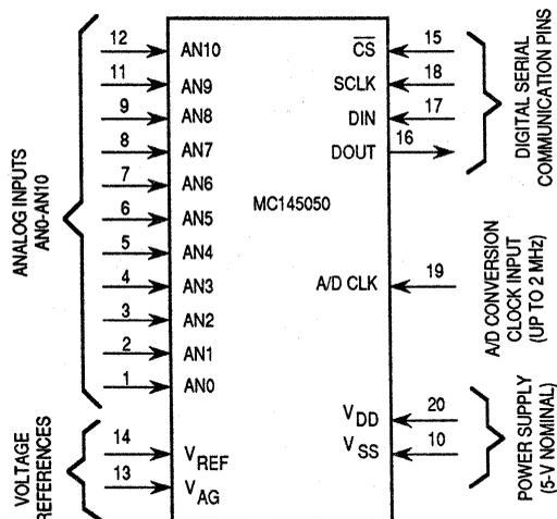
Figure 1. MC145050 Pinout
