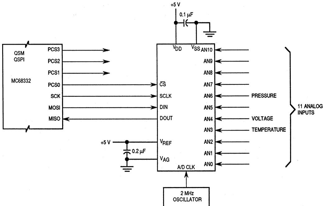
Figure 7. Basic Serial A/D Data Acquisition System
