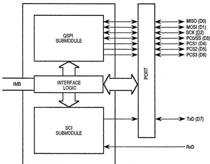
Figure 1-1. QSM Block Diagram
