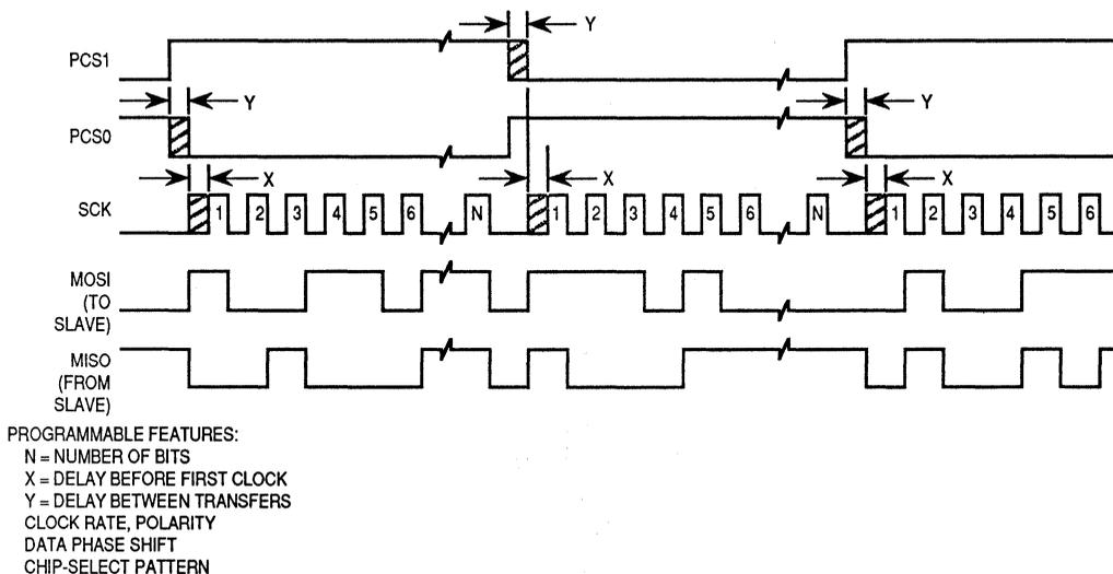
**Figure 5. Basic QSPI Master Mode Timing Diagram**
