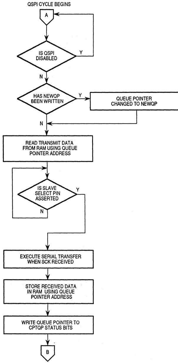
Figure 4-13. Flowchart of QSPI Slave Operation (Part 1)
