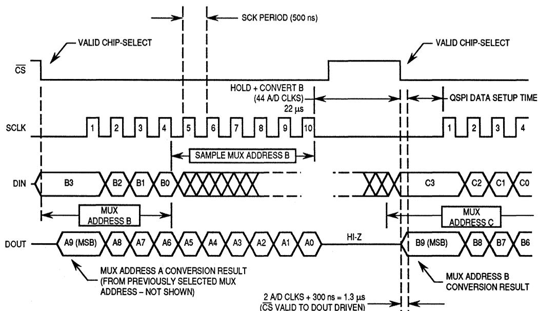
Figure 8. MC145050 Conversion and Transfer Timing
