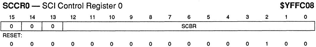
**Figure 5-3. SCI Control Register 0**
