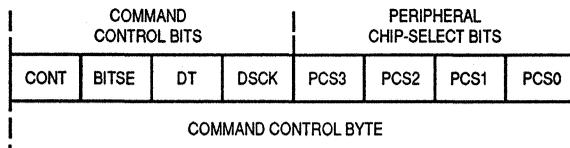
**Figure 4. Command Control Byte**
