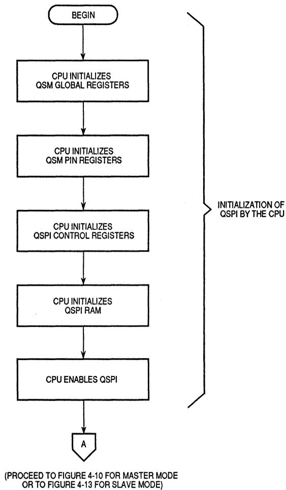
**Figure 4-9. Flowchart of QSPI Initialization Operation**
