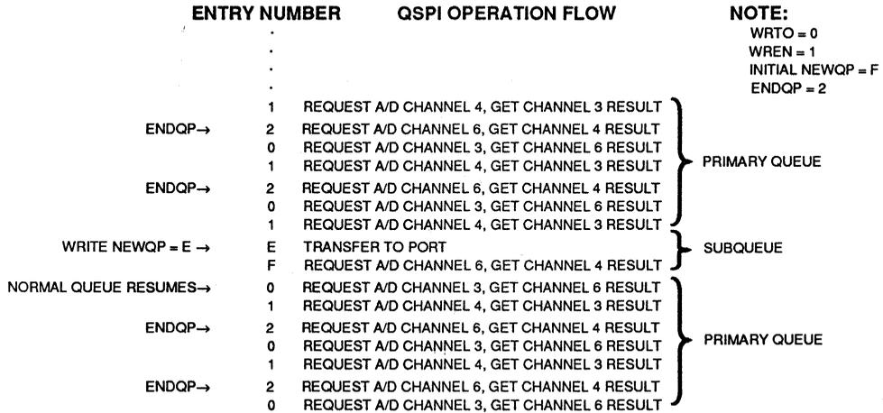
Figure 11. Example Subqueue Structure and Operation
