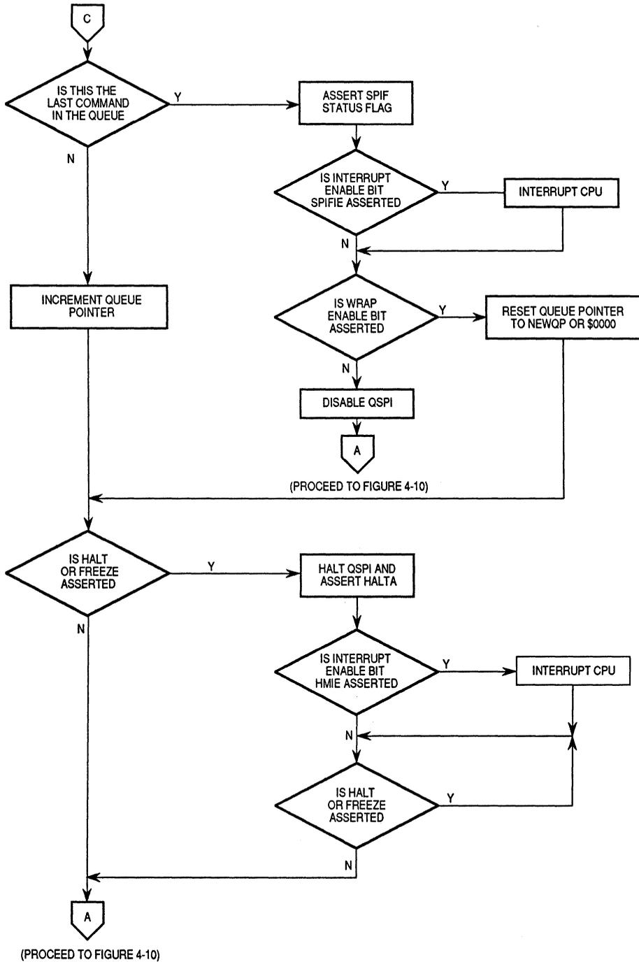
Figure 4-12. Flowchart of QSPI Master Operation (Part 3)
