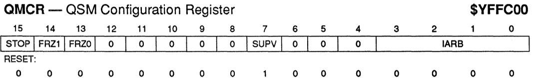
**Figure 3-1. QSM Configuration Register**
