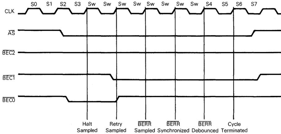
Figure 4-13.  $\overline{\text{BEC}}$  Debouncer Timing Diagram
