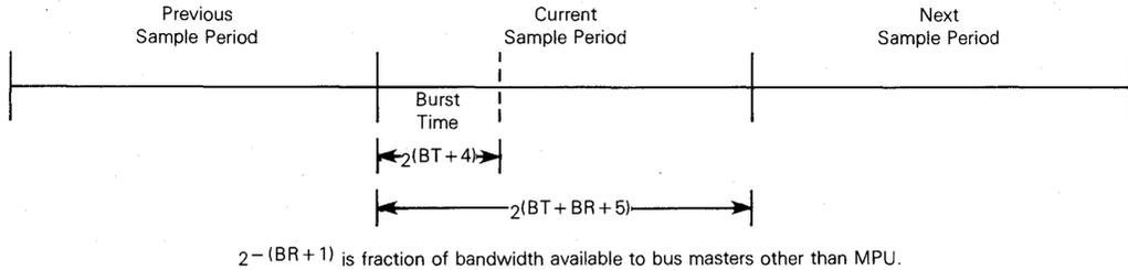
**Figure 5-2. Limited Rate Auto Request Operation Timing Parameter Relationships**
