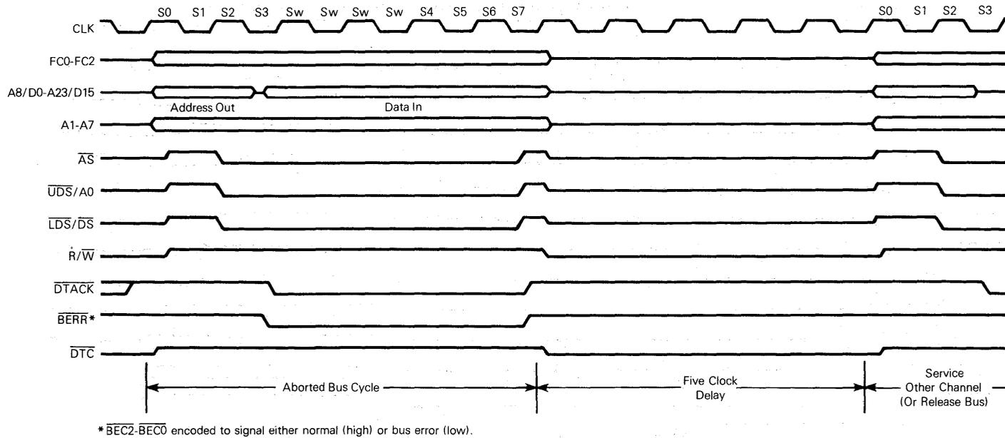
Figure 4-15. Bus Error Operation Timing Diagram
