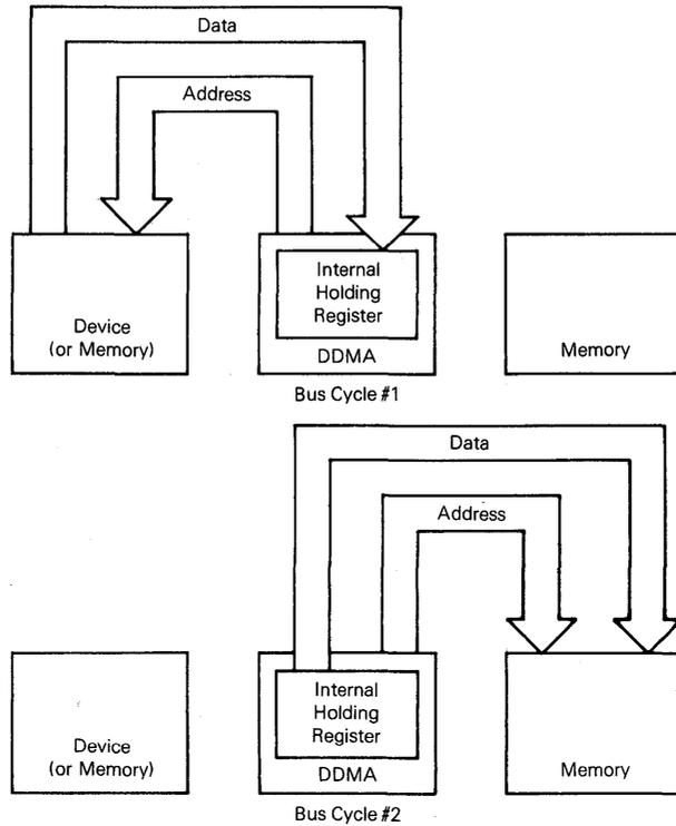
**Figure 1-4. Dual-Address Transfer Sequence**
