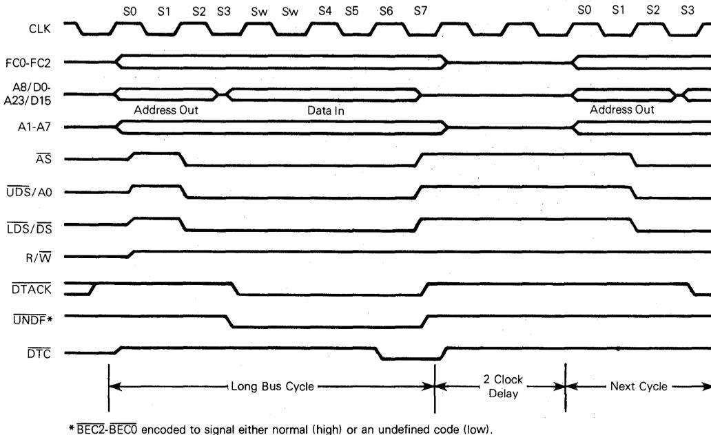
**Figure 4-18. Undefined BEC Operation Timing Diagram**
