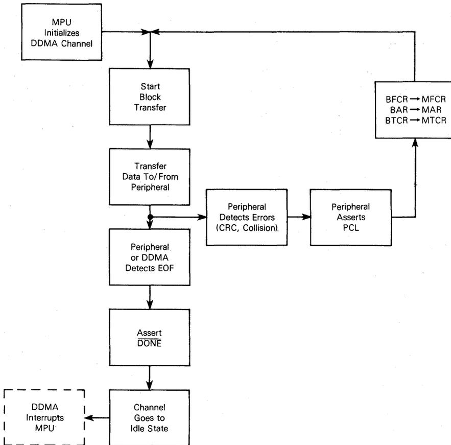
Figure 5-4. Reload Operation Flowchart
