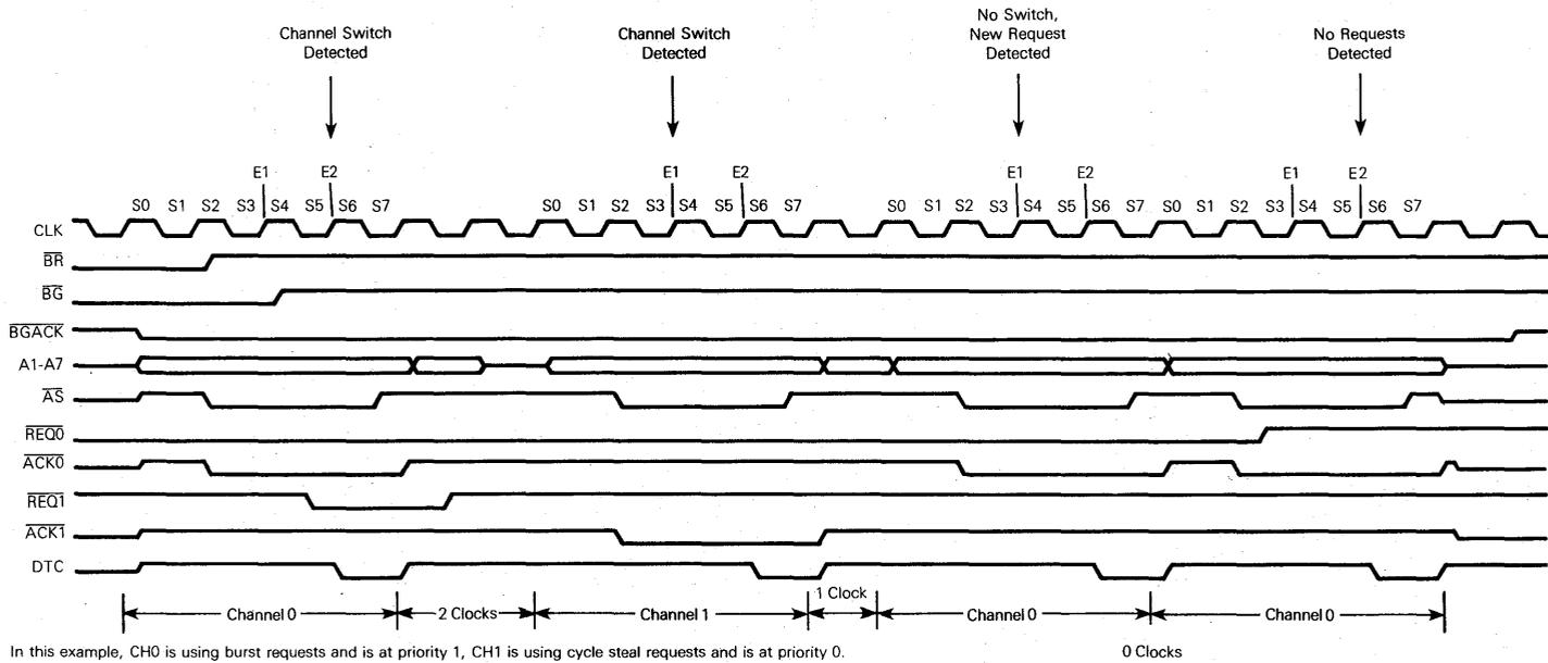
Figure 4-21. Inter-Cycle Overhead Timing Diagram
