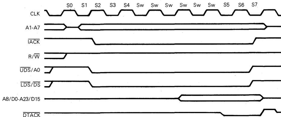
Figure 4-5. Interrupt Acknowledge Cycle Timing Diagram
