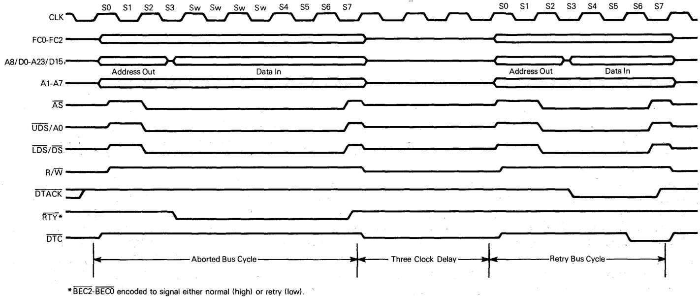
Figure 4-16. Retry Operation Timing Diagram
