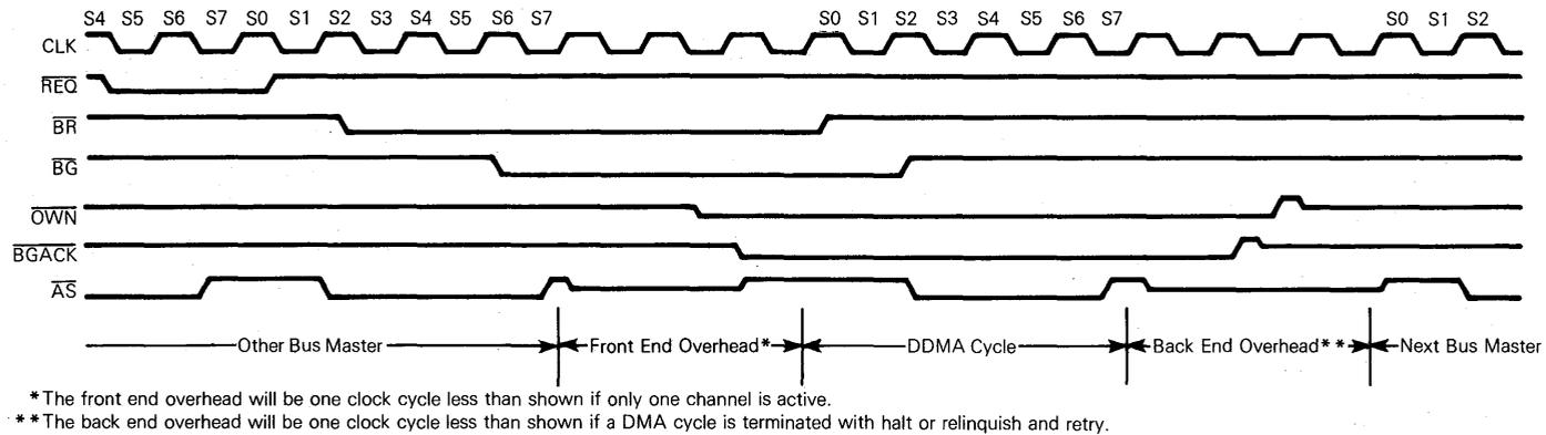
Figure 4-20. Bus Arbitration Timing Diagram
