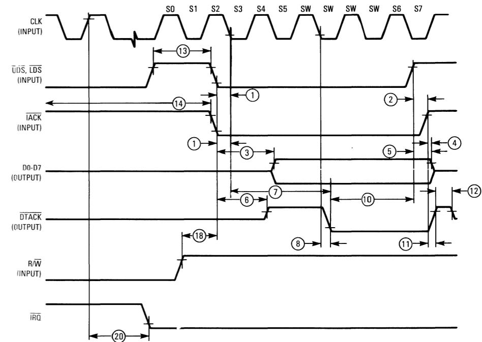
Figure 10-3. Interrupt Acknowledge Cycle Timing Diagram
