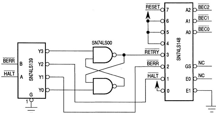
**Figure 8-6. Example  $\overline{\text{BEC}}$  Signal Generation Circuit**
