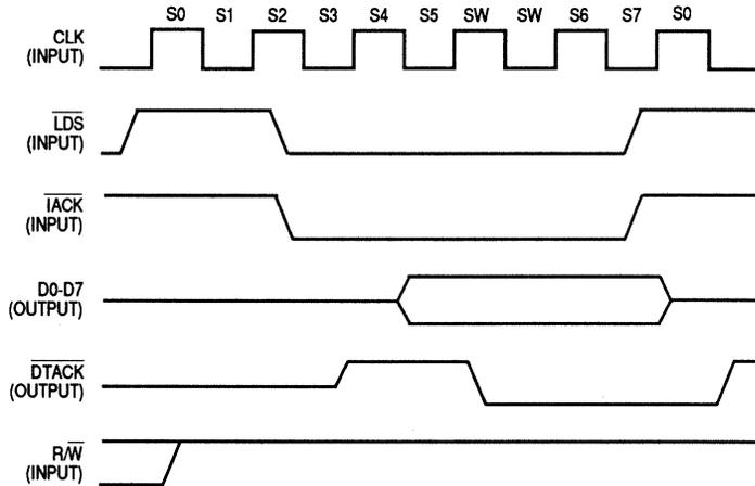
Figure 8-3. Interrupt Acknowledge Cycle
