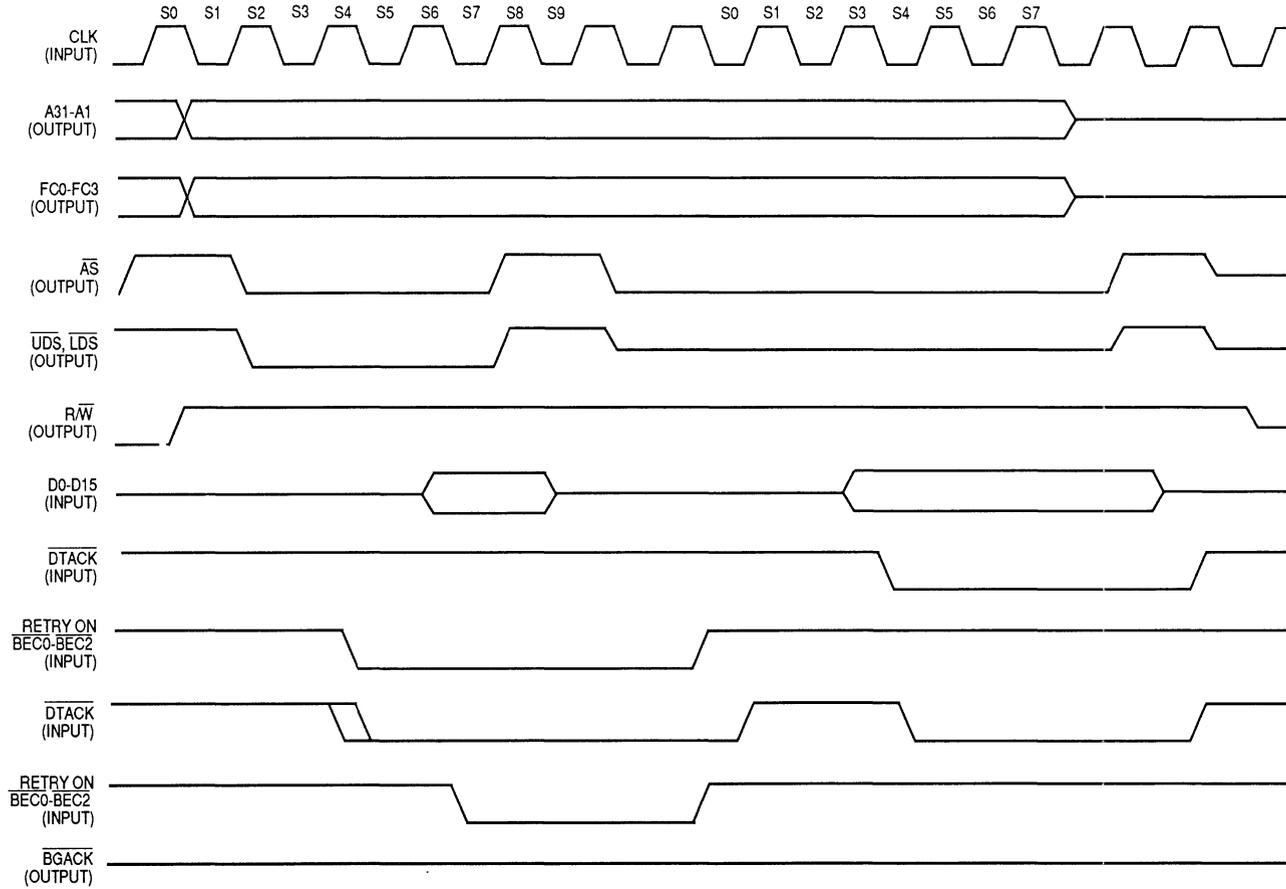
NOTE: Two alternatives of  $\overline{DTACK}$  and retry are drawn in the first one. The second cycle is postponed for one additional cycle due to  $\overline{BEC}$  synchronization.
