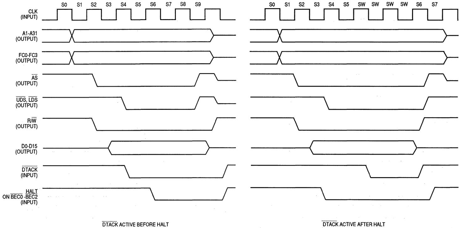
Figure 8-7. Write Cycle with Halt
