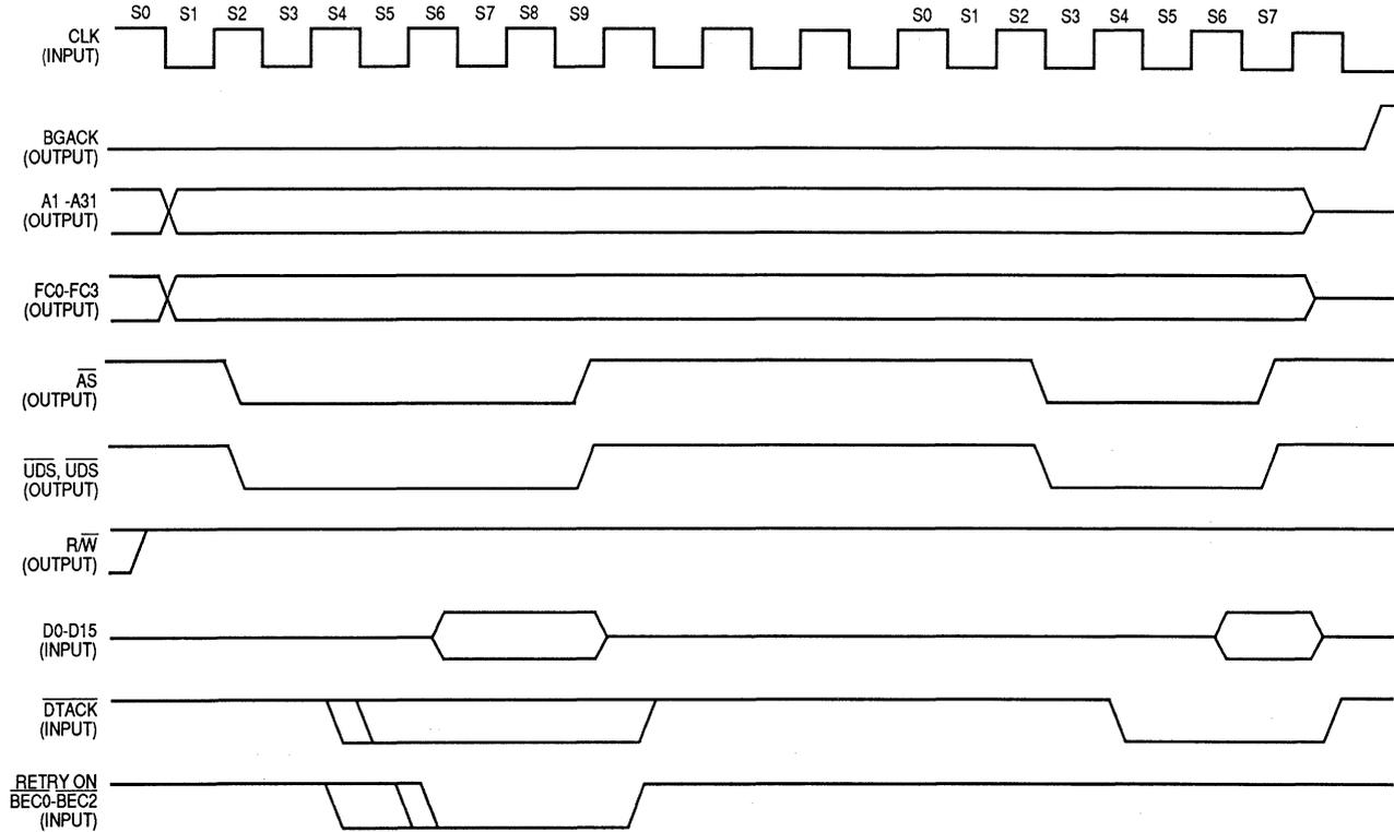
Figure 8-10. Read Cycle with Retry
