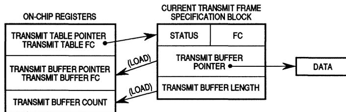
Figure 4-2. Transmit Registers
