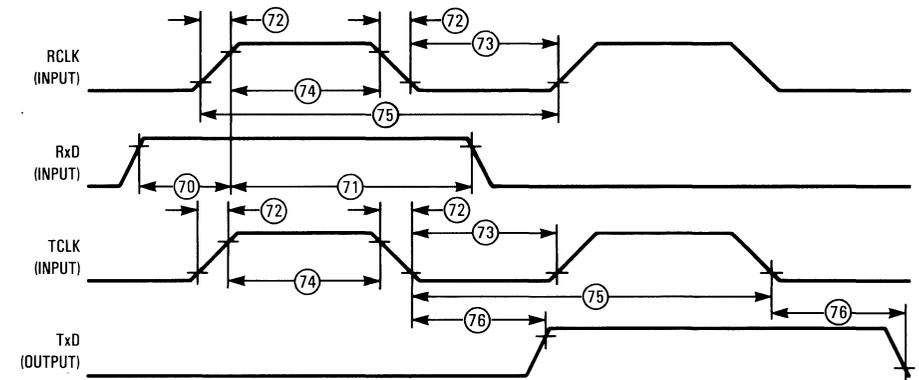
Figure 10-12. XPC Serial Data RxD, TxD, and Serial Clocks (RCLK, TCLK) Timing Diagram
