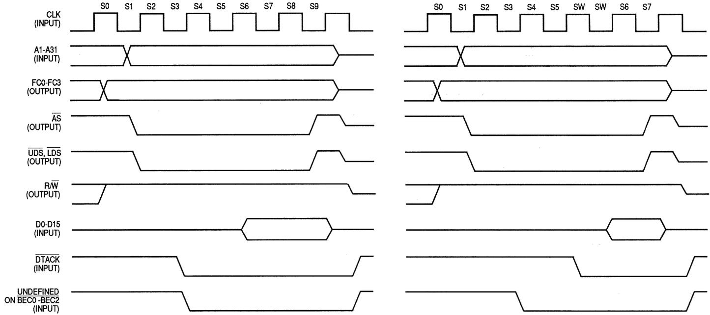
Figure 8-12. Read Cycle with Undefined  $\overline{BEC0}$ - $\overline{BEC2}$
