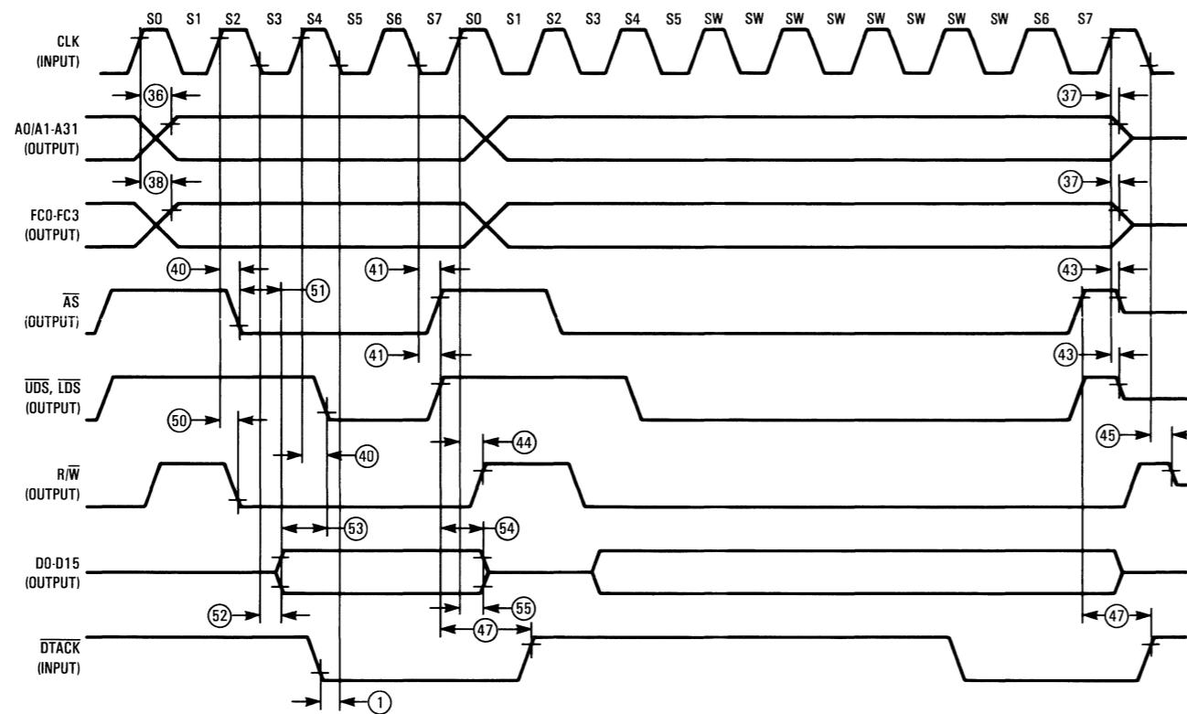
Figure 10-6. Write Cycle Timing Diagram
