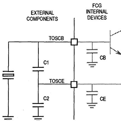
Figure 3-5. Transmitter Crystal Oscillator
