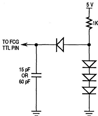
Figure 5-1. TTL Test Load
