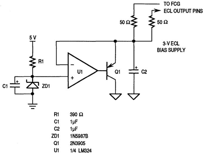
Figure 5-5. ECL Test Load
