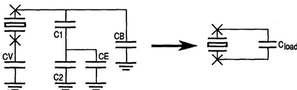
Figure 3-4. Load Capacitance Model
