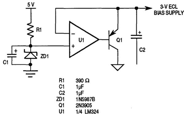
**Figure 4-5. Discrete Bias Supply Generator**
