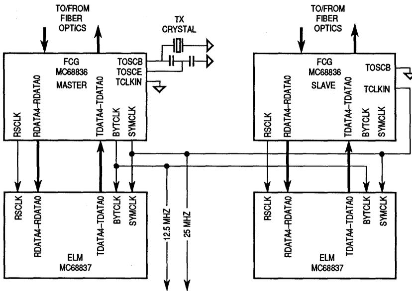
Figure 4-1. Dual Attached Station
