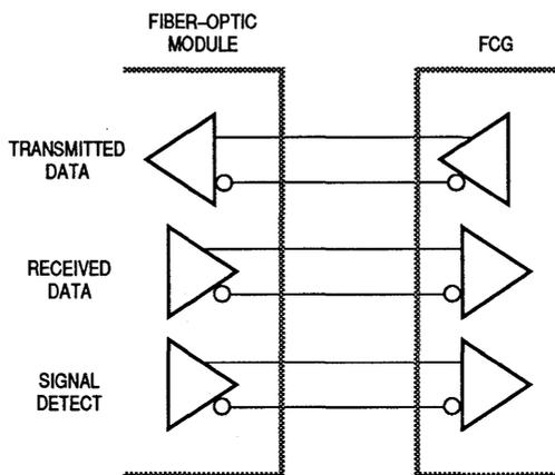
**Figure 4-2. Differential Raised ECL Interface**
