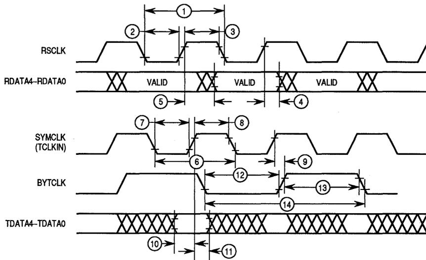
Figure 5-2. Parallel Interface Timing
