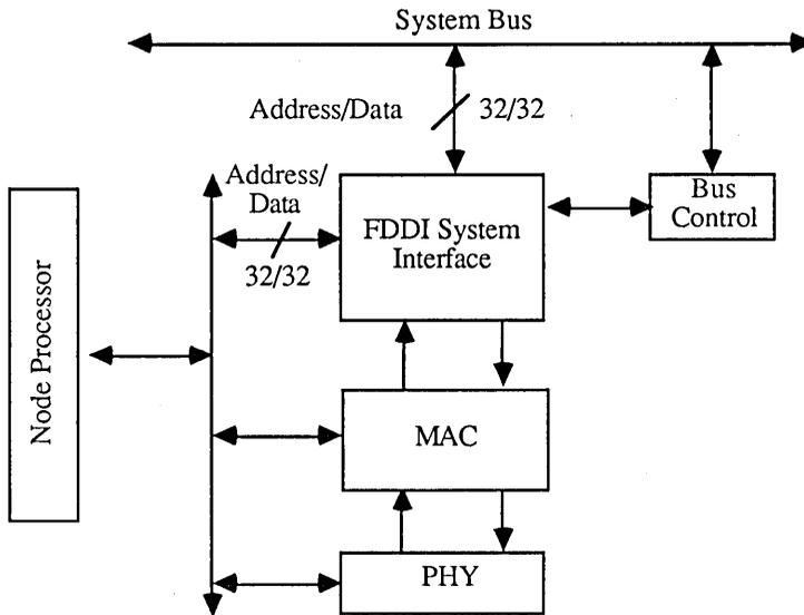
**Figure B-2. Basic Configuration With Separate Node Processor**
