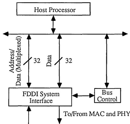
**Figure B-6. 64-Bit Data With FSI DMA**
