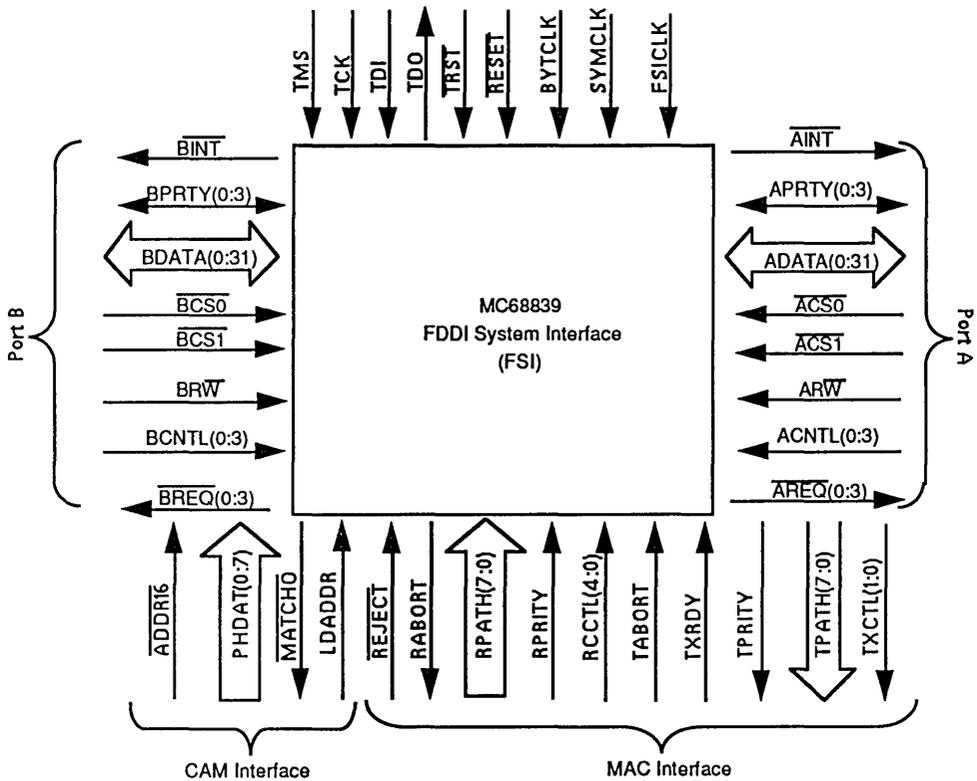
Figure 4-1. FSI Pinout
