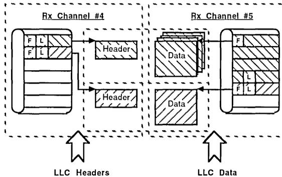
**Figure 6-23. Header Splitting**
