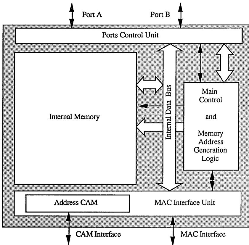
Figure 2-1. Internal Architecture
