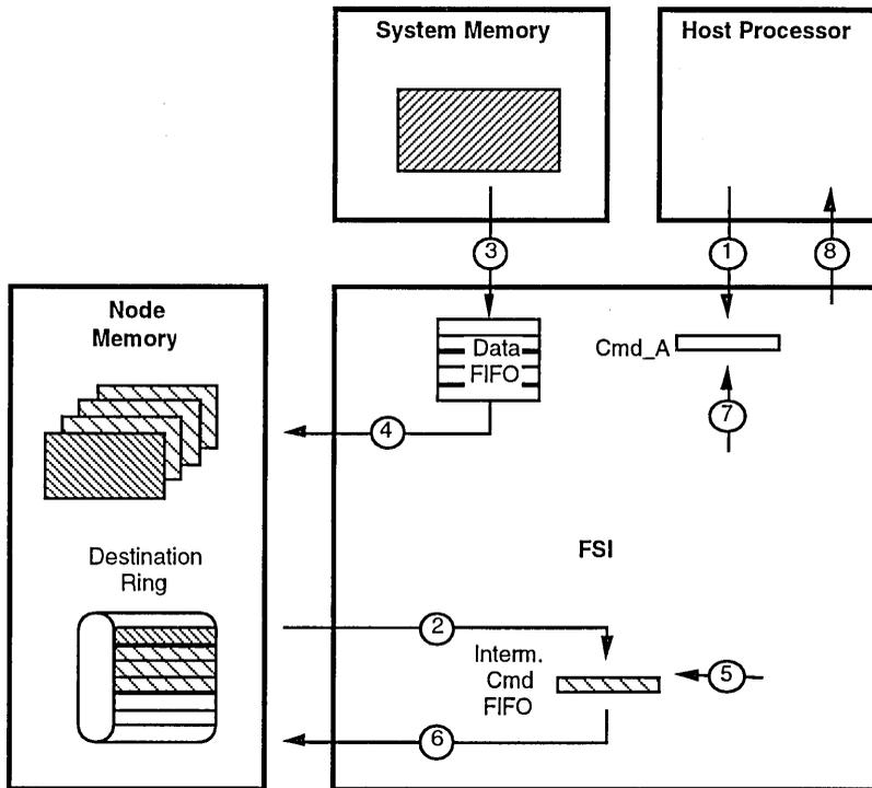
Figure 6-22. DMA Transfers Using Command Register
