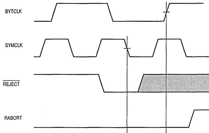
Figure 10-6. FSI REJECT/RABORT Timing
