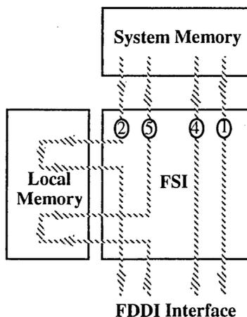
**Figure 6-3. Direct and Expanded Local Memory Options**
