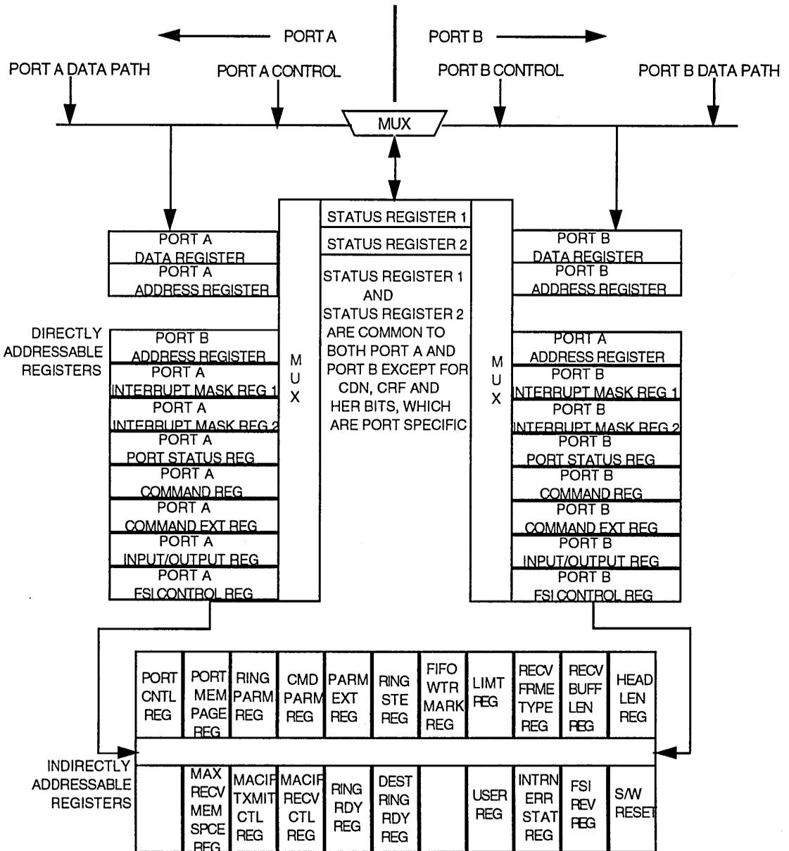
Figure 3-1. Internal and Common Registers
