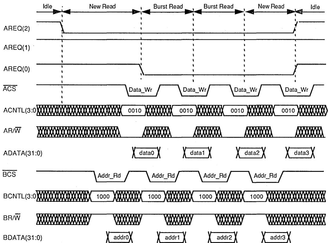
**Figure 8-4. Non-Multiplexed Address/Data Operation**
