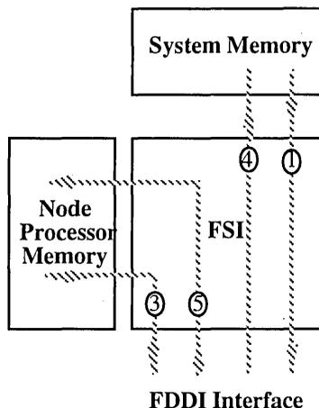
Figure 6-1. Direct Transmission and Reception
