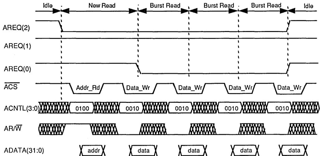
**Figure 8-3. Address/Data Multiplexed Operation**
