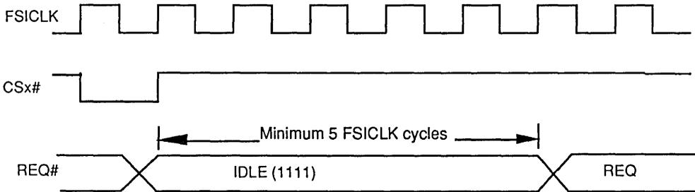
**Figure 8-8. Request Negation to Request Assertion in Asynchronous Mode**
