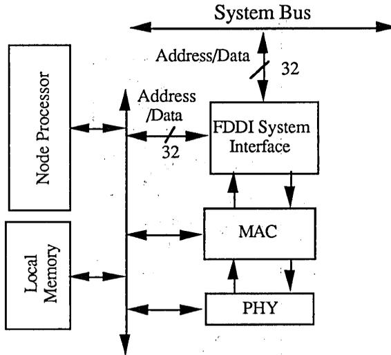
**Figure B-4. Local Memory with Separate Node Processor**
