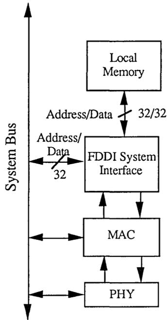
**Figure B3. Basic Configuration with Local Memory**
