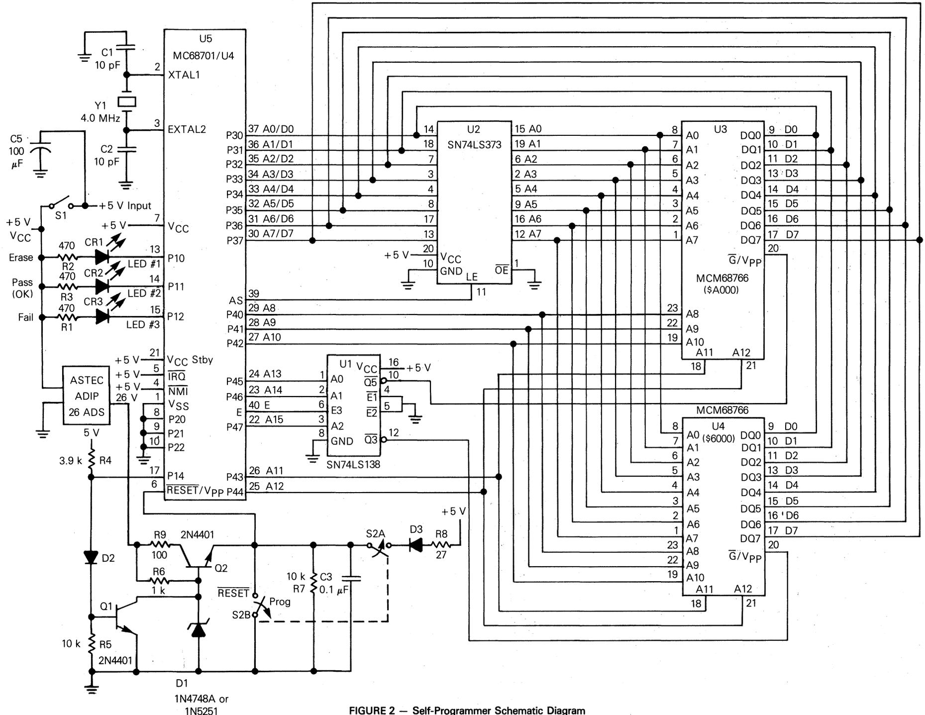
FIGURE 2 — Self-Programmer Schematic Diagram
