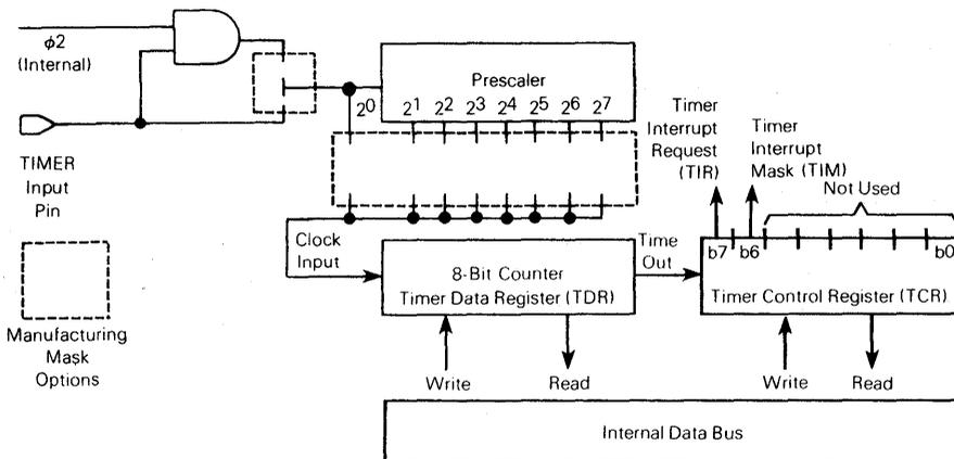
Figure 5-1. MC6805P2/P4/P6 Timer Block Diagram
