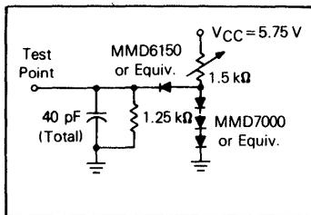
Figure 11-1. TTL Equivalent Test Load
