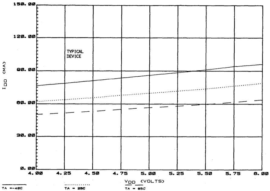
Figure 11-14.  $V_{DD}$  vs  $I_{DD}$  (Variation with Temperature)
