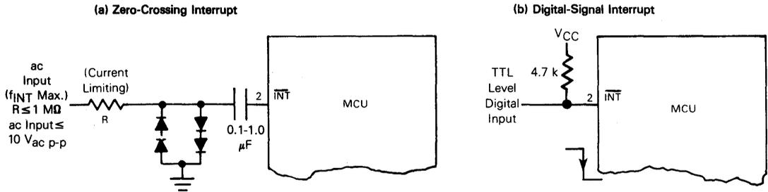
Figure 7-9. Typical Interrupt Circuits
