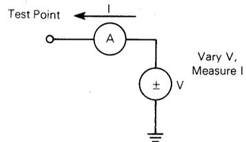
Figure 11-18. I/O Characteristic Measurement Circuit
