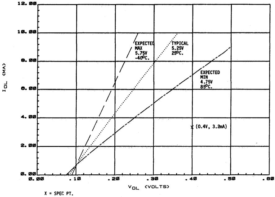
Figure 11-7. Port B  $V_{OL}$  vs  $I_{OL}$
