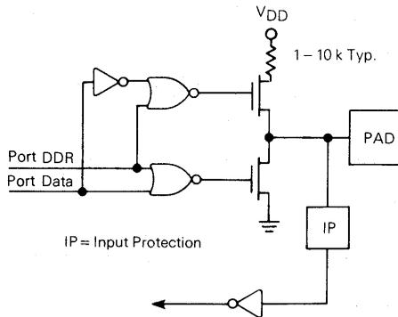
Figure 11-16. Port B Logic Diagram
