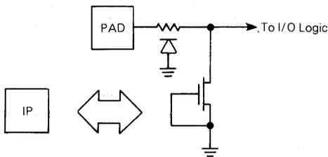
Figure 11-17. Typical Input Protection
