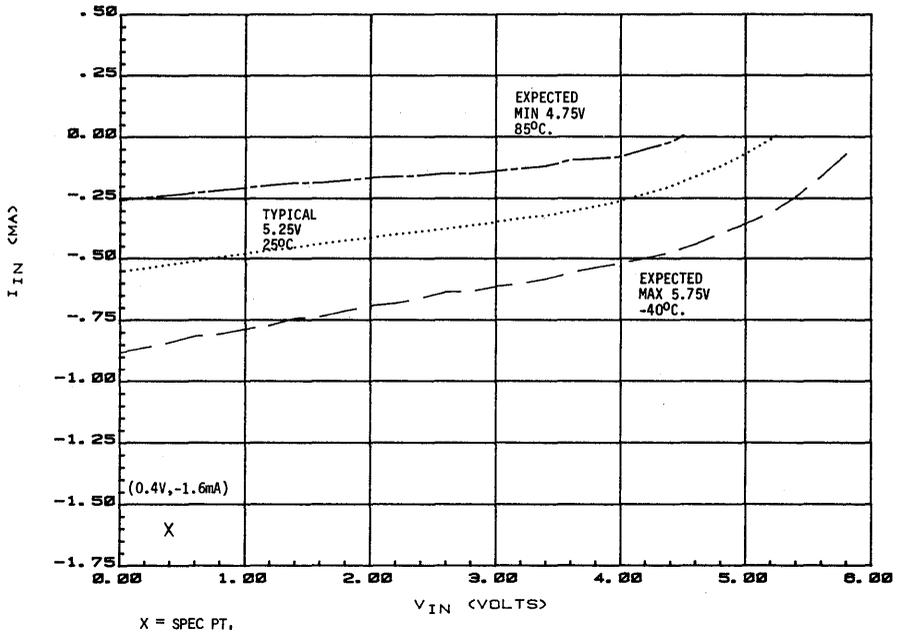
Figure 11-11. EXTAL  $V_{in}$  vs  $I_{in}$
