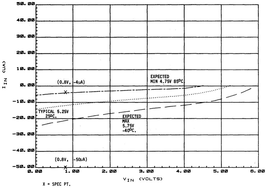
Figure 11-13. RESET  $V_{in}$  vs  $V_{in}$
