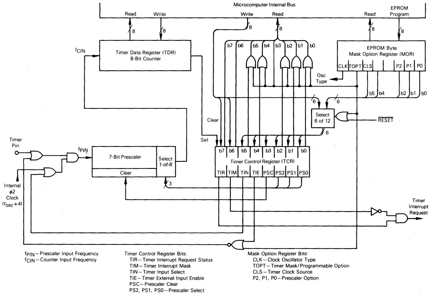
NOTE: The TOPT bit in the Mask Option Register selects whether the timer is software programmable via the Timer Control Register or emulates the mask programmable parts via the MOR PROM byte.
