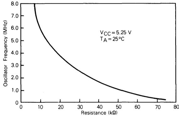
Figure 7-5. Typical Frequency Selection for Resistor Oscillator Option
