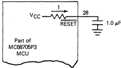
Figure 7-3. Power-Up  $\overline{\text{RESET}}$  Delay Circuit
