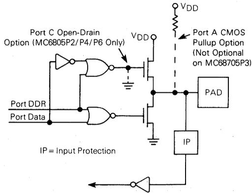
Figure 11-15. Ports A and C Logic Diagram
