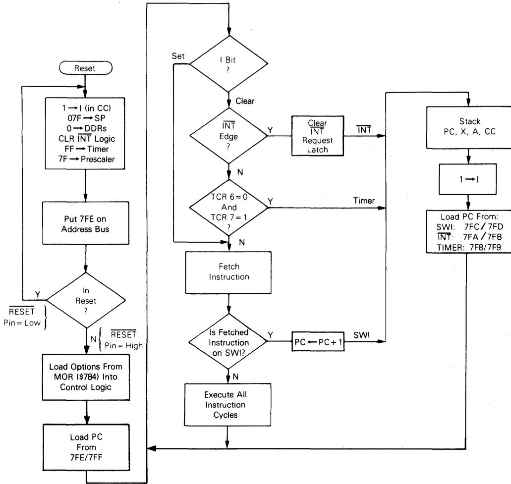
Figure 7-8. Reset and Interrupt Processing Flowchart for MC68705P3
