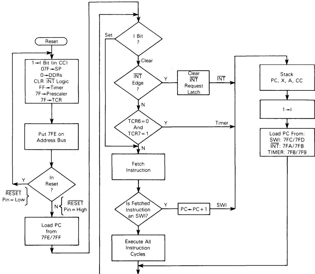
Figure 7-7. Reset and Interrupt Processing Flowchart for MC6805P2/P4/P6
