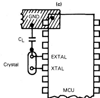
NOTE: Keep crystal leads and circuit connections as short as possible.
