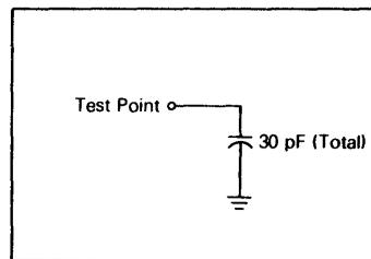
Figure 11-2. CMOS Equivalent Test Load
