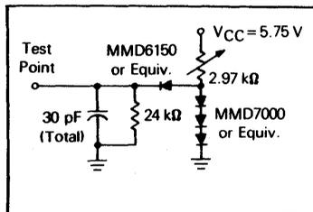
Figure 11-3. TTL Equivalent Test Load
