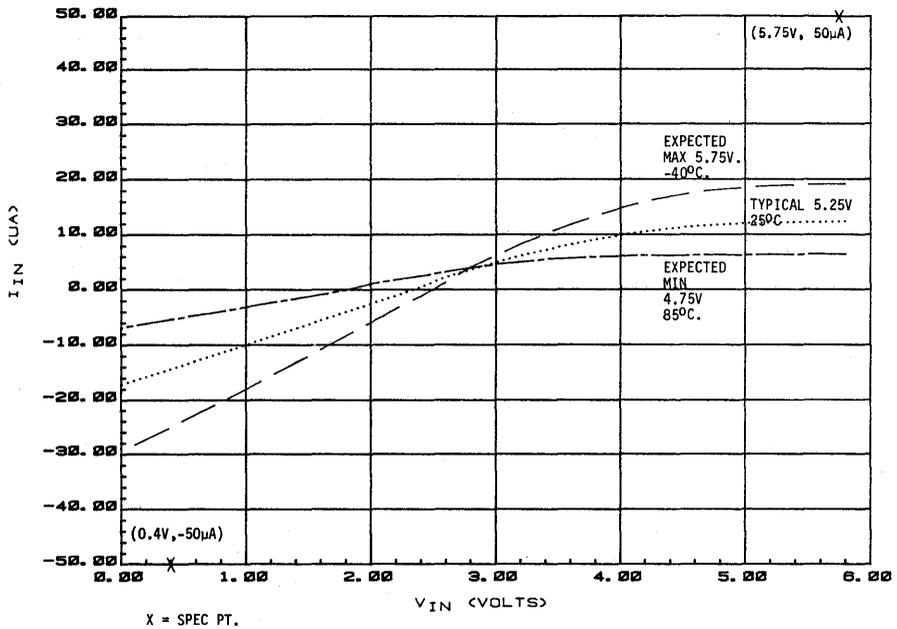
Figure 11-12. Interrupt  $V_{in}$  vs  $I_{in}$
