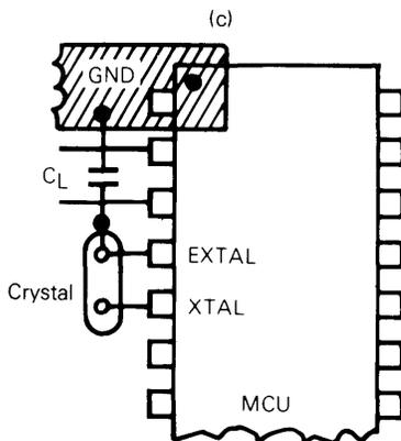
NOTE: Keep crystal leads and circuit connections as short as possible.
