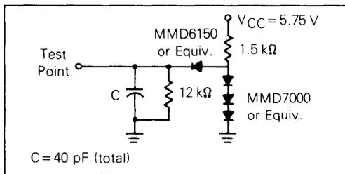
**FIGURE 2 — CMOS EQUIVALENT TEST LOAD (PORT A)**
