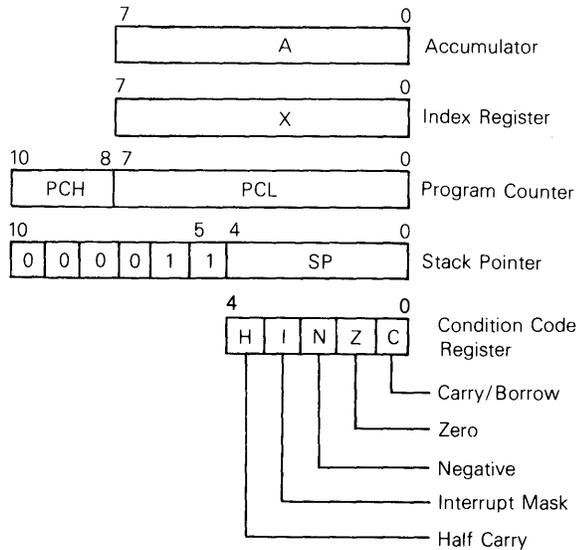
**ACCUMULATOR (A)** — The accumulator is a general purpose 8-bit register used to hold operands and results of the arithmetic calculations or data manipulations.
