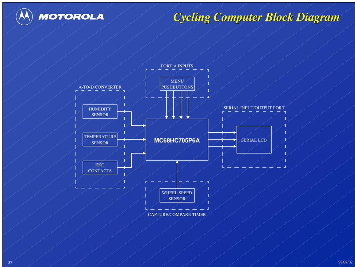
For riders to find the cycling computer useful, it must collect and present its statistics with a minimum of fuss. Ambient temperature and humidity are easily monitored with sensors attached to the cycling computer's housing, but the rider's heart rate presents a special problem.
