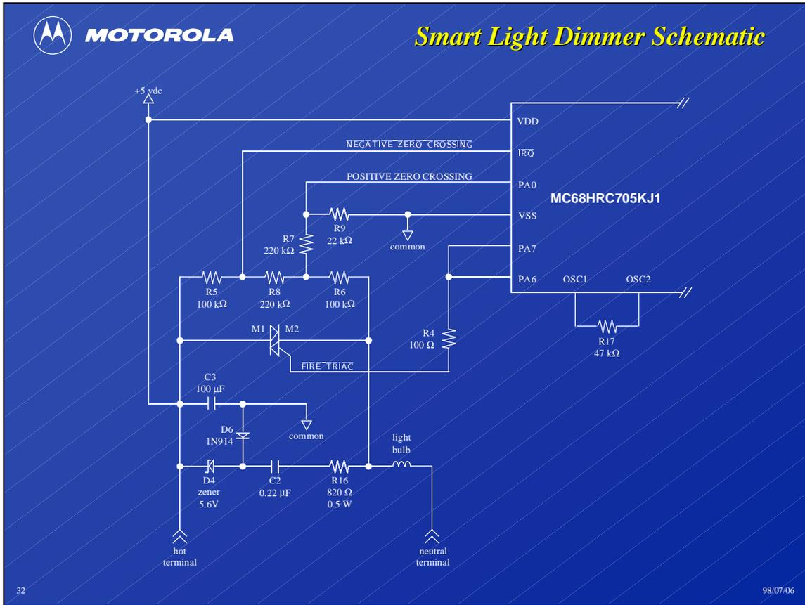
All 68HC05 devices have some number of pins, either dedicated or shared with other peripherals, that can be used as digital inputs and outputs. The partial circuit for the smart light dimmer, shown above, illustrates two useful features available on the I/O pins of the MC68HRC705KJ1.
