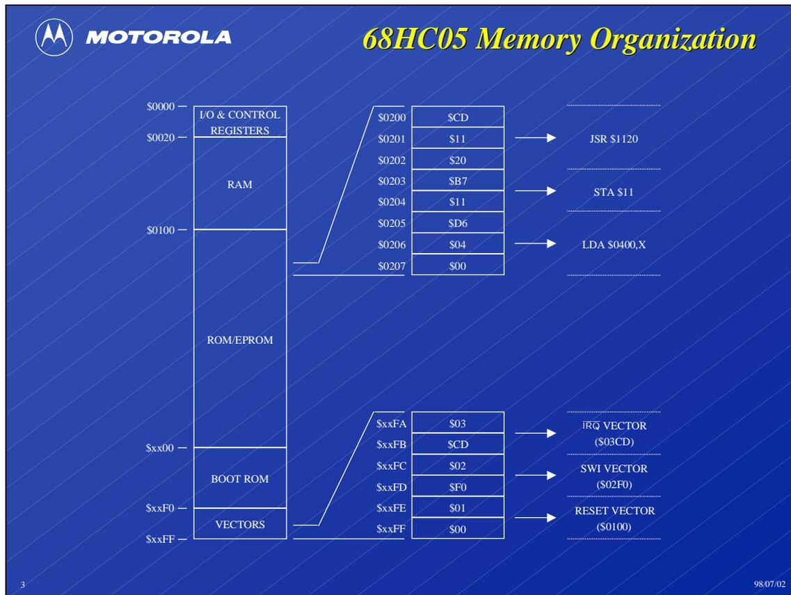
The 68HC05 is a Von Neumann computer. All storage and input/output resources are memory mapped into a single linear address space.
