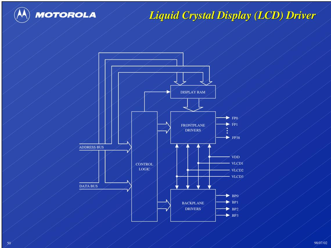
All 68HC05 “L” family members have liquid crystal display (LCD) interfaces of varying degrees of sophistication. A representative implementation is the LCD driver on the popular MC68HC705L16, shown in the block diagram above.
