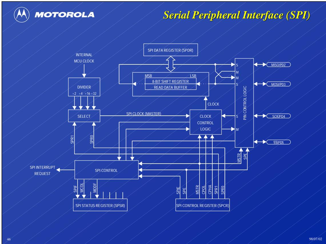
The serial peripheral interface (SPI) is the full-duplex, synchronous data transfer mechanism upon which the simpler serial input/output port (SIOP) is based. Differences between the SIOP and the SPI are discussed below.
