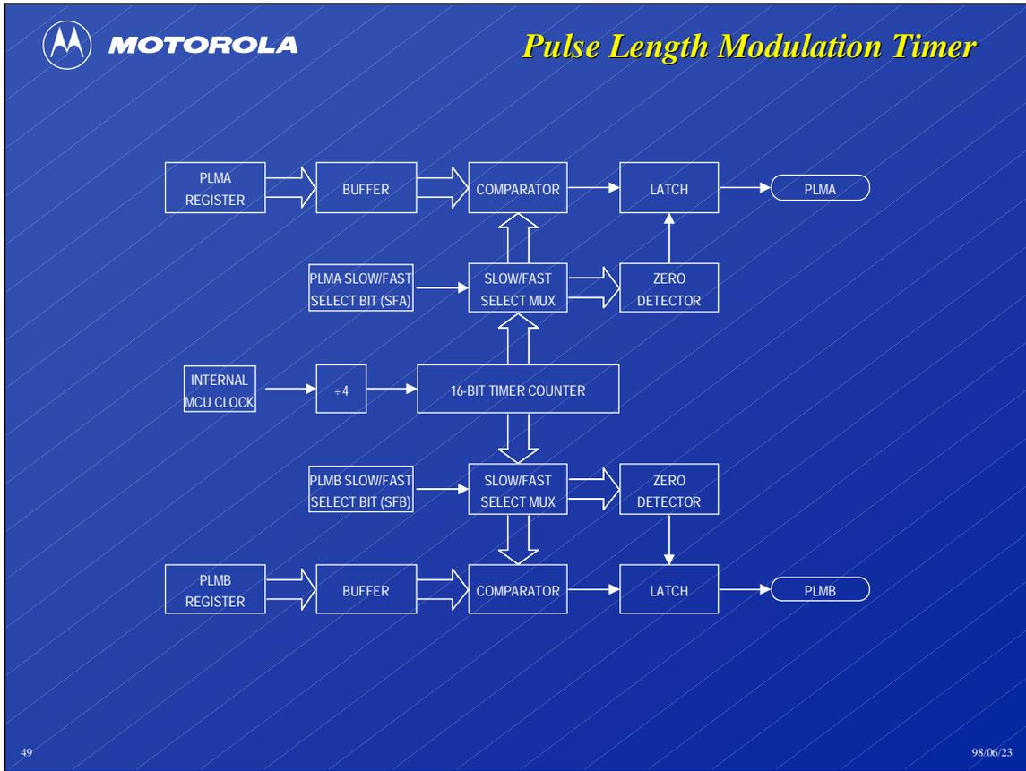
The pulse length modulation (PLM) timer has two channels, each with an 8-bit, buffered duty cycle register, an 8-bit comparator, zero detection circuitry, a slow/fast rate multiplexer, and a latch that drives an associated output pin.
