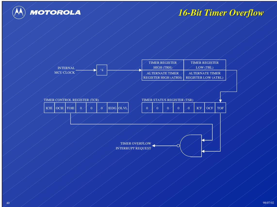
All functions of the 16-bit timer are related to the 16-bit counter which serves as its time base.
