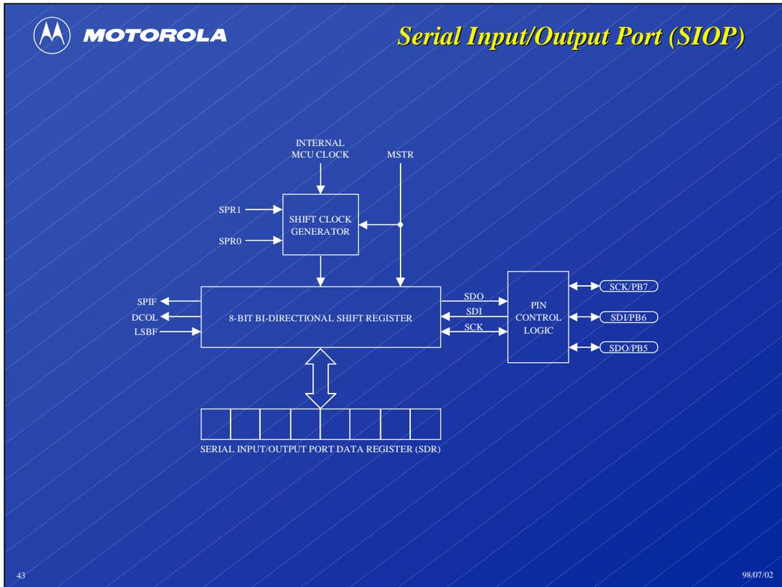
The serial input/output port (SIOP) is a simplified version of the serial peripheral interface (SPI) that appears on numerous Motorola microcontrollers ranging from other 68HC05 devices to members of the highly-integrated 68300 family. The SIOP supports master (processor initiated) and slave (externally initiated) mode transfers.
