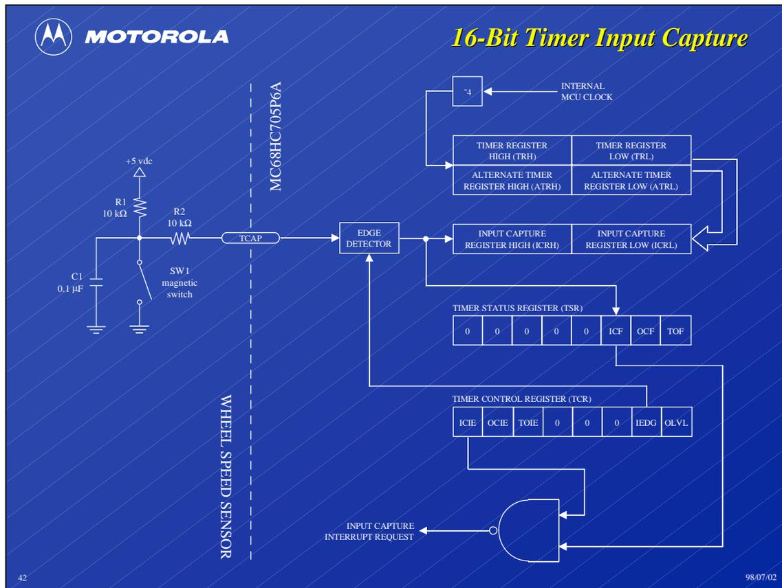
Input capture functions like output compare in reverse. Instead of generating an edge on the TCMP pin at a specific time, input capture saves the time at which a specific edge occurs on the TCAP pin.
