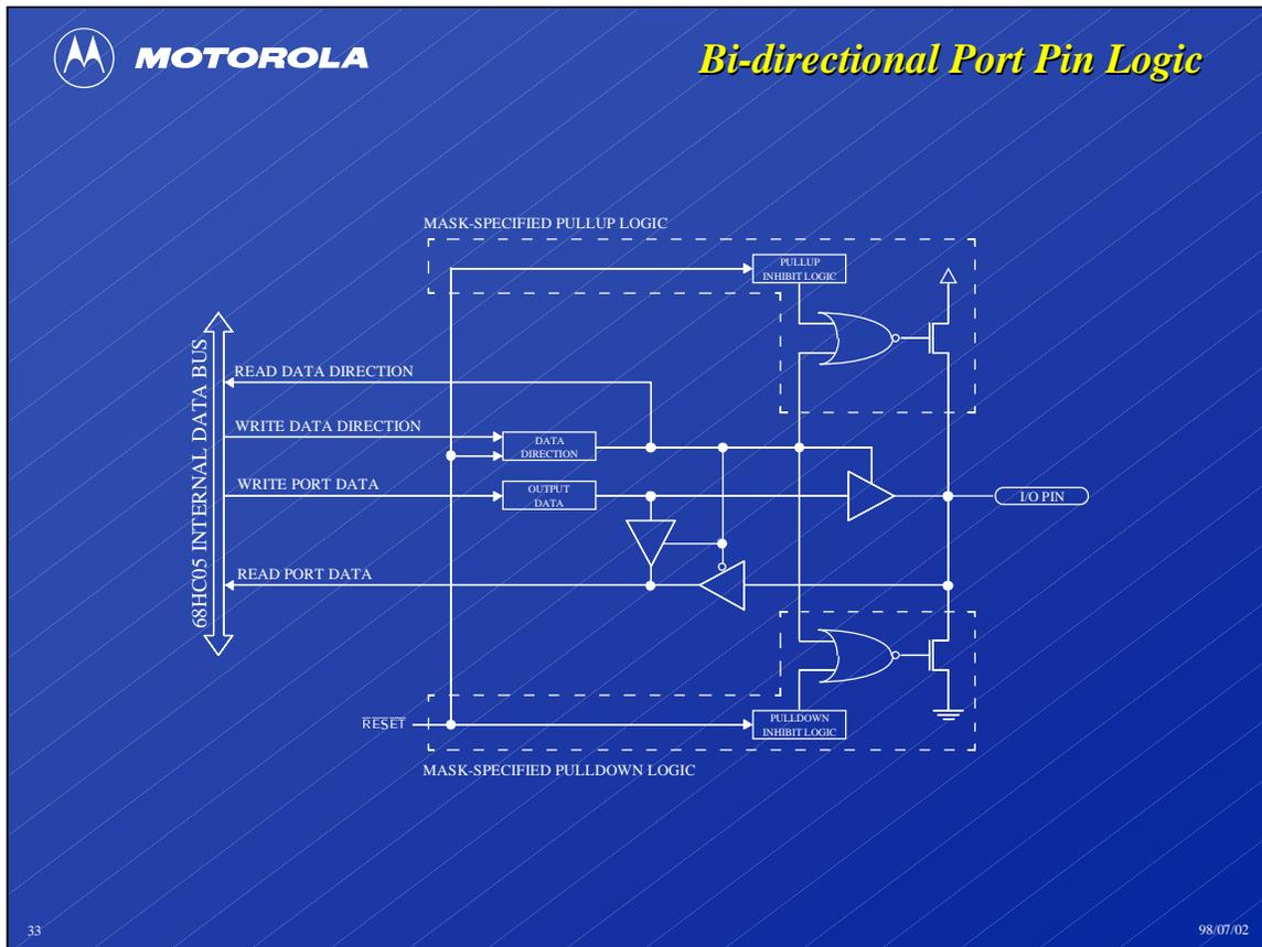
The diagram above shows a simplified version of the logic that comprises a bi-directional port pin. I/O pins, typically in groups of eight, comprise a single port.
