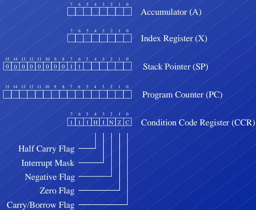
The 68HC05 central processor unit (CPU) consists of an accumulator (A), an index register (X), a stack pointer (SP), a program counter (PC), and a condition code register (CCR).
