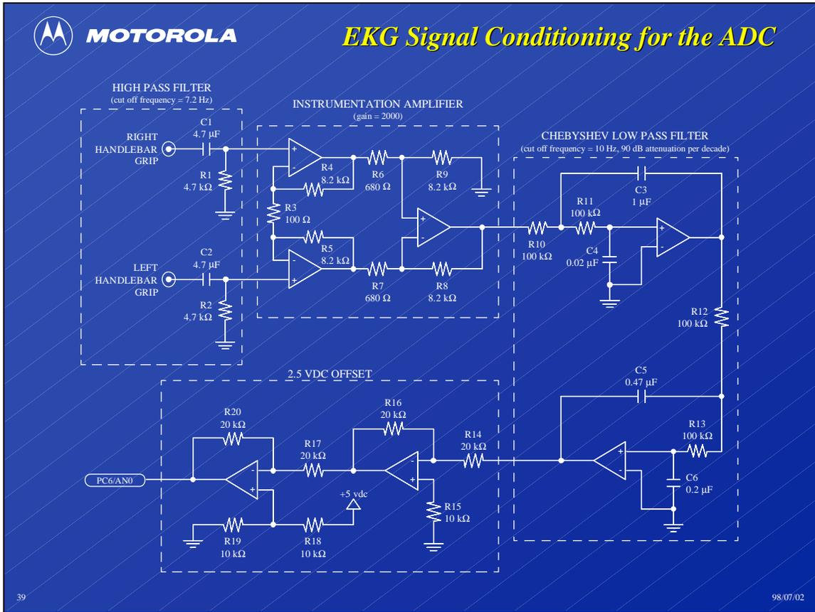
The cycling computer uses the analog-to-digital converter to sample the EKG signal that appears across the handlebar contacts when they are gripped.
