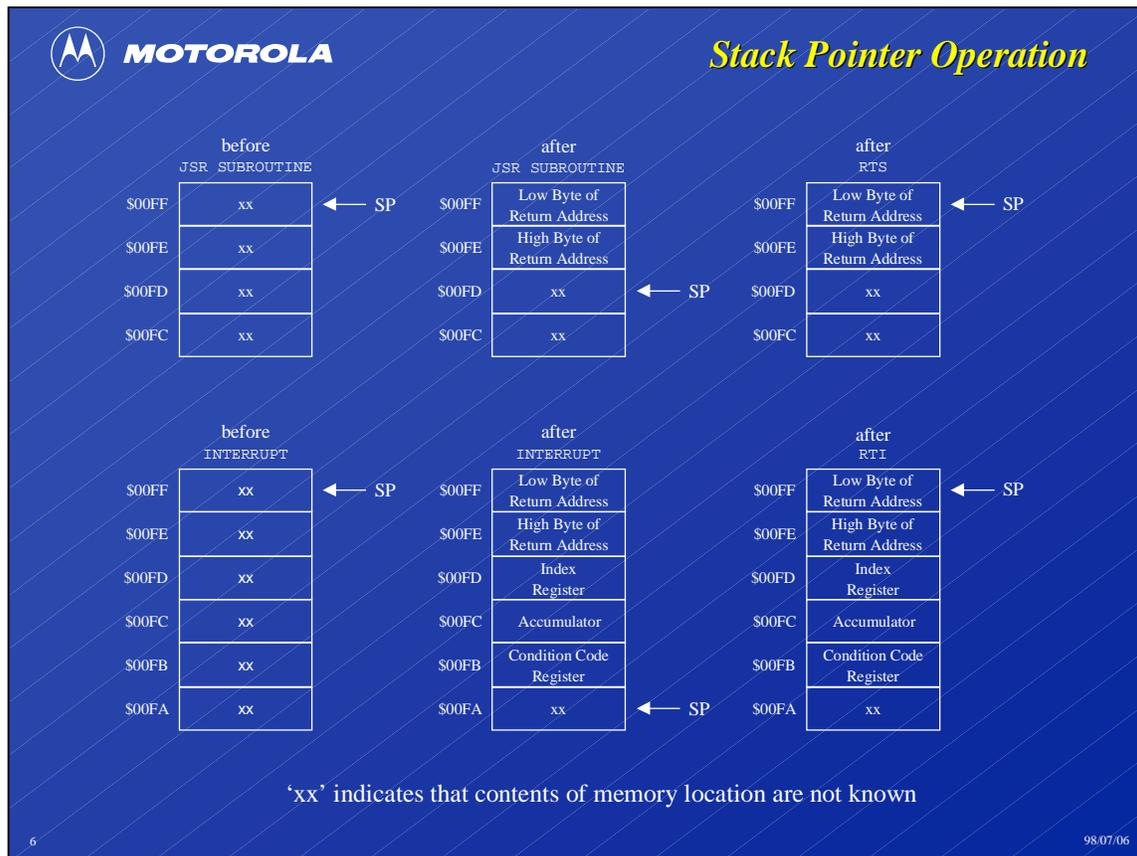
Processor state is saved on the stack when changes in program flow occur. The 68HC05 has a 64-byte hardware-controlled stack. Reset initializes the stack pointer to \$00FF; the RSP instruction does the same. No other instructions allow direct user manipulation of the stack.
