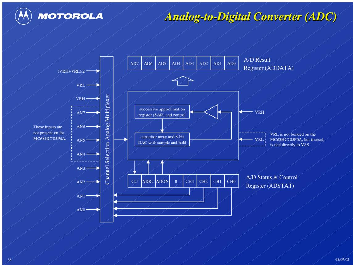
The MC68HC705P6A incorporates a 4-channel version of the 8-bit analog-to-digital converter (ADC) used on several 68HC05 devices.
