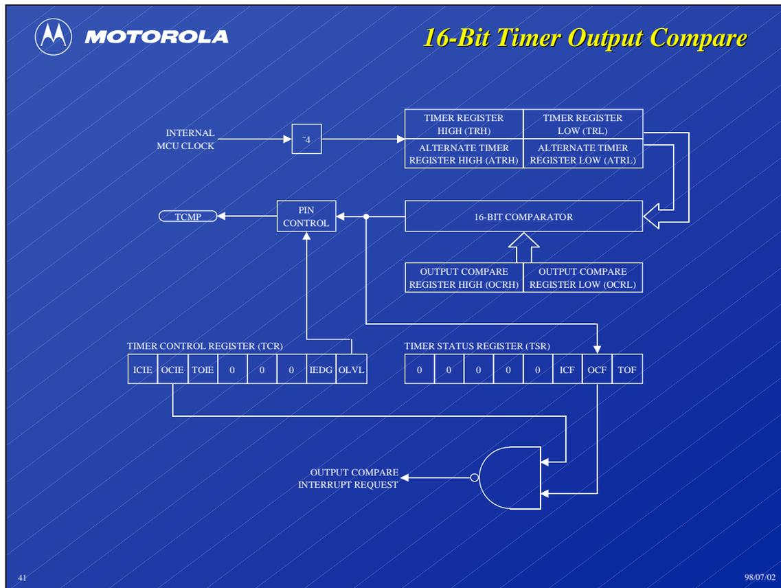
Output compare is essentially a method for generating delays, because it allows future events to be synchronized to the current value of the 16-bit timer counter.
