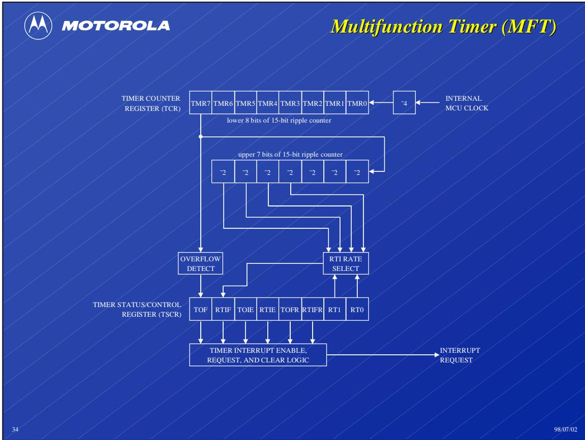
Simple 68HC05 devices have a simple timer, the multifunction timer (MFT). Consisting of a 15-bit ripple counter, the lower eight bits of which can be read from the timer counter register (TCR), the MFT is clocked at one fourth the internal MCU clock frequency.
