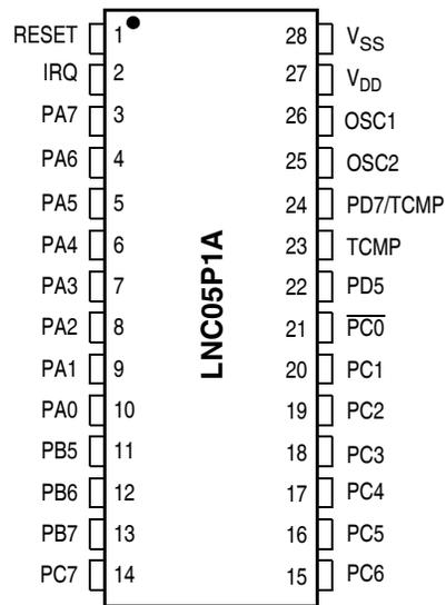
**Figure 3. LNC05P1A Pinout**
