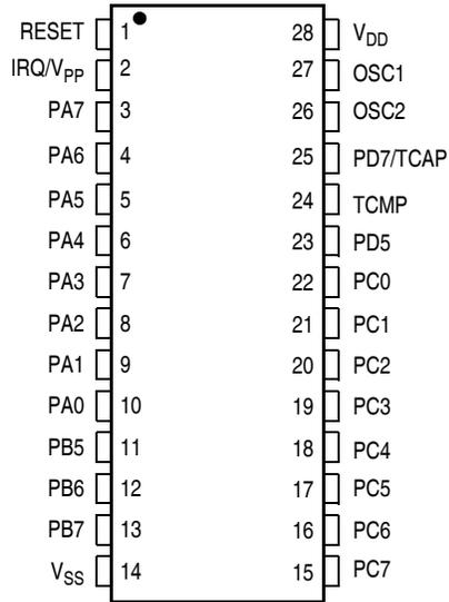
**Figure 2. Pinout**
