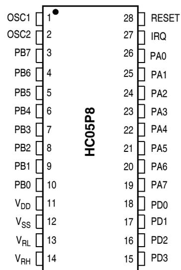
**Figure 5. HC05P8 Pinout**
