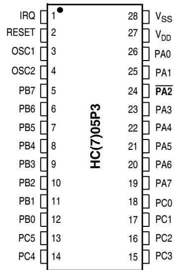
**Figure 4. HC705P3 Pinout**
