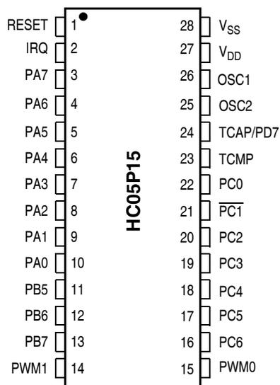
**Figure 6. HC05P15 Pinout**
