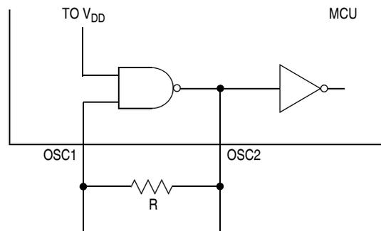
**Figure 1. RC Oscillator Circuit Diagram**
