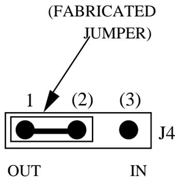
**NOTE:** Using the F4EM with the fabricated jumper installed between pins 2 and 3 will interfere with correct operation of the RESETIN and RESETOUT commands. The J4 pins 2-and-3 configuration is **not** correct for a F4EM that is part of an MMDS05 system.
