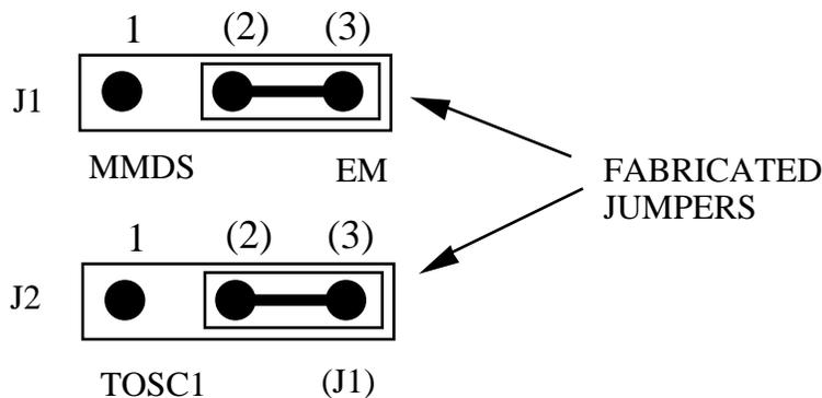
Jumper J2 can be used to select between an internal generated clock or a external clock generated by the target system. If the target clock is selected by placing the jumper on J2 between pins 1 and 2 the position of the fabricated jumper on J1 does not matter.
