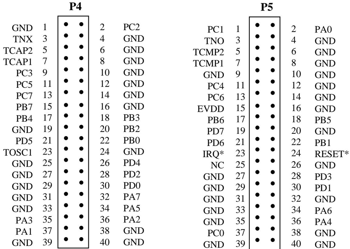
Figure 1-2. Target Connector
