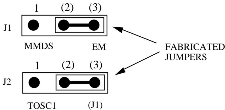
Alternatively, you may use a clock source originating from the MMDS05 control board. To do so, reposition the J1 jumper between pins 1 and 2. Then use the MMDS OSC command to select clock frequency.
