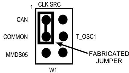
There are two other possible clock sources. To use the one originating from the development system platform, reposition the W1 jumper header between the MMDS05 and COMMON pins. Then use the system's OSC command to select a frequency.
