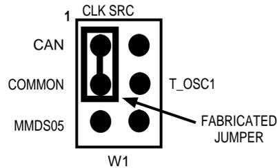
Another possible clock source is a user supplied clock source, coming through the target cable connected to J2. To use this source, reposition the W1 jumper header between the T\_OSC1 and COMMON pins.
