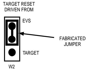
**NOTE:** *The TARGET configuration is not correct for an M68EM05P18 that is part of an MMDS or MMEVS. Such a configuration would interfere with correct operation of the RESETIN and RESETOUT commands.*
