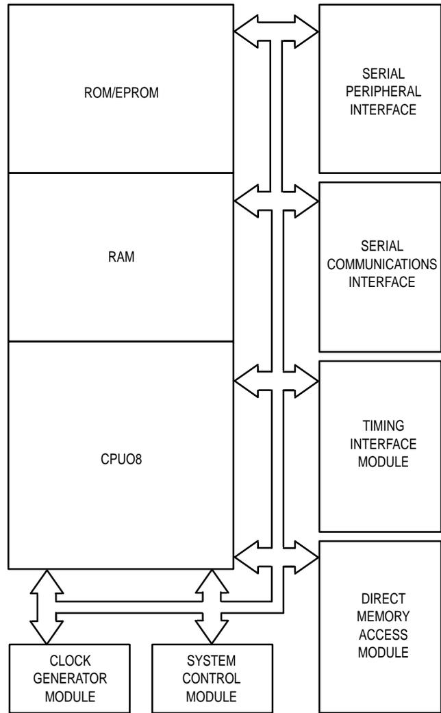
Figure 3. Block Diagram of Typical M68HC08 MCU
