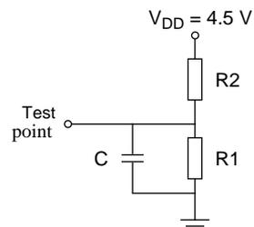
**Figure 9-1** Equivalent test load
