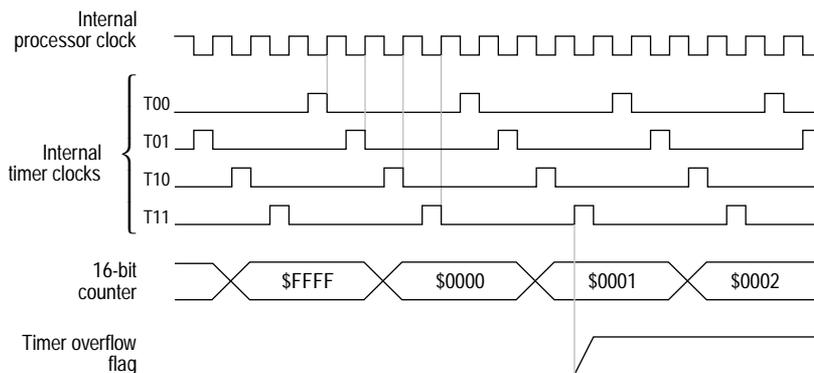
**Note:** The timer overflow flag is set at timer state T11 (transition of counter from \$FFFF to \$0000). It is cleared by a read of the timer status register during the internal processor clock high time, followed by a read of the counter low register.
