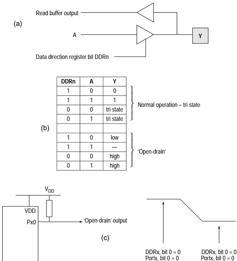
**Figure 4-3** Port logic levels
