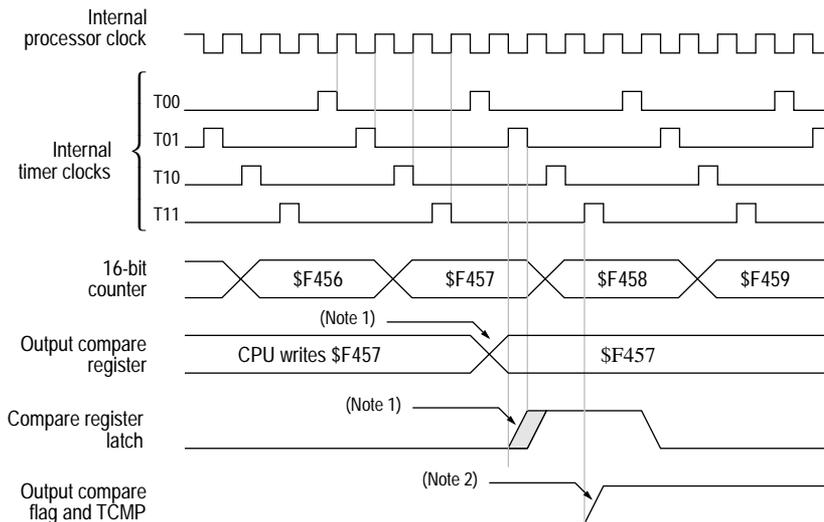
**Note:** (1) The CPU write to the compare registers may take place at any time, but a compare only occurs at timer state T01. Thus a four cycle difference may exist between the write to the compare register and the actual compare. (2) The output compare flag is set at the timer state T11 that follows the comparison match (\$F457 in this example).
