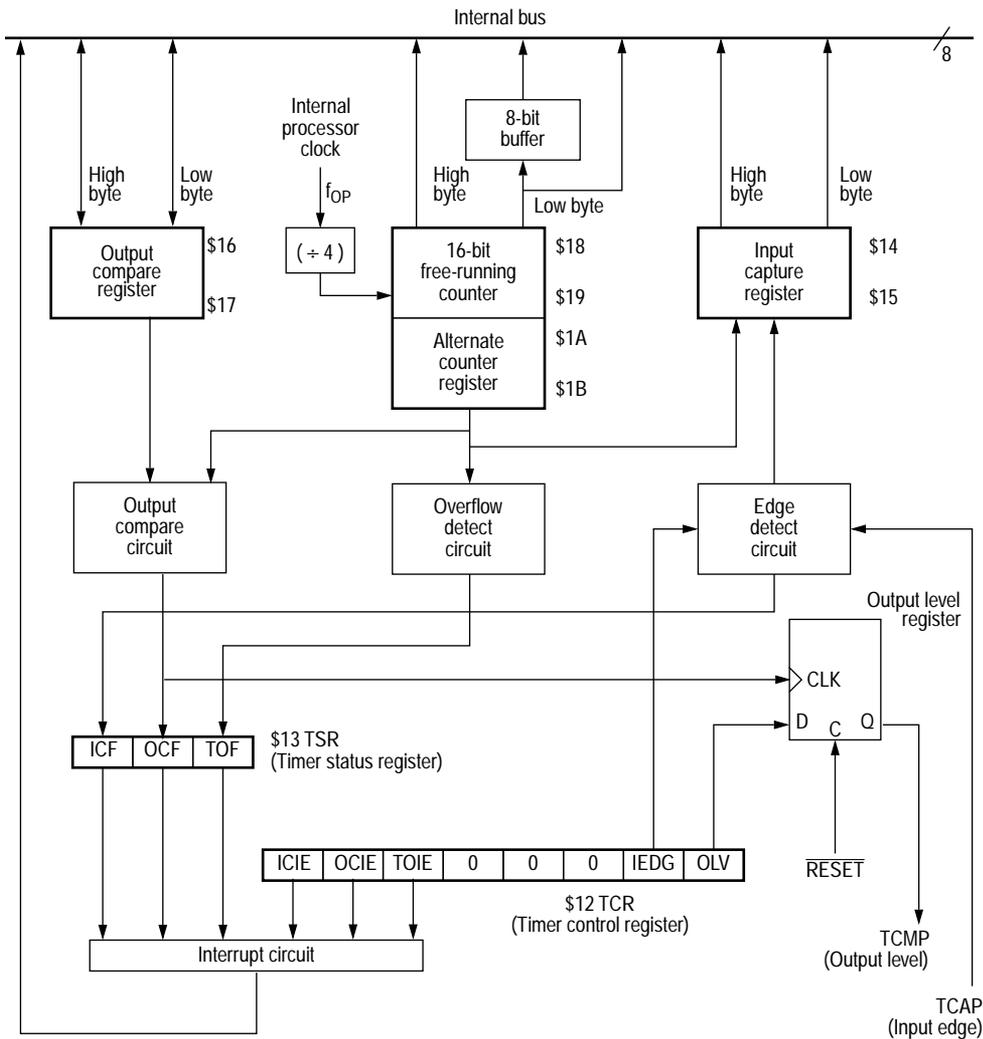
Figure 6-1 16-bit programmable timer block diagram
