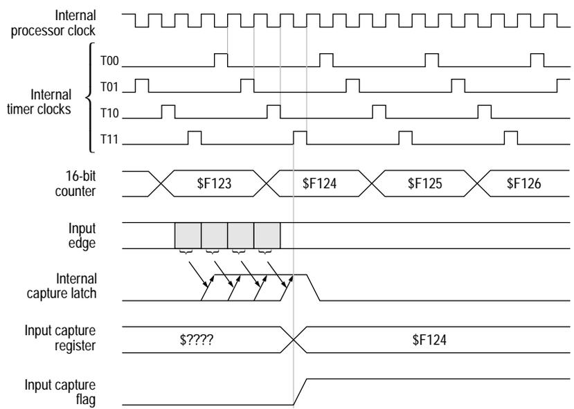
Note: If the input edge occurs in the shaded area from one timer state T10 to the next timer state T10, then the input capture flag will be set during the next T11 state.
