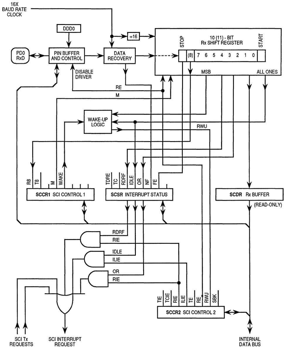
Figure 7-2. SCI Receiver Block Diagram
