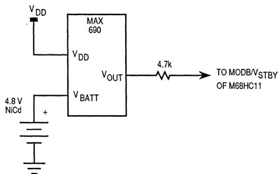
**Figure 4–3. RAM Standby MODB/ $V_{STBY}$  Connections**
