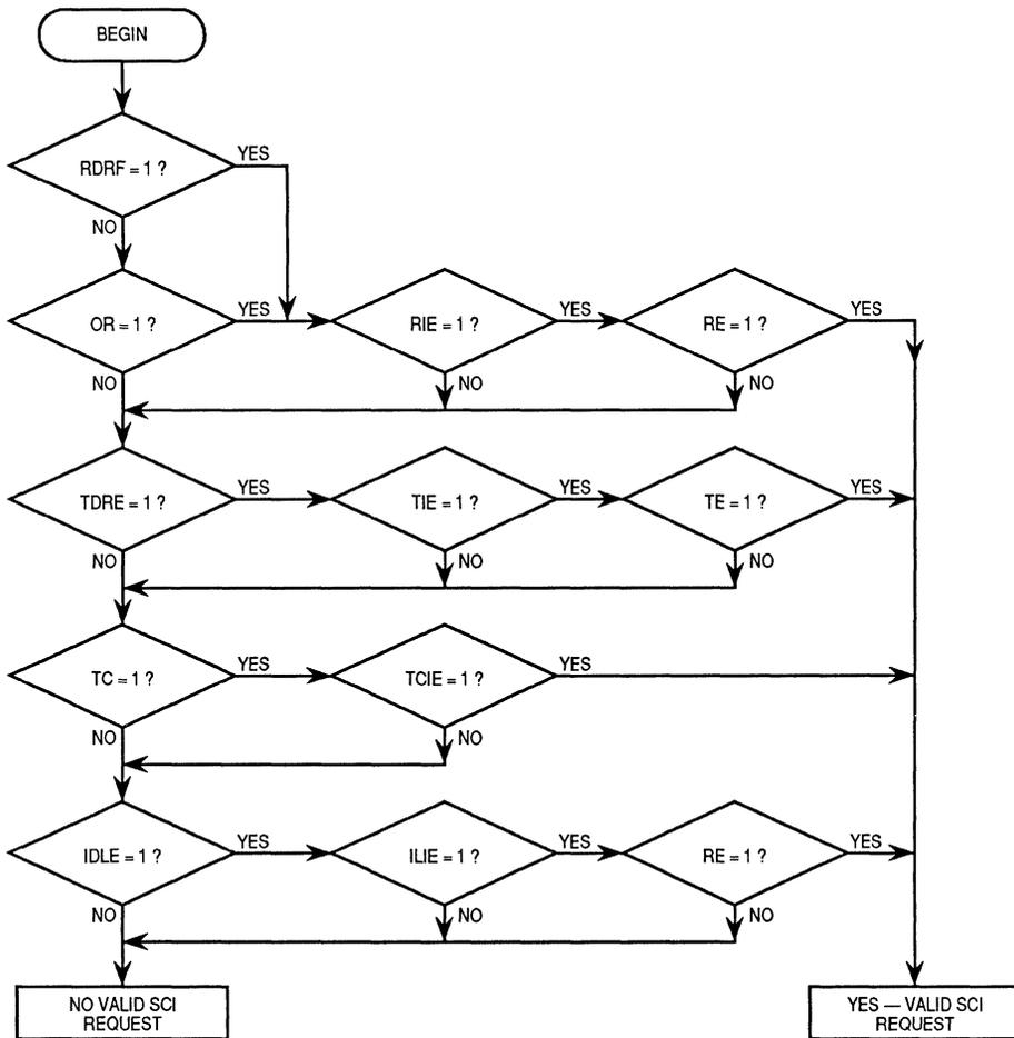
**Figure 5-3. Interrupt Source Resolution within SCI**
