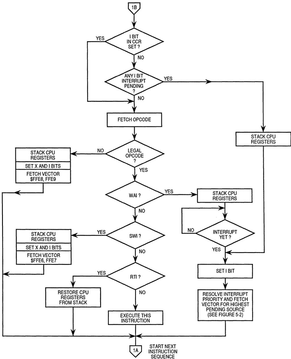
Figure 5-1. Processing Flow out of Reset (2 of 2)
