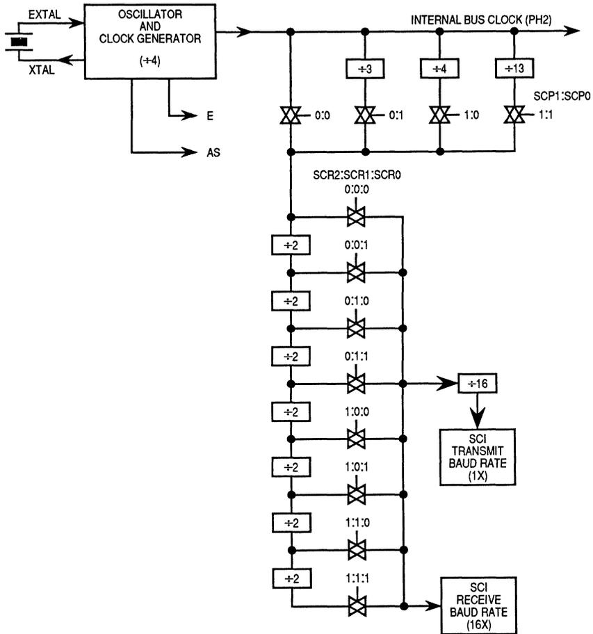
Figure 7-3. SCI Baud Rate Diagram
