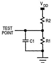
Equivalent Test Load<sup>1</sup>
