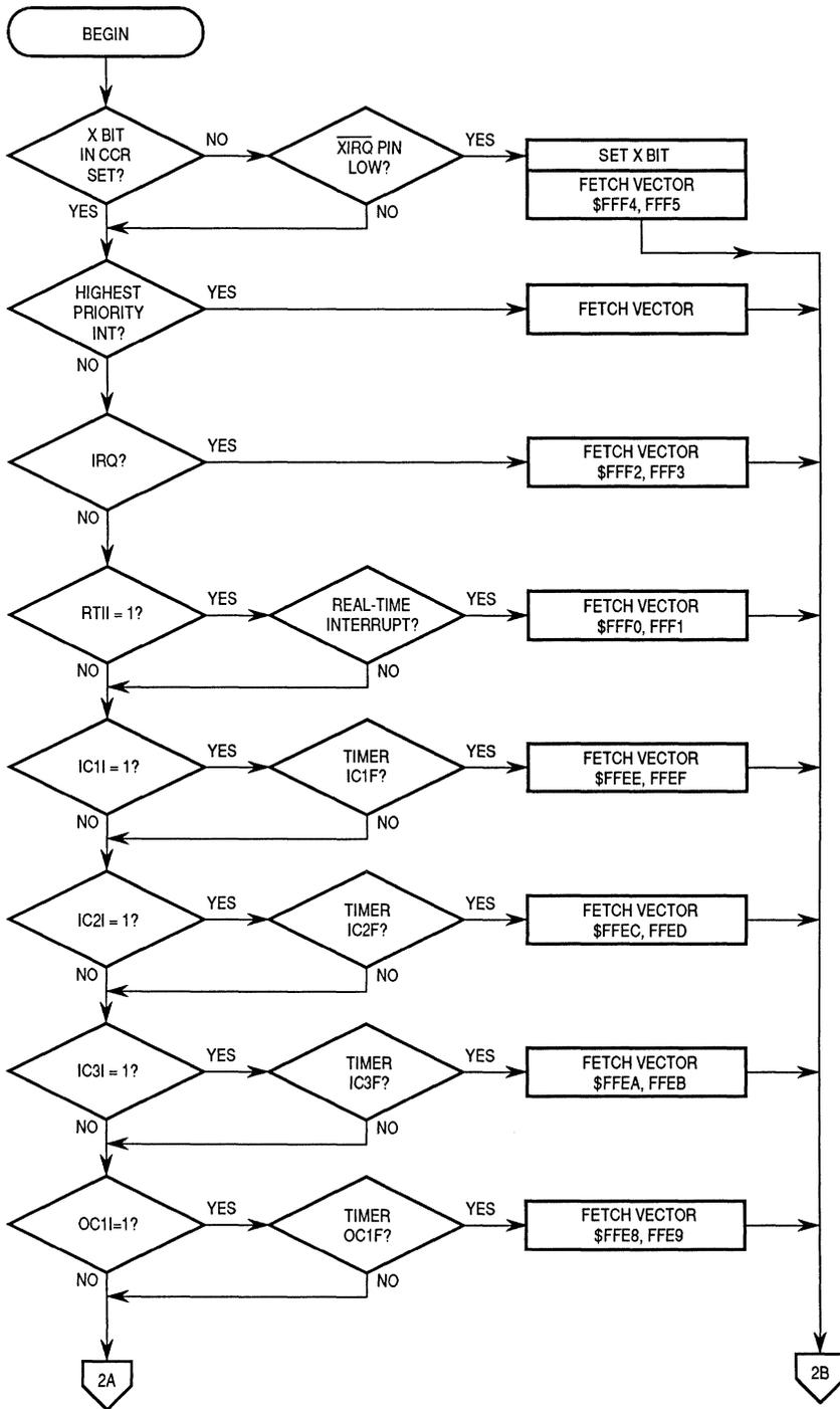
Figure 5-2. Interrupt Priority Resolution (1 of 2)
