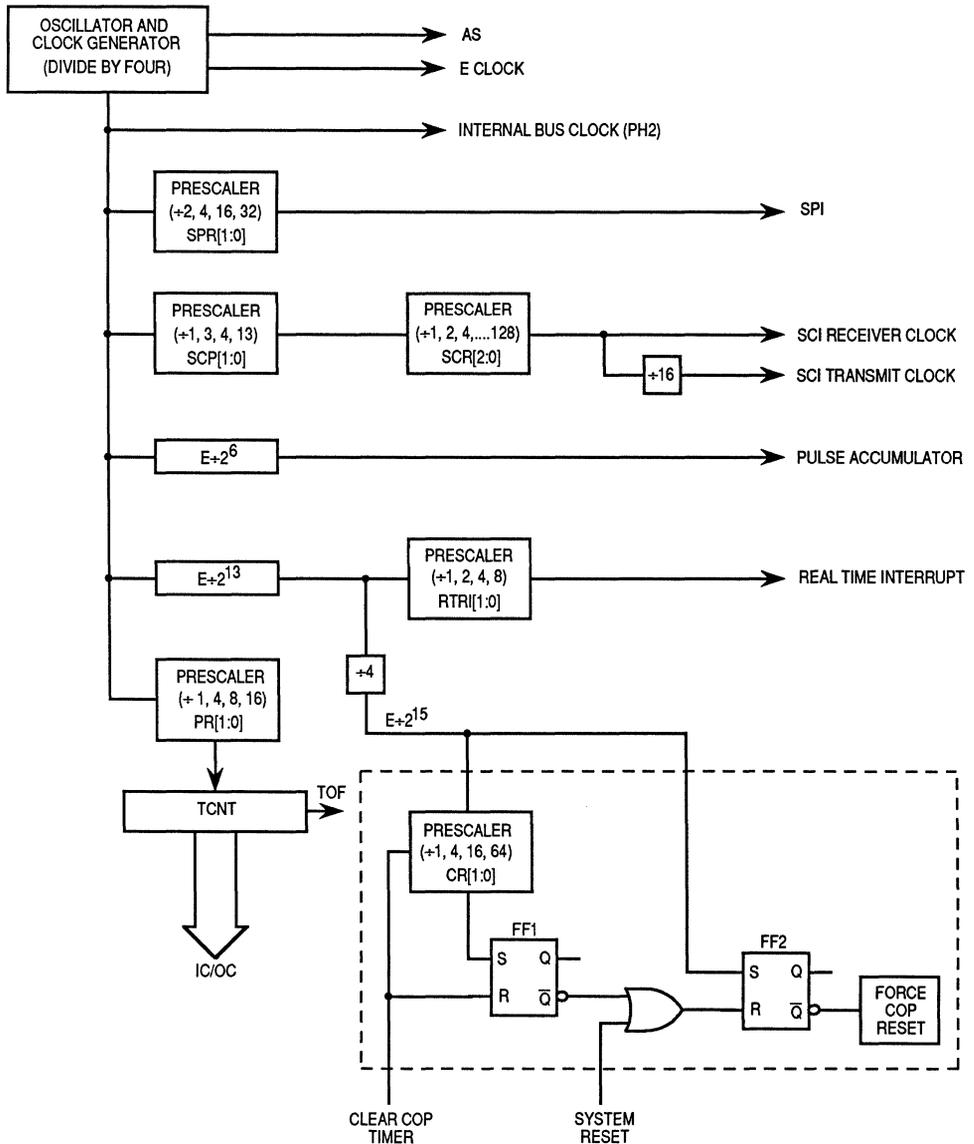
**Figure 9–1. Timer Clock Divider Chains**
