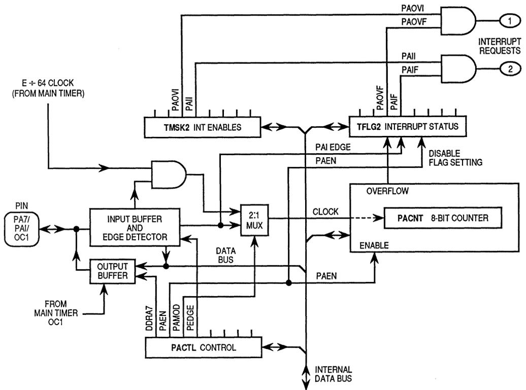
Figure 9-3. Pulse Accumulator
