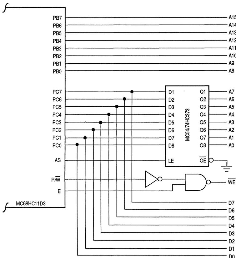
**Figure 4-1. Address/Data Demultiplexing**
