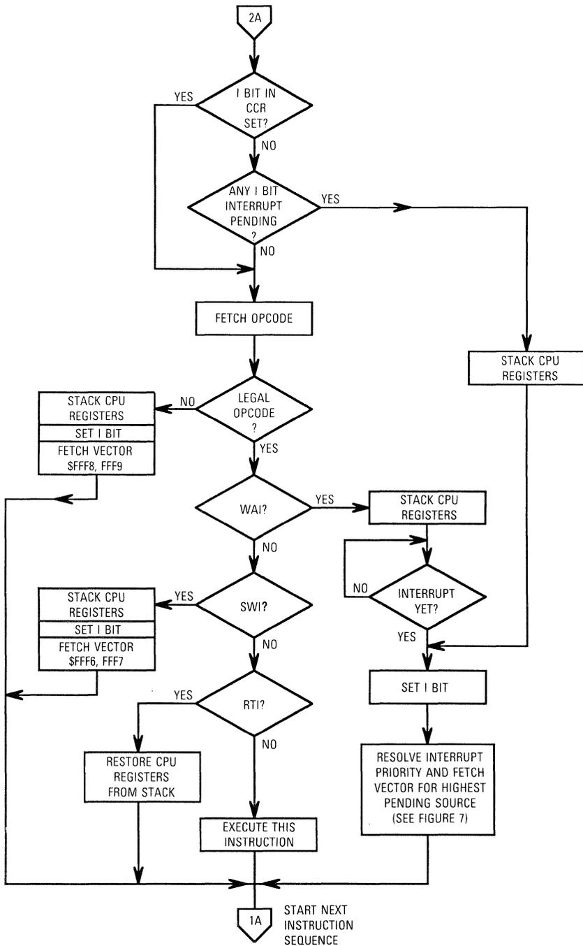
Figure 6-3. Processing Flow Out of Resets (Sheet 2 of 2)
