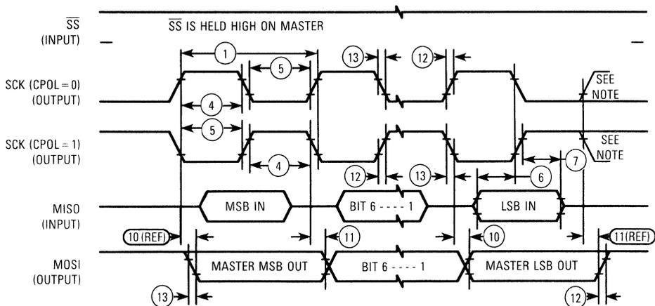
NOTE: The last clock edge is generated internally but is not seen at the SCK pin.
