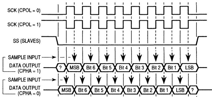
**Figure 10-3. SPI Data Clock Timing Diagram**
