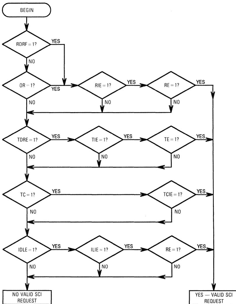
**Figure 6-5. Interrupt Source Resolution within SCI**
