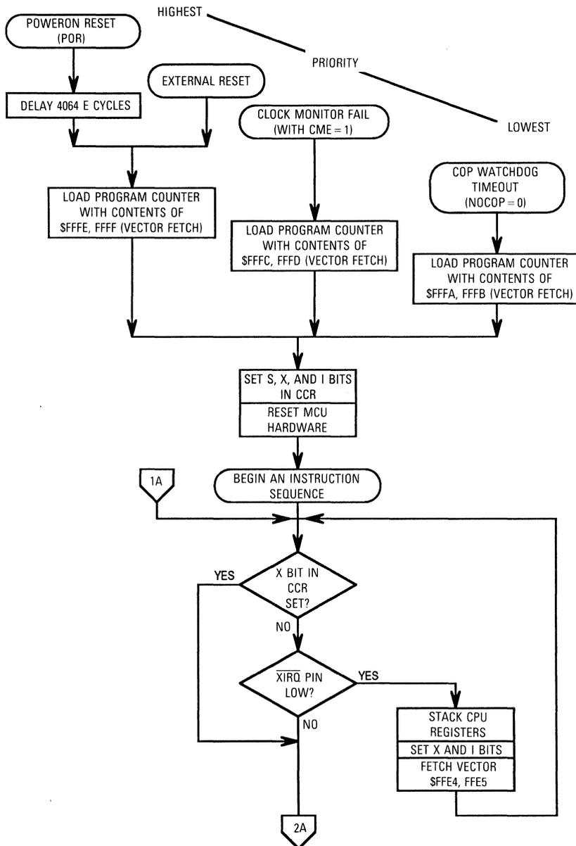
Figure 6-3. Processing Flow Out of Resets (Sheet 1 of 2)
