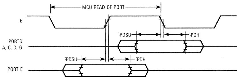
**Figure 13-8. Port Read Timing Diagram**
