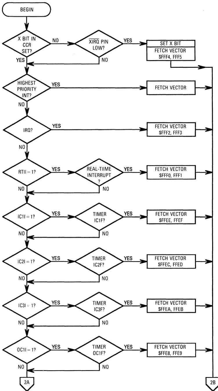
Figure 6-4. Interrupt Priority Resolution (Sheet 1 of 2)
