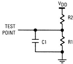
Equivalent Test Load<sup>1</sup>
