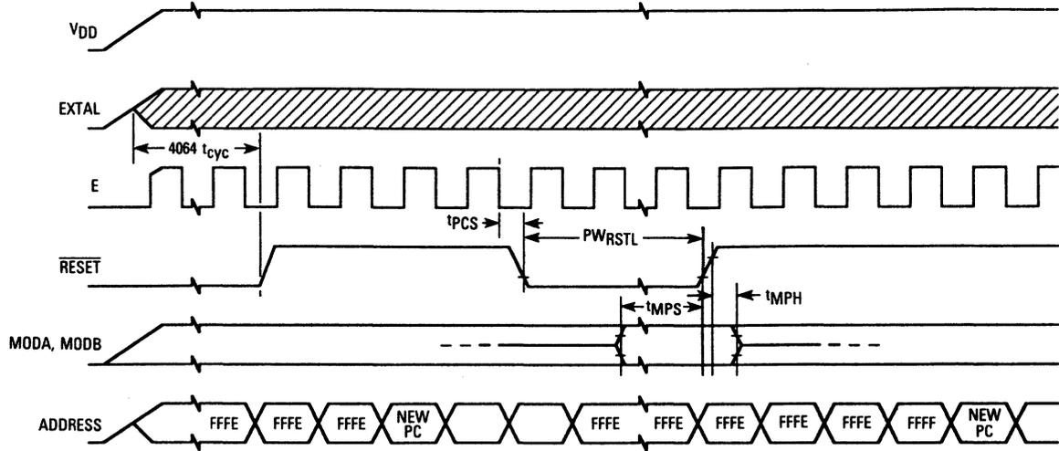
Figure 13-3. POR External Reset Timing Diagram
