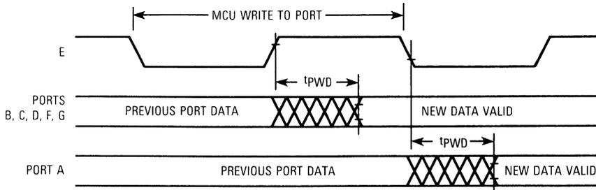
**Figure 13-7. Port Write Timing Diagram**
