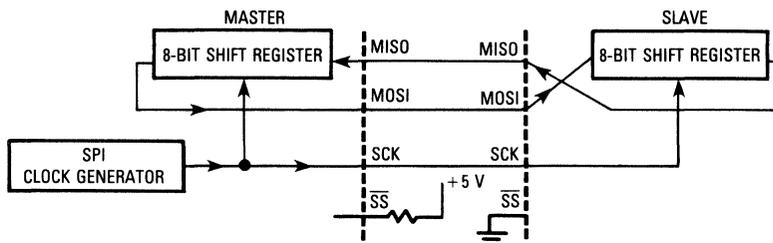
**Figure 10-2. SPI Master-Slave Interconnections**
