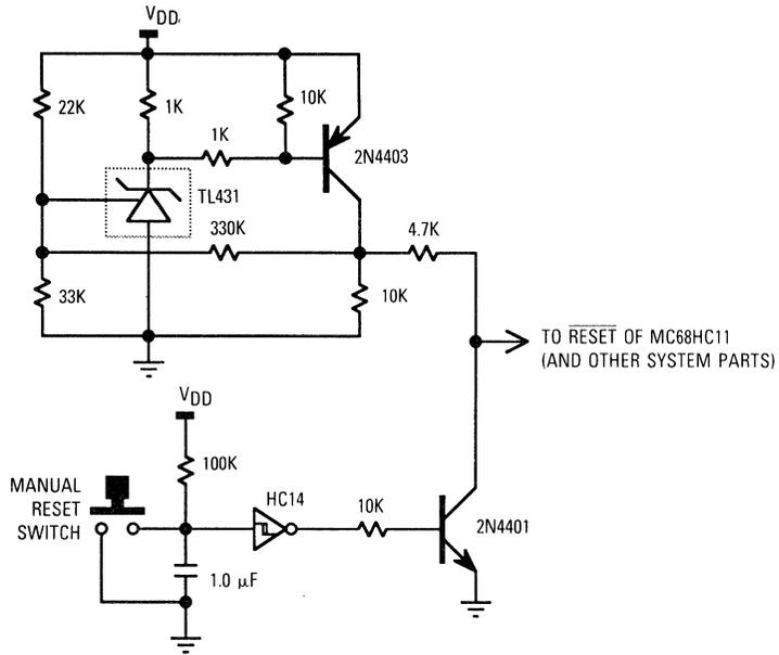
**Reset Circuit with LVI and RC Delay**
