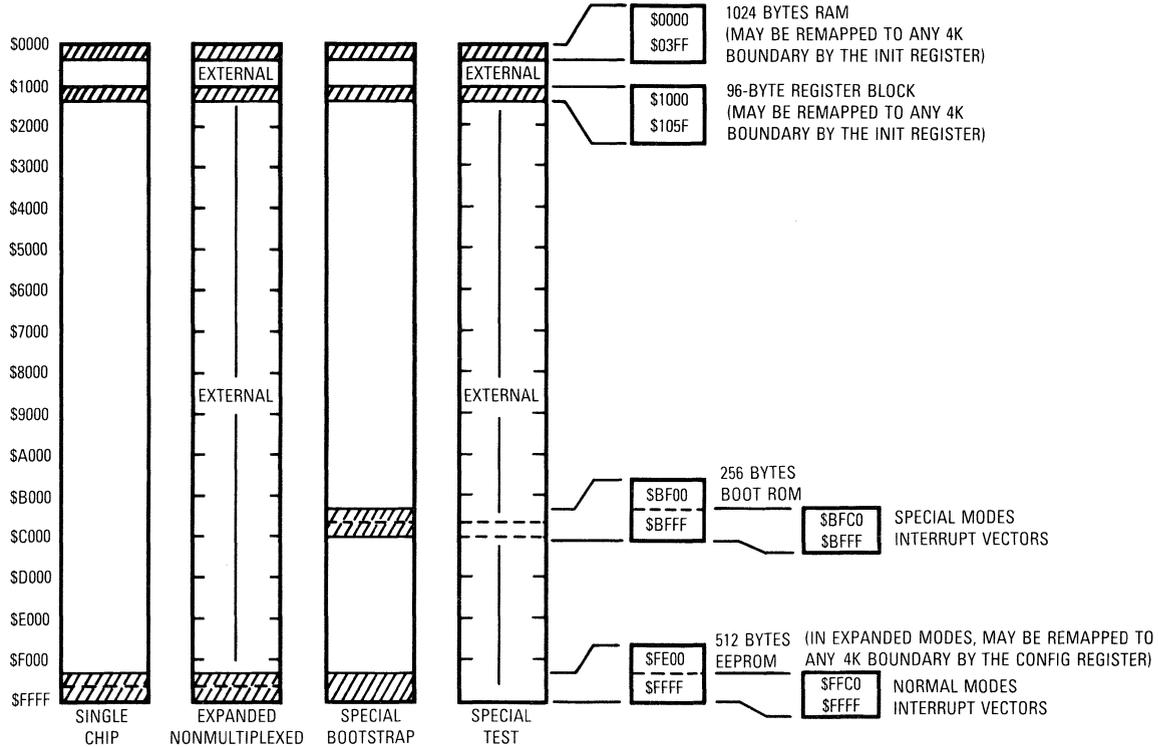
NOTE: The EEPROM can be enabled in special test mode by writing a one to the EEOB bit of the CONFIG register after reset.
