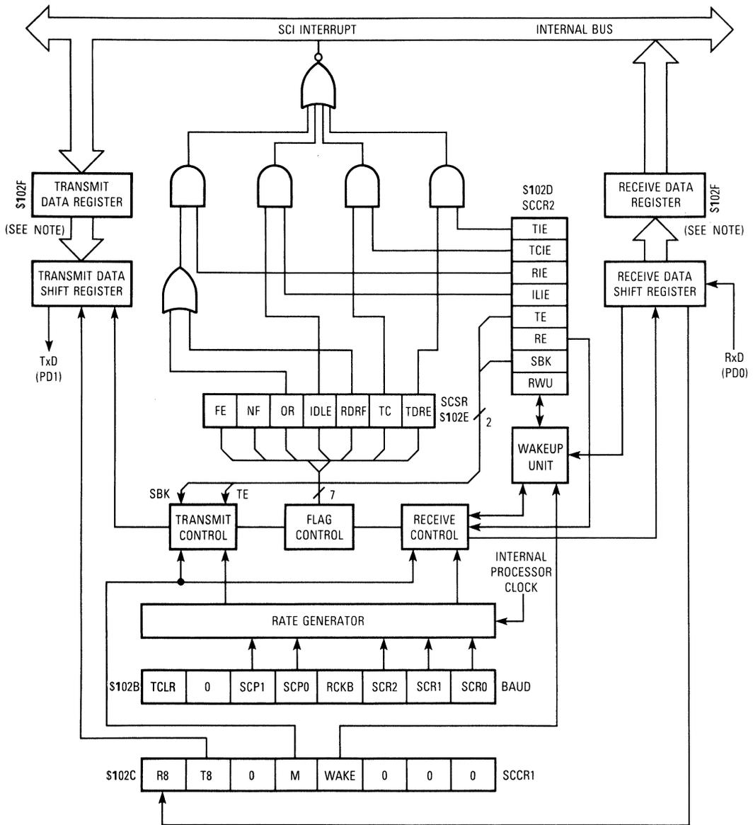
NOTE: The serial communications data register (SCDR) is controlled by the internal  $R/\bar{W}$  signal. It is the transmit data register when written and received data register when read.
