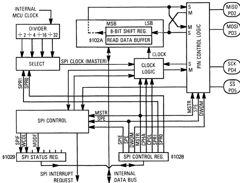
Figure 10-1. SPI Block Diagram
