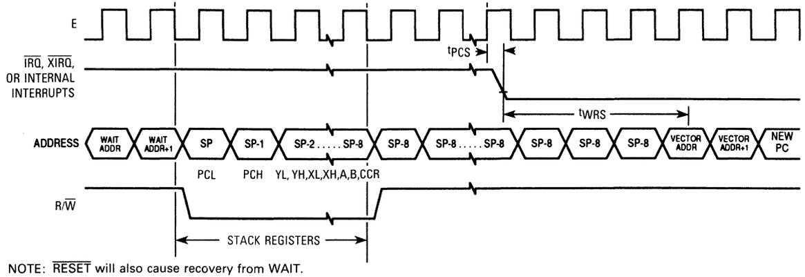
Figure 13-5. WAIT Recovery from Interrupt Timing Diagram
