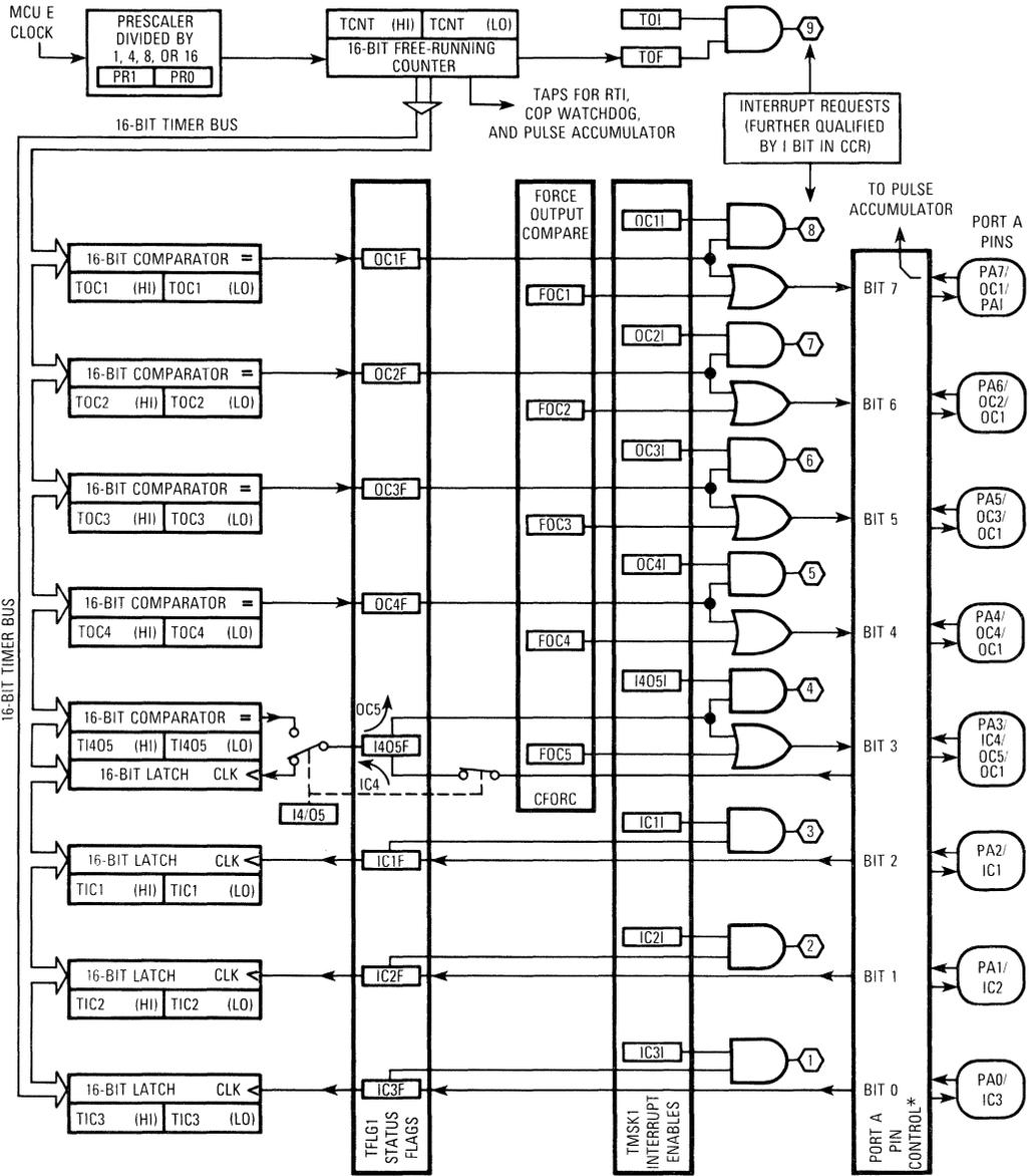
\*Port A pin actions controlled by DDRA, OC1M, OC1D, TCTL1, and TCTL2 registers.
