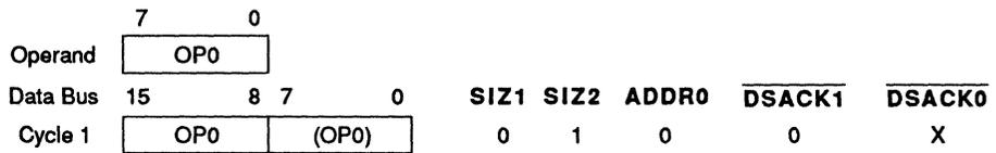
**Figure 4–8. Byte Operand to 16-Bit Port, Even (ADDR0 = 0)**
