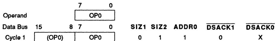
**Figure 4–9. Byte Operand to 16-Bit Port, Odd (ADDR0 = 1)**
