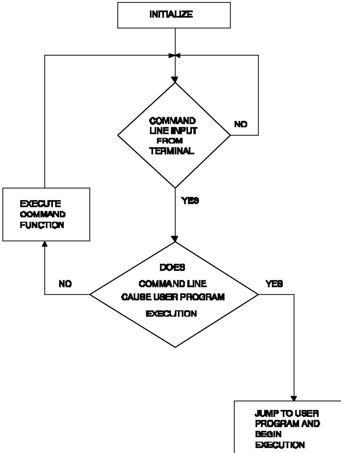
Figure 2-1. Flow Diagram of dBUG Operational Mode.
