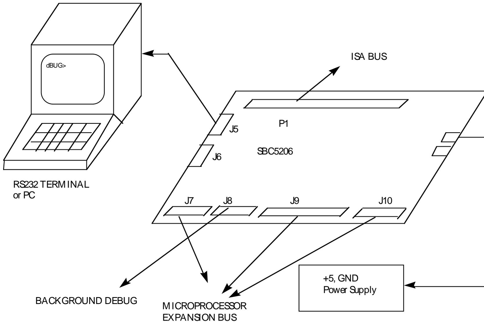
Figure 1.2. System Configuration
