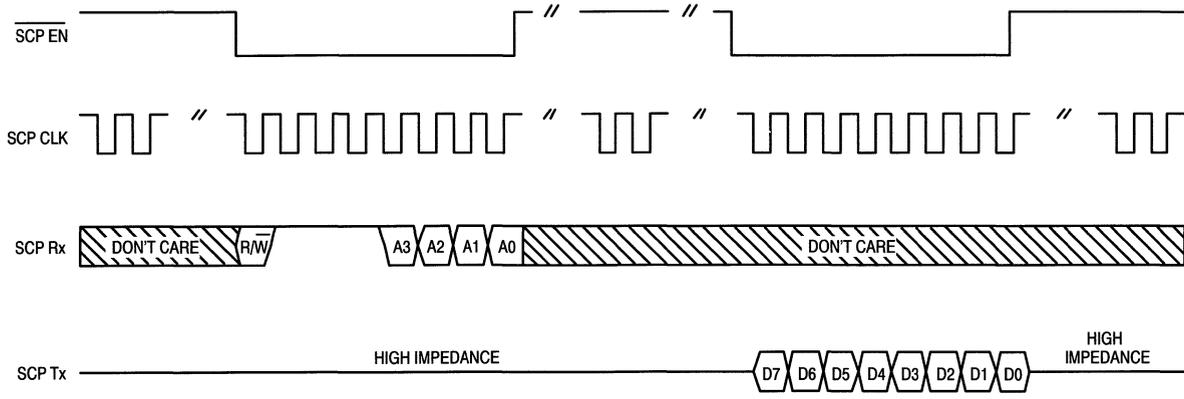
**Figure 5-4. Serial Control Port Byte Read Operation
