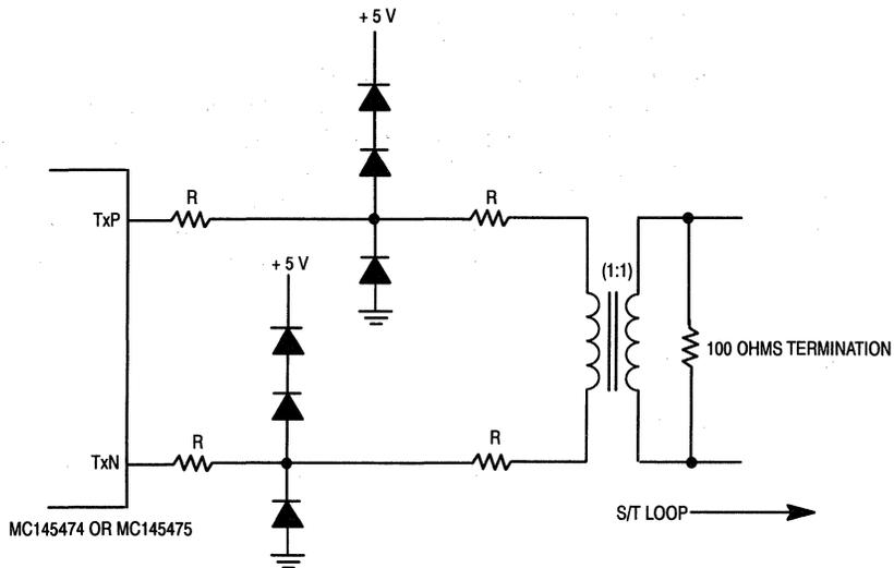
NOTE:  $4R + \text{winding resistance} = 26.4 \text{ ohms}$ .
