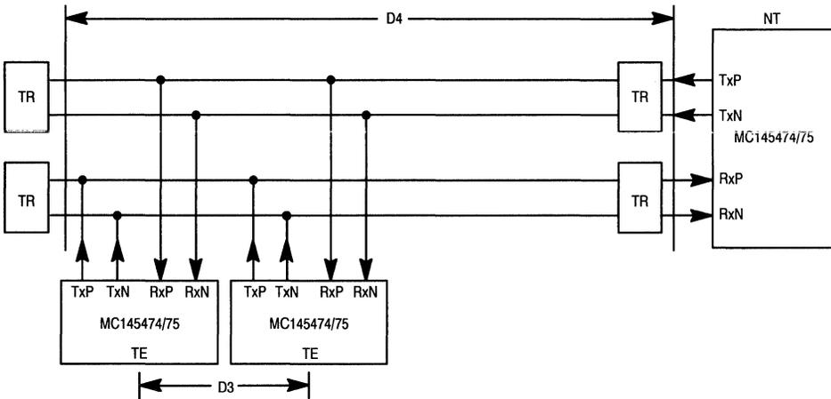
Figure 2-3. Extended Passive Bus
