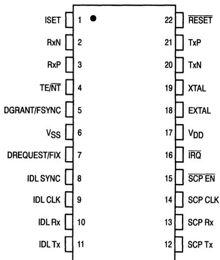
Figure 16-1. MC145474 Pin Assignment
