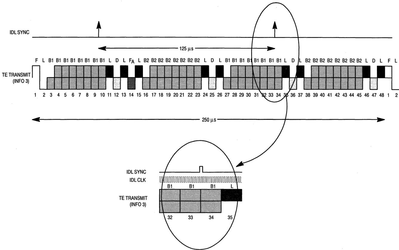
Figure 4-4. Phase Relationship of TE Transmit Signal
