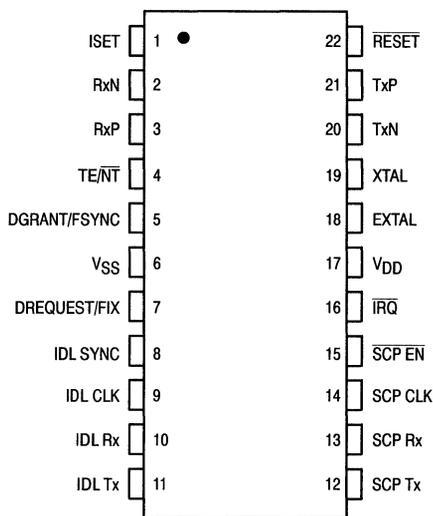
Figure 6-1. MC145474 Pin Assignment
