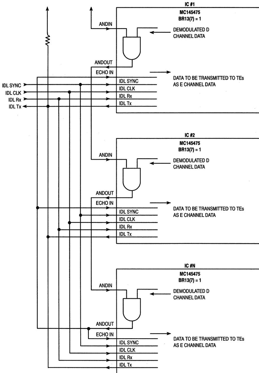
Figure 11-1. NT1 Star Mode of Operation
