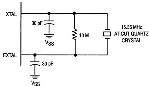
Figure 6-3. Crystal Circuit
