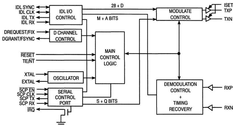
Figure 1-1. MC145474/75 Block Diagram
