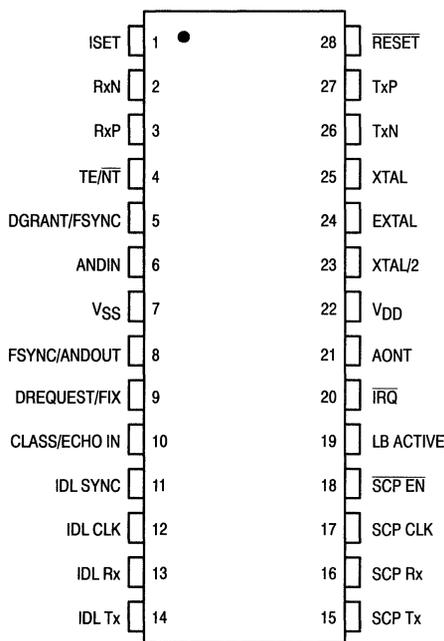
Figure 6-2. MC145475 Pin Assignment
