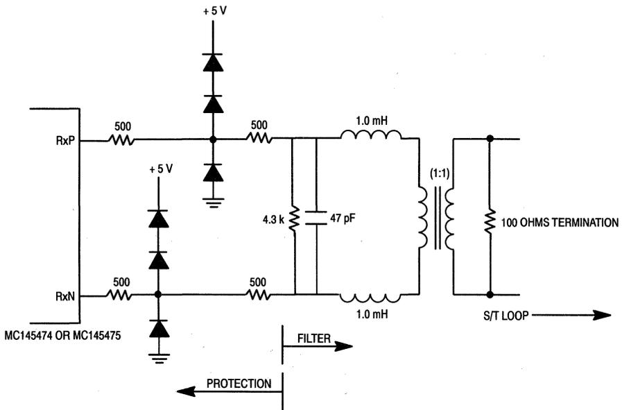
**Figure 14-2. Receive Line Interface Circuit**
