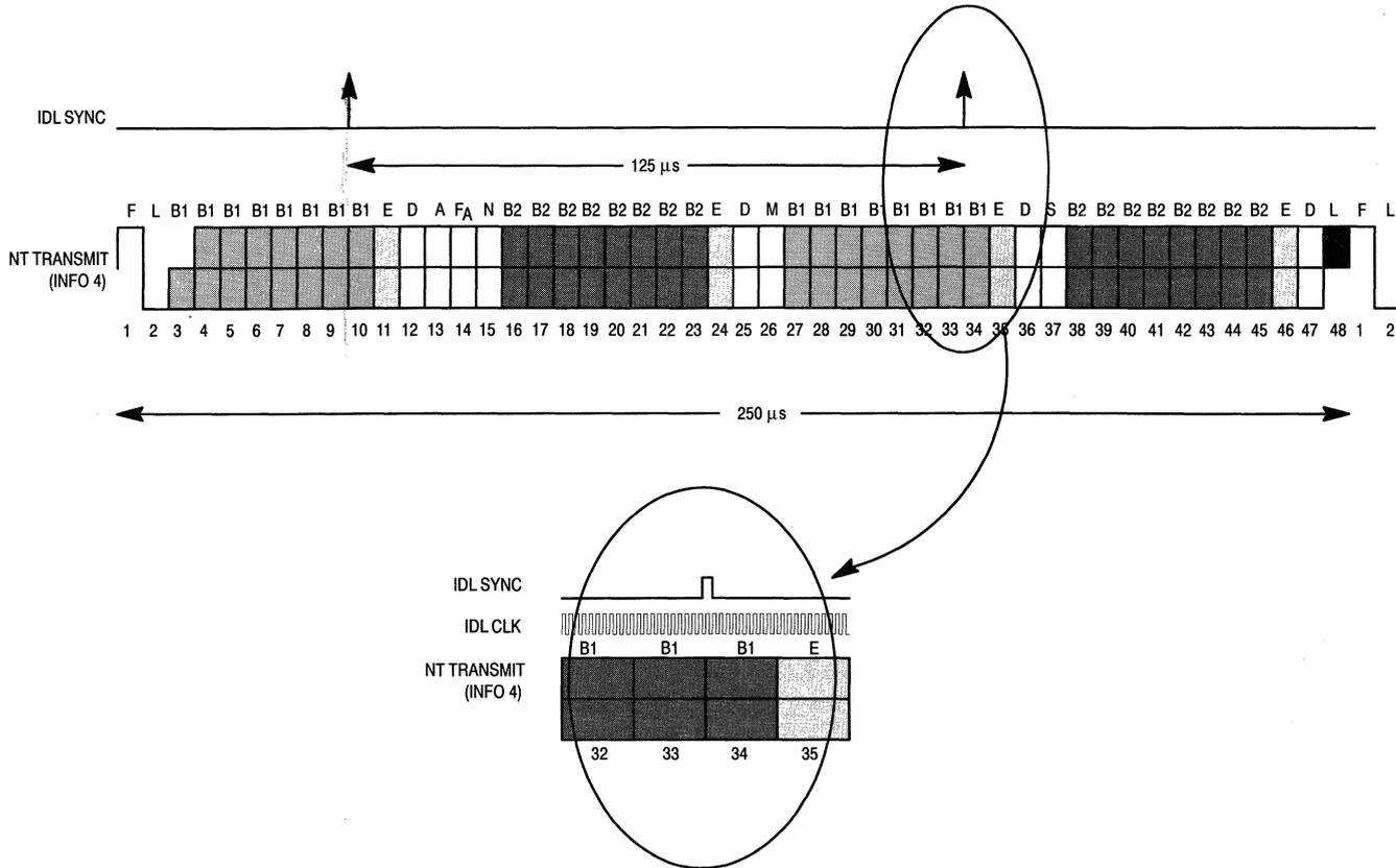
Figure 4-2. Phase Relationship of NT Transmit Signal
