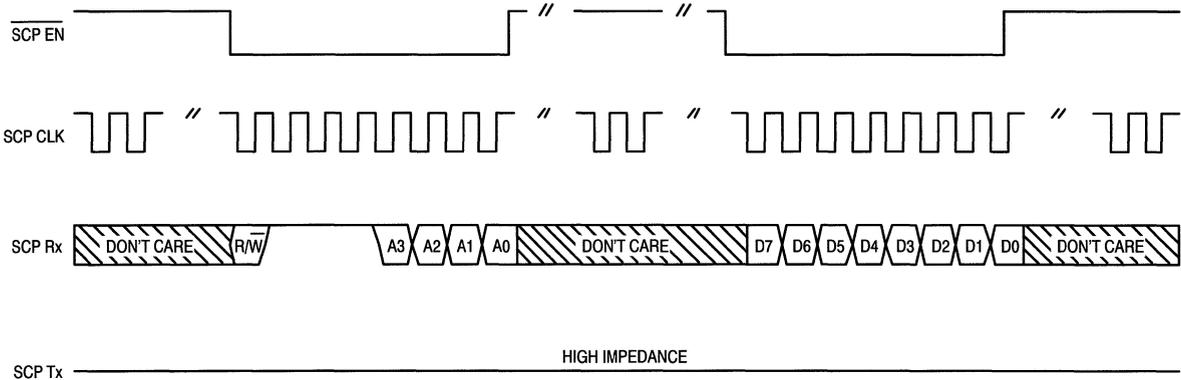
**Figure 5-6. Serial Control Port Byte Write Operation
