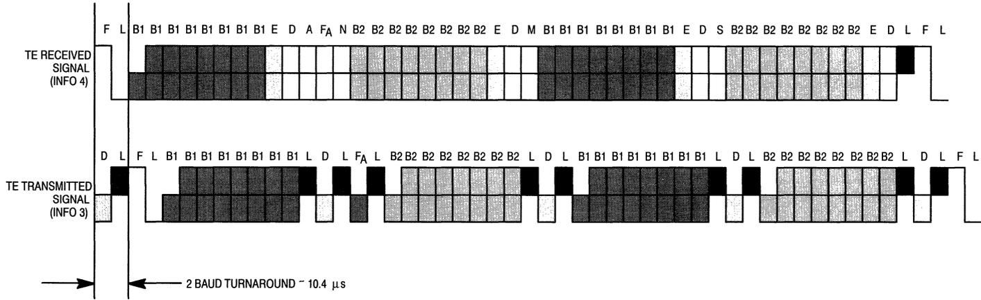
Figure 4-3. Two Baud Turnaround in TE
