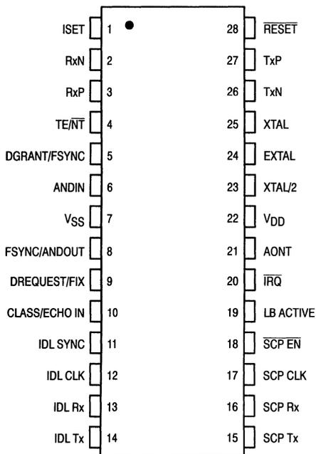
Figure 16-2. MC145475 Pin Assignment
