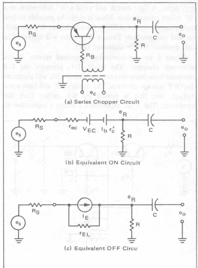
FIGURE 3 — Series Chopper Circuit
