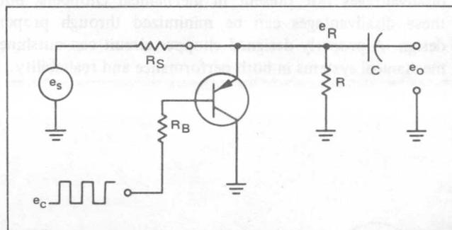
FIGURE 2 - Shunt-Transistor Chopper Circuit
