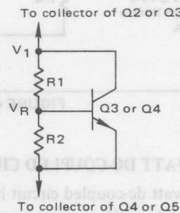
FIGURE 6 – Bias Circuit for Output Stage
