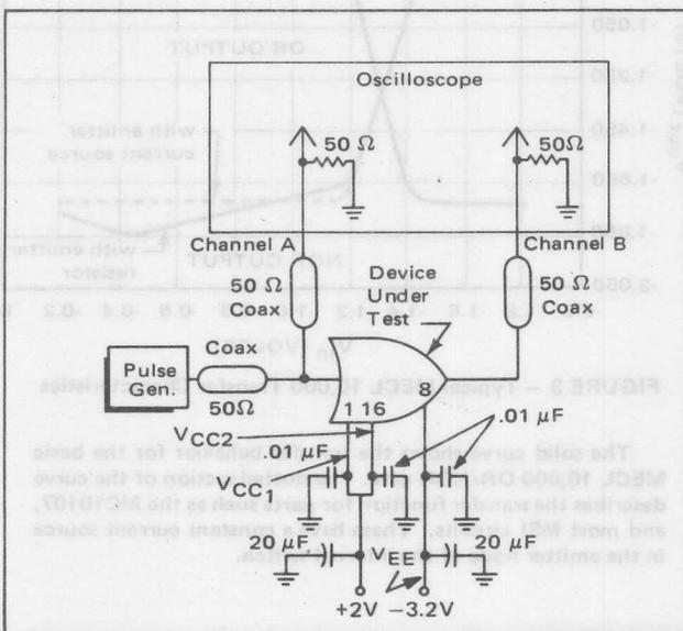
FIGURE 1A - MECL 10,000 Test Fixture Schematic
