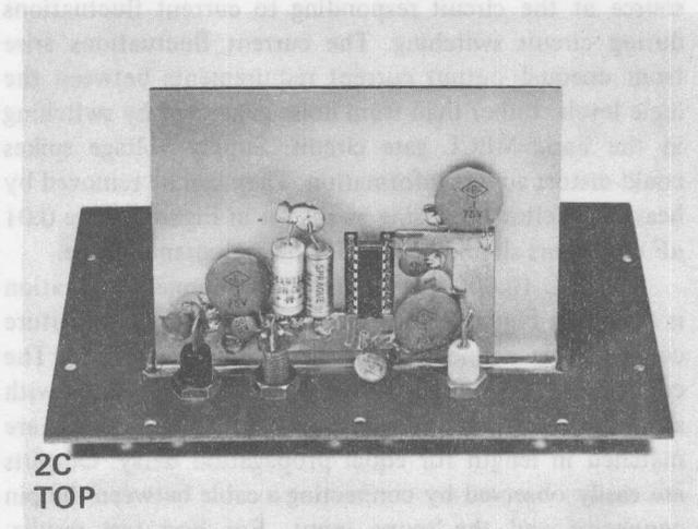
FIGURE 2 — Views of MECL 10,000 Test Fixture
