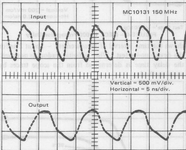
FIGURE 6 - MC10131 Toggle Rate Test
