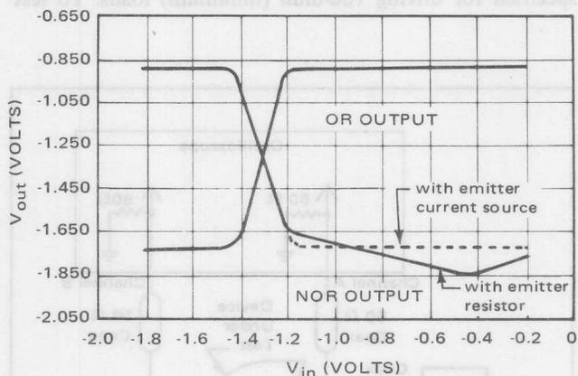
FIGURE 3 — Typical MECL 10,000 Transfer Characteristics
