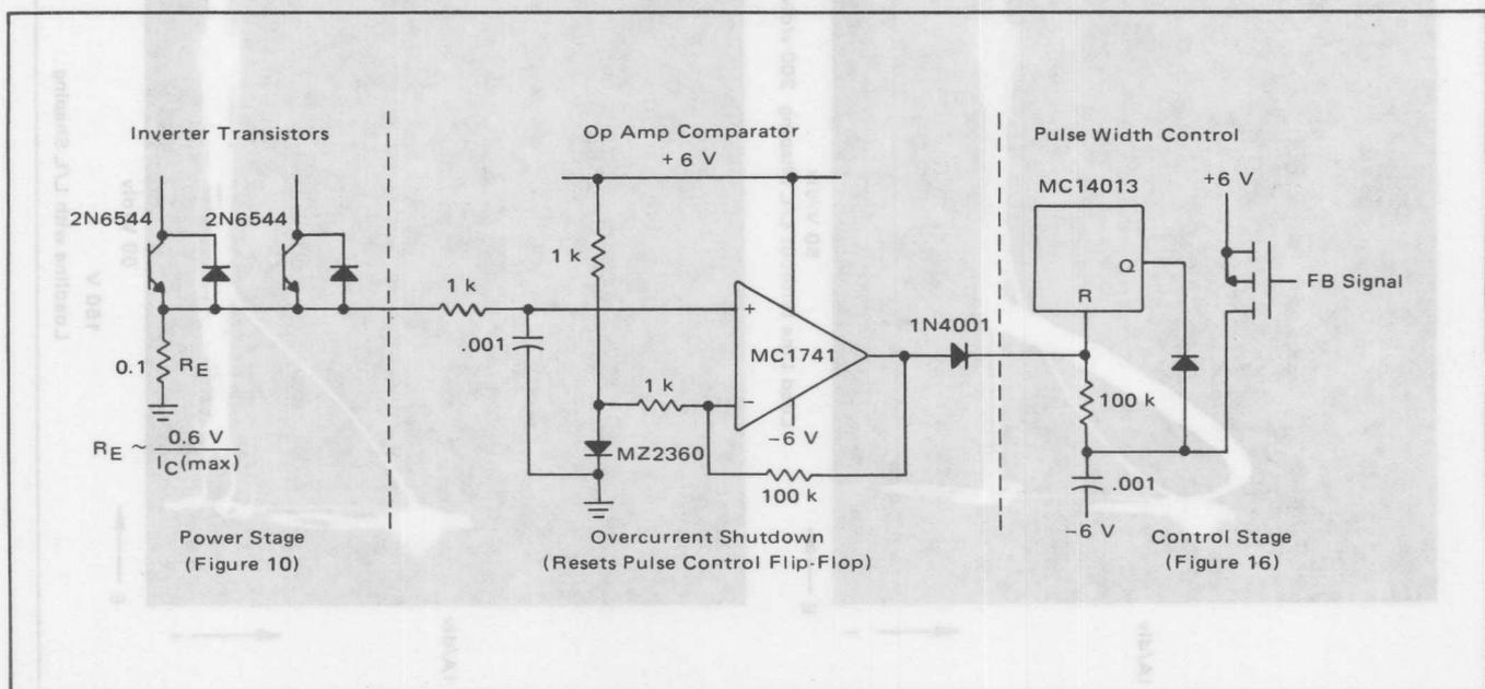
FIGURE 13 - Suggested Overcurrent Shutdown Circuit
